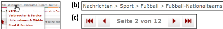
Figure 1: Examples of navigation design patterns. (a) Hierarchical pop-up menu, (b) breadcrumb trail, (c) pagination
