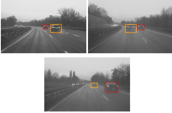
Figure 3.13.: Screenshots of one testing sequence with two vehicles performing an overtaking maneuver on an extra urban street (Firl and Tran, 2011). Maneuver recognition results are shown in Figure 3.14. Screenshots are captured approximately at frame 0, 270 and 560.
