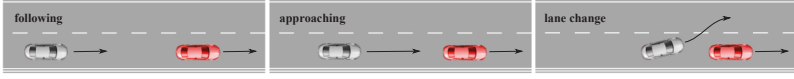
Figure 4.1.: Typical flow of a lane change maneuver on extra urban traffic roads. The three stages are: following (optional), approaching and lane change; see (Firl et al., 2012).
