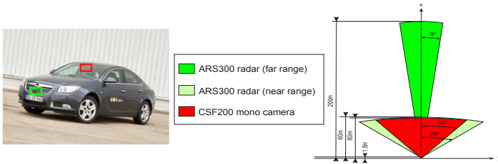
Figure 3.12.: Sensor setup of the used experimental vehicle: Sensor system consists of a mono camera and a radar sensor performing a far and a short range scan. Left: Opel Insignia experimental vehicle. Right: Opening angles of the used sensor setup (Firl and Tran, 2011).
