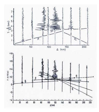
**Fig. 1-3:** Record section of the ESE profile of the blasts near Haslach in 1948 **Top:** Correlation of phases after Reich et al. (1948), **bottom:** Correlation by Landisman et al. (1966)
