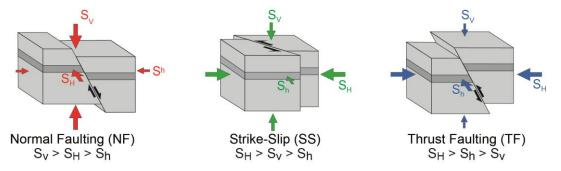
Fig. 2: Tectonic regimes and the role of the vertical stress which is the maximum principal stress in normal faulting regimes, the intermediate principal stress in a strike-slip regime and the least principal stress in a thrust faulting regime.
