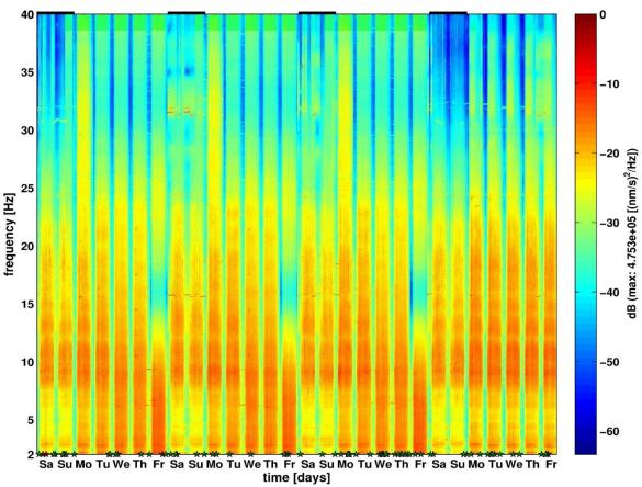
**Fig. 9.21:** Spectrogramme of a site in Bucharest, the capital of Romania, with the power spectral density in decibel for four weeks: there is a daily and a weekly rhythm of the background seismic noise. Thick bars at the top indicate weekends, stars at the bottom local and teleseismic events (courtesy of J. Groos).
