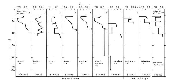
**Fig. 4-08:** Velocity-depth models of the subcrustal lithosphere in Western Europe for profiles recorded until 1973 (from Prodehl, 1984, Fig. 15; Prodehl and Mooney, 2012, Fig. 7.2.1-07). 73H5: Hirn et al., 1973, 74K1: Kind, 1974a, 75A2: Ansorge, 1975, 75H1: Hirn et al., 1975, 74S4: Steinmetz et al., 1974.
