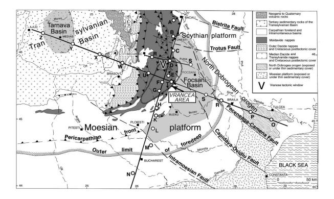
**Fig. 12-01:** Location map of seismic-refraction VRANCEA profiles 1999 (N-S line) and 2001 (W-E line) through the seismogenic Vrancea zone in the eastern Carpathians of Romania (from Hauser et al., 2002; Prodehl and Mooney, 2012, Fig. 9.2.4-11). V = Vrancea seismogenic zone with strong intermediate-depth earthquakes between 70 and 160 km depth.
