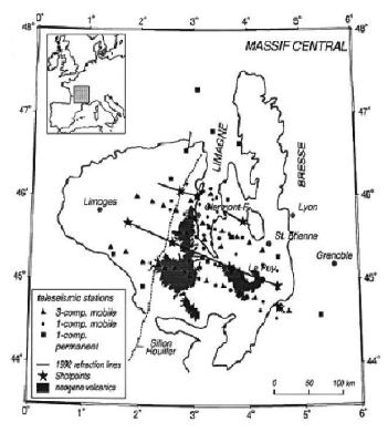
**Fig. 3-05:** Limagnegraben 1992: location of teleseismic stations and seismic refraction lines (stars = shotpoints) (from Prodehl et al., 1995, Fig. 4-4; Prodehl and Mooney, 2012, Fig. 9.2.2-09).
