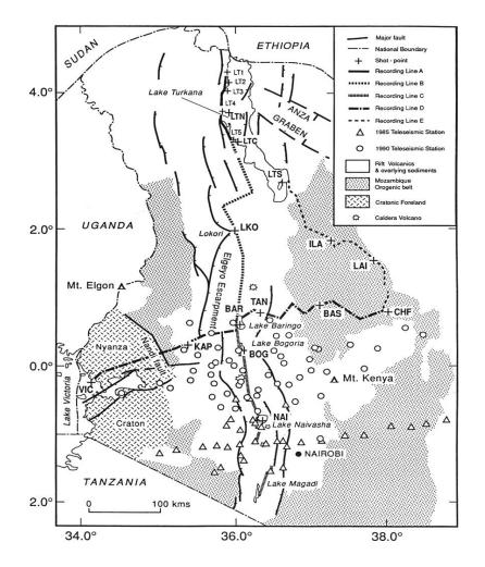
**Fig. 9-07:** KRISP 90 location map showing the seismic refraction / wide-angle reflection lines and the configuration of the teleseismic networks in 1985 and 1989-1990 (from Keller et al., 1994b, Fig. 1; Prodehl and Mooney, 2012, Fig. 9.5.1-01). The 1985 refraction lines extended from Lake Baringo to Lake Magadi and across the rift valley south of Lake Naivasha, parallel to the 1985 teleseismic cross line (white triangles).
