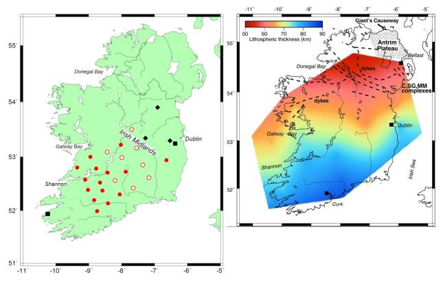
**Fig. 9.16:** Left: Map of Ireland with the station sites of the ISLE experiment, black squares and diamonds indicate permanent broadband and short-period stations, red and white circle indicate mobile broadband and short-period stations. Right: Map of the lithospheric thickness and Tertiary volcanic structures in the northern of Ireland (after Landes et al., 2007).
