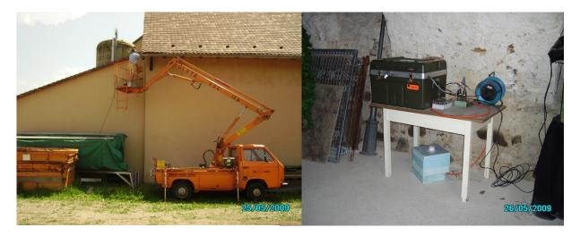
**Fig. 9.26:** Station SFN02, URS2 experiment in Staufen im Breisgau. Left: installation of a GPS antenna. Right: recording box and STS-2 seismometer (inside the blue box for thermal insulation) in a historic cellar.
