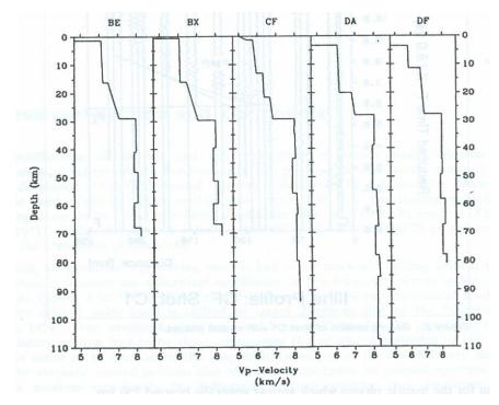
Fig. 4-24: 1-D velocity-depth models for the long-range profiles of ILIHA (from Arlitt et al., 1993, Fig. 8).
