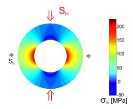
Fig. 3: Distribution of tangential stress magnitudes  $\sigma_{\theta\theta}$  around a vertical wellbore situated in a far field stress with the maximum horizontal stress  $S_H$  and the minimum horizontal stress  $S_h$ . The stress magnitudes concentrate in the orientation of  $S_h$ , where the stress magnitudes can overcome the rock strength and lead to the evolution of wellbore failure: borehole breakouts.
