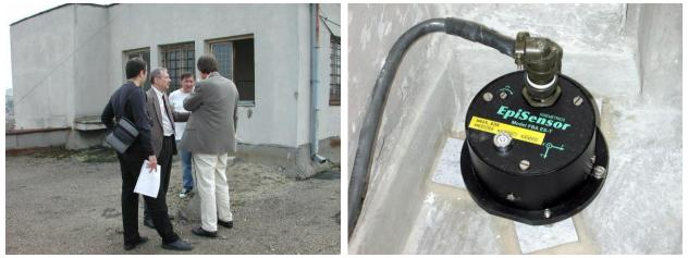
**Fig. 38:** Briefing at the top of the multy-story building: M. Bayraktarli (project C1/C2), Dan Lungu (owner of the flat, see Fig. 37), INCERC member, K.-P. Bonjer (left figure). The center Episensor is still without thermal protection. The ceramic isolators of the feet are visible (right figure).
