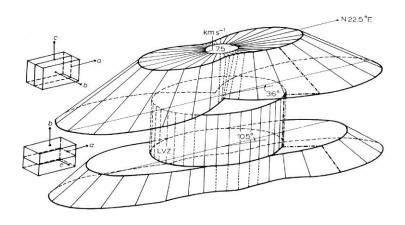
**Fig. 2-09:** Three-dimensional "anvil" model of Fuchs (1983) showing the continental anisotropic velocity-depth distribution in the uppermost mantle under southern Germany found by Bamford's (1973) time-term analysis (Fuchs, 1983, Fig.13; see also Prodehl and Mooney, 2012, Fig. 7.2.4-02).
