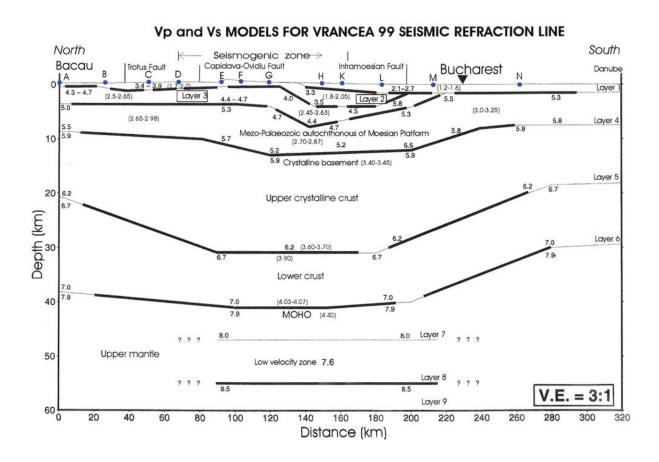
**Fig. 12-02:** Crustal P-wave cross section along the north-south profile VRANCEA 1999 (from Hauser et al., 2001, Fig. 9; Prodehl and Mooney, 2012, Fig. 9.2.4-13). Velocities in brackets are corresponding S-velocities.
