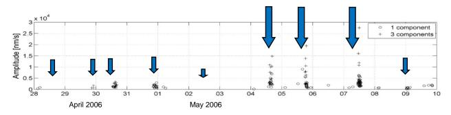
**Fig. 9.30:** Occurrence of seismic events ( $M_L < 1$ , see amplitude scale) in the TIMO dataset at stations near Landau. Arrows indicate fluid injection periods with length about proportional to injection rate (modified after Plenkers et al., 2013).
