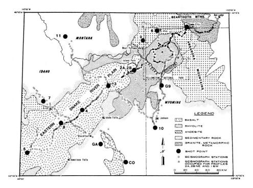
**Fig. 11-01:** 1978-80 seismic refraction observations in the Yellowstone – Snake River plain (from Braile et al., 1982, Fig. 1; Prodehl and Mooney, 2012, Fig. 7.4.1-03).
