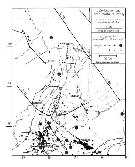
Fig. 3-04: Seismic-reflection lines and seismicity in the Rhinegraben (from Mayer et al., 1997; see also Prodehl and Mooney, 2012, Fig. 9.2.2-06).
