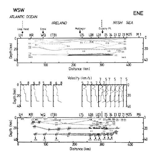
Fig. 6-06: Crustal cross section resulting from the ICSSP project of 1982 (from Jacob et al., 1985, Fig. 8; Prodehl and Mooney, 2012, Fig. 8.3.2-04). Upper part: Cross section with lines of equal velocity, middle part: 1-D velocity-depth functions, lower part: Position of zones where crustal reflected phases originate.
