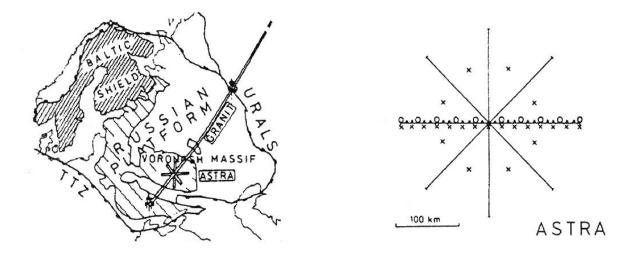
Fig. 4-28: Left: Location of the ASTRA sub-experiment (from (Lueschen, 1992; see also Prodehl and Mooney, 2012, Fig. 9.3-17). Right: Observation scheme. Crosses are borehole shots with 200-300 kg charges, 20 km apart. Circles are 48-channel digital recording instruments of type < Progress >, which were spaced 30 km apart. Dots are 3-component analogue recording devices, which were 10 km apart.
