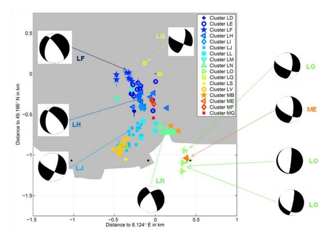
**Fig. 9.31:** Results of the seismic event analysis ( $M_L < 2.7$ ) below Landau (grey area corresponds to the town area of Landau). Colours indicate events with a very high waveform correlation which are merged in clusters. Fault plane solutions imply a normal to strike slip faulting regime. Figure courtesy of Laura Gassner, Jörn Groos, Michael Grund, Joachim Ritter and Jens Zeiß.
