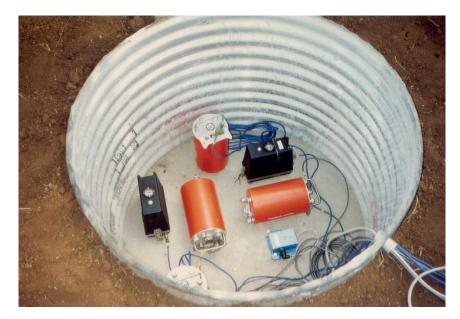
**Fig. 9.9:** Test installation in the Chyulu Hills. Different sensors and their recorders were run in parallel mode to compare response functions (red: Geotech S13, black: Kinemetrics SH-1, blue: Lennartz electronic 1 s)
