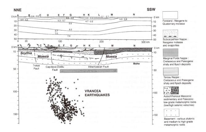
**Fig. 12-03:** Interpreted geological cross section along the main VRANCEA99 seismic refraction line between Bacau and Bucharest (from Hauser et al., 2001, Fig. 10). Circles represent the foci of the intermediate depth earthquakes of the Vrancea zone after Oncescu et al. (1999) projected into this cross section.
