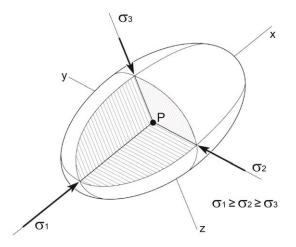
Fig. 1: Lamé stress ellipsoid. The three principal stresses (Eigenvectors)  $\sigma_1$ ,  $\sigma_2$  and  $\sigma_3$  of the symmetrical stress tensor  $\sigma_{ii}$  describe the state of stress at a point P.
