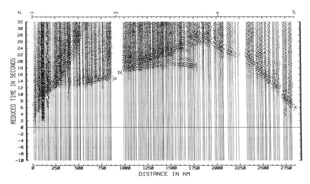
**Fig. 4-27:** Data example of the super long deep seismic sounding profile "Quartz" in the USSR observed in 1984 (thick line in **Fig. 4-26**) (from Mechie et al., 1993, Fig. 3b; see also Prodehl and Mooney, 2012, Fig. 8.4-03).
