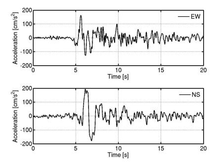
Horizontal acceleration records of the March 4, 1977 earthquake in Bucharest (INCERC). The long-period characteristic of the NS-component made engineers believe that the Vrancea events have much more lower frequencies as compared to standard Eurocode Spectra.
