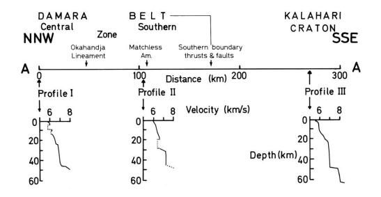
**Fig. 7-07:** Velocity-depth sections through the Damara orogen and adjacent Kalahari craton, approximately 380 km NNE of the Atlantic coast (from Baier et al., 1983, Fig. 4; Prodehl and Mooney, 2012, Fig. 7.7.2-03).
