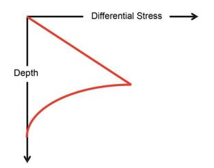
Fig. 10: Sketch of the vertical distribution of maximum differential stress in the crust. For the uppermost crust with low temperatures and low pressures, the differential stress is limited by frictional sliding. At greater depth ductile deformation is limiting the maximum sustainable differential stress.
