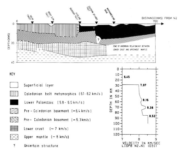
Fig. 4.12: Top: Crustal cross section of LISPB 1974 (from Bamford et al., 1978, Fig. 15). Bottom: Schematic cross section of subcrustal reflections (from Faber, 1978, Fig. 10.4; see also Prodehl and Mooney, 2012, Fig. 7.2.4-06).
