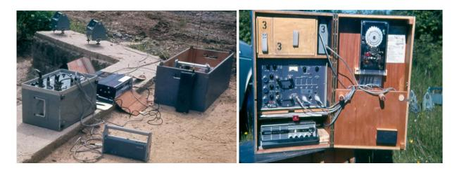
**Fig. 2-03:** Recording unit MARS 66. Left: modulator, center: tape recorder and T75A time receiver, right: seismometer box.
