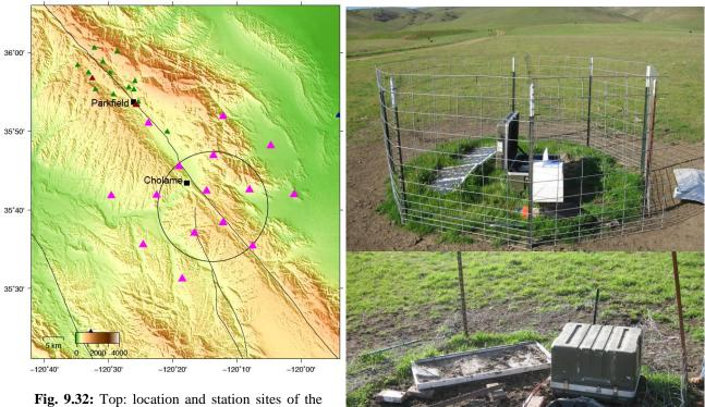
PERMIT experiment near Cholame, California. Purple triangles are KABBA stations, green triangles are permanent stations. Black lines indicate faults related to the San Andreas Fault system. Right: Recording station before and after an attack by cows. Note the upside down recorder box and the trampled seismometer vault (courtesy W. Scherer & E. Cochran).
