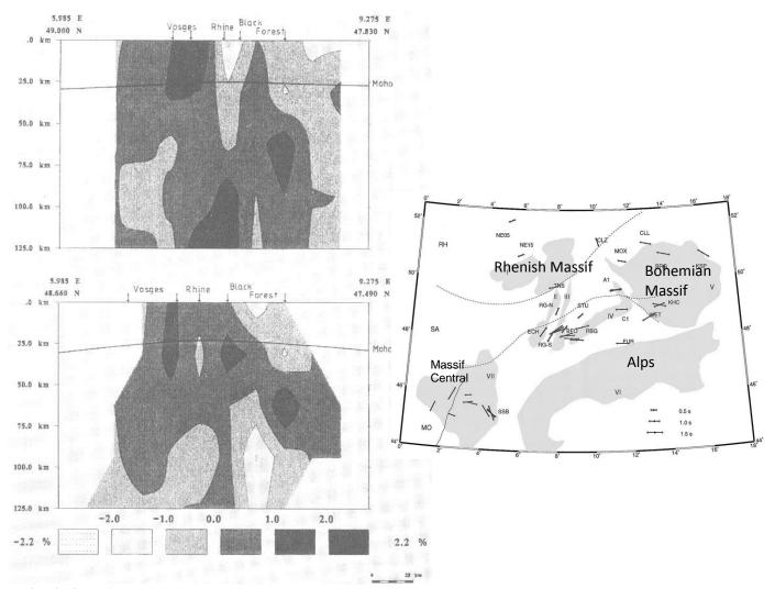
**Fig. 9.12:** Left: vertical cross sections through the 3-D model with perturbations of the P-wave velocity underneath the southern Upper Rhine Graben (for position of the sections see map in Fig. 9.11 from SFB Berichtsband 1991). Right: collection of fast polarisation directions of SKS splitting measurements in several regions of Central Europe. Mountain areas are indicated in grey, modified after Granet et al. (1998).
