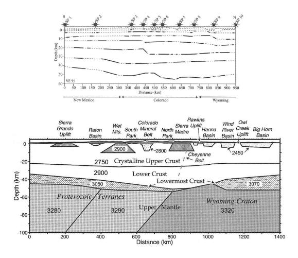
Fig. 11-11: Interpretation of the CD-ROM seismic-refraction data (from Snelson et al., 2005, Fig. 11c and Fig.12d; Prodehl and Mooney, 2012, Fig. 9.4.2-29). Top: Model based on first arrivals and wide-angle reflections (from Snelson et al., 2005, Fig. 11c). Bottom: 2.5-D density model along the CD-ROM transect. The distance scale corresponds to that of the seismic model (from Snelson et al., 2005, Fig.12d).
