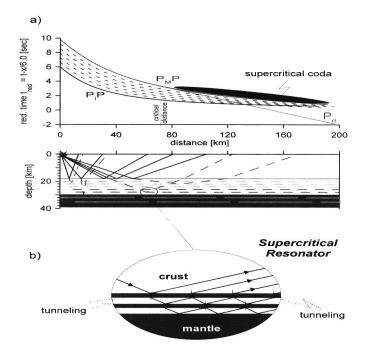
Fig. 4-25: Scattering of energy between PiP and  $P_MP$  phases, caused by internal structure of the lower crust from 18-30 km model-depth, is followed by supercritical reverberations following  $P_MP$  (supercritical coda), caused by internal structure of the topmost mantle below 30 km model-depth, which has a different scale of structural dimensions (from Enderle et al., 1997, Fig. 4a; Prodehl and Mooney, 2012, Fig. 9.2.2-12).
