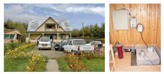
**Fig. 41:** The Early Warning Site Plostina in the center of the southeastern bend of the Carpathian Mountains: the main building and the instrument hut with borehole, K2-datalogger, Episensor, and Mark Products sensor.
