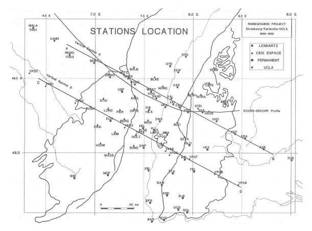
**Fig. 9.11:** Network with temporary and permanent stations in the southern Upper Rhine Graben region in 1988/89 (SFB-Berichtsband, 1991).
