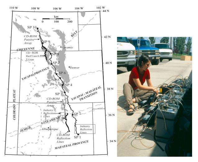
**Fig. 11-07:** Seismic profiles in the Southern Rocky Mountains (from Rumpel et al., 2005, Fig.1; Prodehl and Mooney, 2012, Fig. 9.4.2-27). **Fig. 9.4.2-27**.
