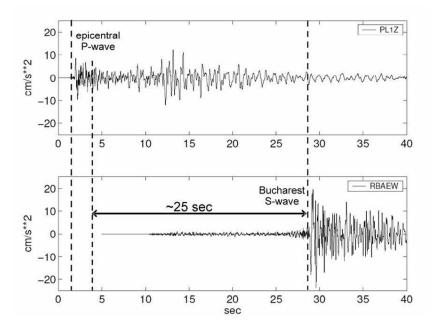
The maximum warning time for Bucharest is defined by the time span between the arrival of the direct P-wave at the detecting EEW sensor in the epicentral area and the S-wave arrival in Bucharest. The expected warning time for Vrancea earthquakes is about 25 s (Maren Böse).
