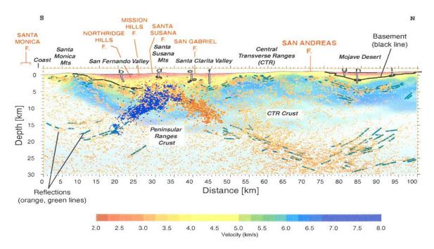
**Fig. 11-19:** Tomographic velocity model and superimposed line drawings of CMP data along LARSE line 2 (from Ryberg et al., 2004, Fig. 11; Prodehl and Mooney, 2012, Fig. 9.4.2-22). Internal report, based on Fuis et al. (2001, 2003).
