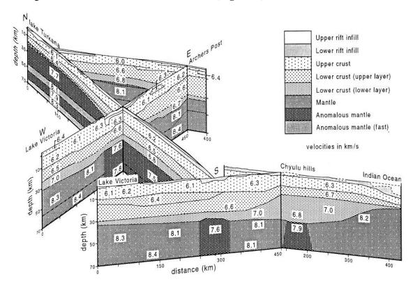
**Fig. 9-25:** KRISP 90/94 fence diagram showing crustal and upper mantle structure of the Kenya rift from Lake Turkana to Lake Magadi and beneath the neighbouring flanks from Lake Victoria to the Indian Ocean (from Khan et al., 1999, Fig. 4; Prodehl and Mooney, 2012, Fig. 9.5.1-08).
