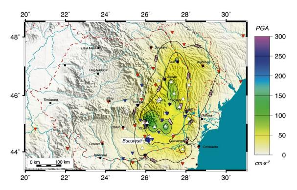
**Fig. 45:** PGA-Shakemap of the October 27, 2004 event: Observed peak ground accelerations (white and blue triangles), and computed PGA's (red triangles) (Bonjer et al., 2008; Bonjer, 2012) on the basis of the observed intensities from the Community Internet Intensity Map (Wald et al., 1999).
