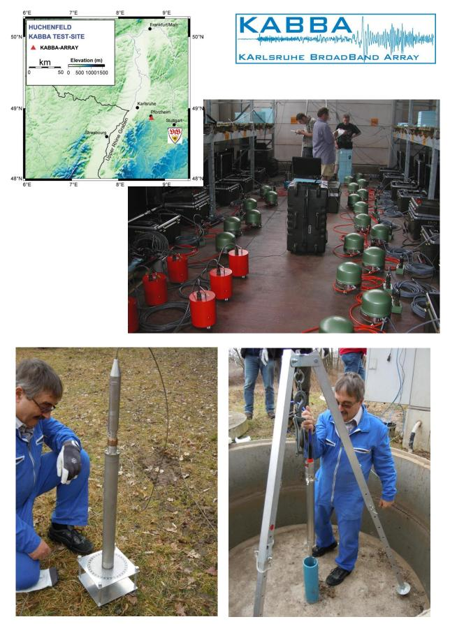
**Fig. 9.19:** Top: first test measurements with the KArlsruhe BroadBand Array near Huchenfeld, Pforzheim (from left: T. Diehl, J. Ritter & J. Mathar). Different sensor types can be seen (red: Geotech KS-2000, green: Streckeisen STS-2, blue: Lennartz 5 s, silver: Güralp 40T). Bottom: Orientation and installation of a Lennartz borehole seismometer near Landau (Fig. 9.29) with W. Walker.
