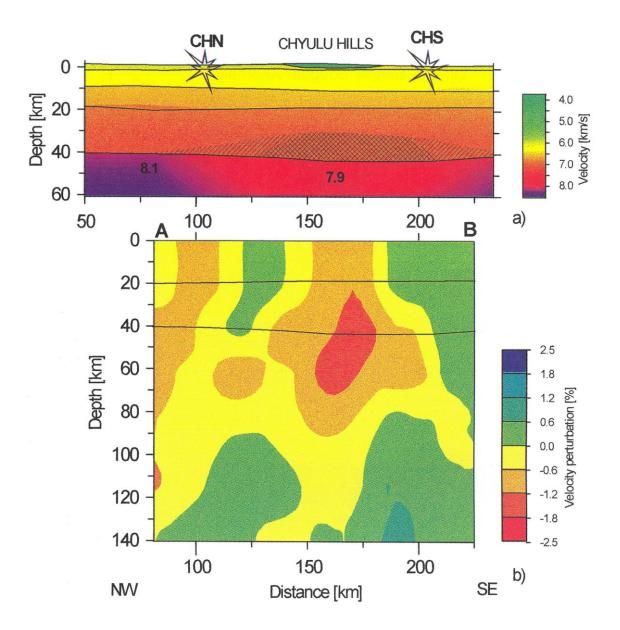
Fig. 9-26: Crust and upper mantle structure underneath the Chyulu Hills volcanic field (from Novak et al., 1997b, Fig. 7; Prodehl and Mooney, 2012, Fig. 9.5.1-09). a) Part of the crustal model along line F of Novak et al. (1997a), b) cross section through the teleseismic tomography model of Ritter and Kaspar (1997).
