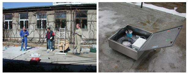
**Fig. 40:** The 100 m borehole at INCERC site: the Karlsruhe installation: The team (left figure): Werner Scherer (GPI), George Chircea (NIEP), and Manfred Rittershofer (GPI). (Right figure): the waterproofed box protecting the borehole mouth, and the power supply.
