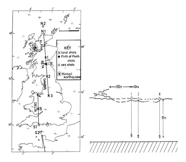
Fig. 4-09: LISPB 1974 location map (from Bamford et al.,<br/>1976, Fig. 1; Prodehl and Mooney, 2012, Fig. 7.2.4-05).Fig. 4-10: Scheme of sea shots with split charges<br/>(from Bamford et al., 1976; Fig. 4)
