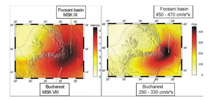
Probabilistic hazard maps for Romania in macro-seismic intensities (left) and peak ground acceleration (right) show the dominant effect of the Vrancea seismicity for the overall hazard, specifically for Bucharest (Vladimir Sokolov).
