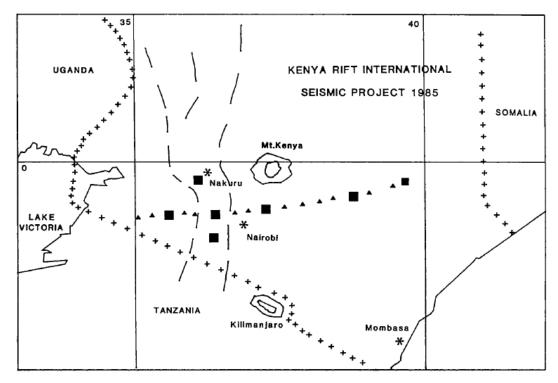
**Fig. 9.4:** Station map of the KRISP'85 experiment. The dashed lines indicate the position of the Kenya Rift, a major zone of continental breakup. Triangles show 1 s one-component stations, squares show 5 s three-component stations (Achauer, dissertation, 1990).
