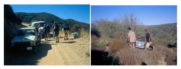
Fig. 11-14 and Fig. 11-15: GFZ-6-channel stations with 6 vertical seismometers being connected to the central station by long cables are being deployed in difficult terrain in the Susanna Mountains north of Los Angeles.
