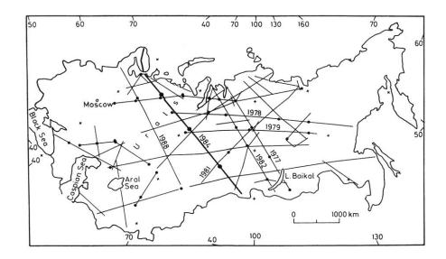
**Fig. 4-26:** Location map of long-range deep seismic sounding profiles in the USSR using PNE (dots - peaceful nuclear explosions) as energy sources for distance ranges of several 1000 km (from Mechie et al., 1993, Fig. 1; see also Prodehl and Mooney, 2012, Fig. 8.4-02).
