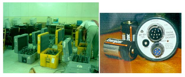
**Fig. 12-08:** Equipment: 15 "Texans" in a box for transportation. **Fig. 12-09:** "Texan" – RefTek-1-component station.
