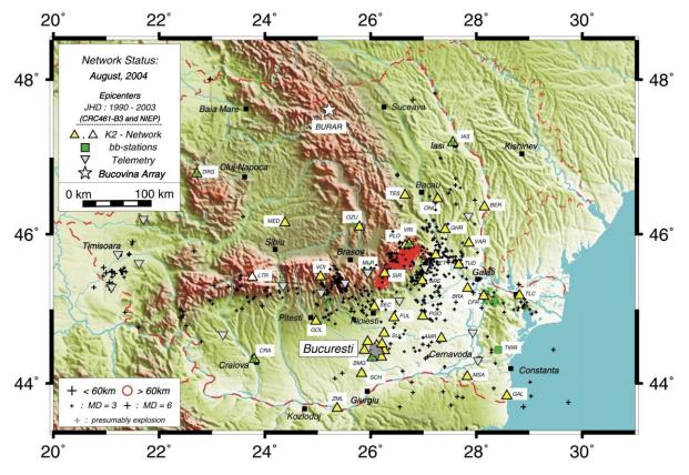
Fig. 34: Position map of the CRC 461- and NIEP K2-accelerometer stations (status of August 2004).
