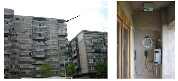
**Fig. 37:** Instrumentation of a standard 11-story building at the Bv. Stefan cel Mare in Bucharest. The arrow indicates the position of the installation (left figure). Installation of the Episensor under the roof (upside down) and the K2 (right figure).
