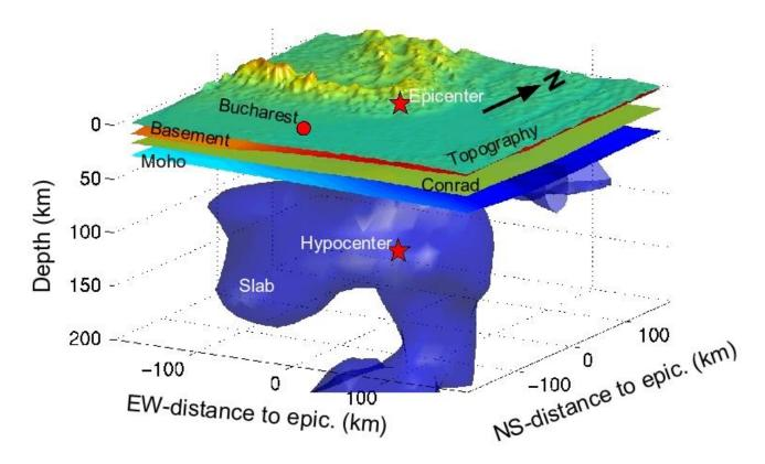
The 3D elastic model that emerged from geology, refraction seismics, and upper mantle tomography. It was used for modeling earthquake wave propagation, tectonic interpretations and state of stress calculations.
