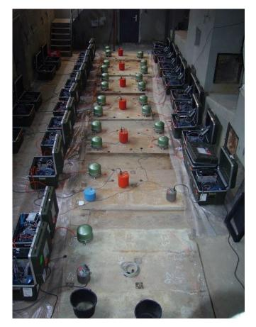
Fig. 13-1: Calibration test with the KABBA instruments in the basement of KIT-GPI. The mobile recording units measured coincidently for two months in order to detect possible instrument malfunctions and to compare the instrument response functions.
