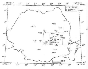
**Fig. 9.2:** Left: Seismic station network in Romania for the tomography of Koch (1985a). Right: 3-D model with the P-wave velocity (in km/s) down to 120 km depth. The area of relatively high velocity (solid line) corresponds to the Vrancea subduction zone (after Koch, dissertation, 1983).
