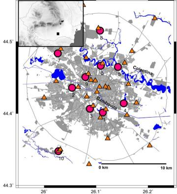
**Fig. 9.20:** Experimental layout for Bucharest urban projects: orange triangles indicate sites of the URS network (2003/04), red circles are locations of boreholes drilled within a NATO-funded project.
