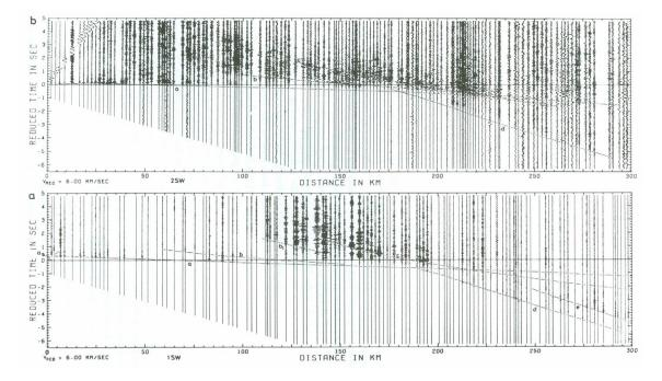
Fig. 8-13: Band-pass filtered record sections with correlated phases for (a) shotpoint 1 SW (true amplitudes) and (b) shotpoint 2-SW (normalized amplitudes). Reduction velocity = 6 km/s (from Mechie et al., 1986, Fig. 3).
