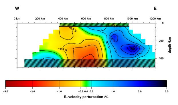
**Fig. 9.28:** East-west cross section through the 3-D tomography model with shear wave velocity (*vs*) perturbations (for approximate position see Fig. 9.27). There is a clear steeply eastward dipping transition with low *vs* in the west (Phanerozoic lithosphere) and higher *vs* in the east (Baltic Shield lithosphere). This velocity contrast continues subvertically into the upper mantle (after Wawerzinek, 2012).
