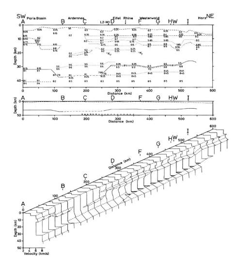
Fig. 4-16: Crustal cross section and velocity-depth functions along the main line of the Rhenish Massif project (from Mechie et al., 1983, Fig. 4; Prodehl and Mooney, 2012, Fig. 7.2.6-04).
