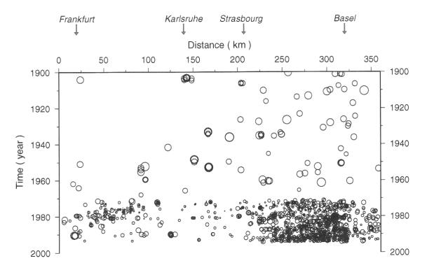
**Fig. 7:** The seismic activity in the Upper Rhinegraben between Frankfurt and Basel for the years 1900-1979. The rather abrupt increase of the seismic activity around 1971/72 is the result of the implementation of the high-gain networks of the GPI, the French networks in the Vosges Mountains and the Swiss networks in the southern end of the Rhinegraben.
