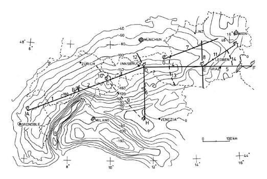
Fig. 4-13: Simplified gravity map of the Alps and the location of ALP75 (from Alpine Explosion Seismology Group, 1976, Fig. 2; see also Prodehl and Mooney, 2012, Fig. 7.2.4-08).
