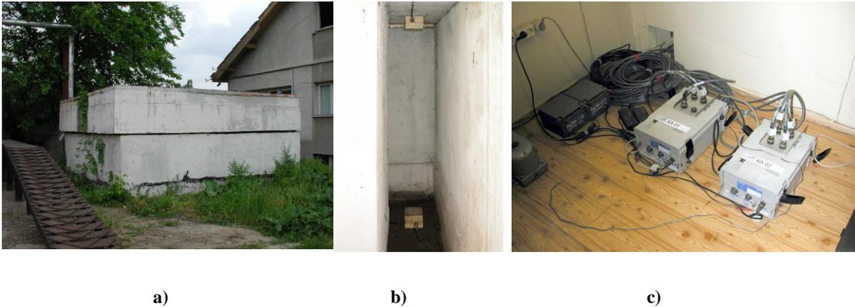
**Fig. 36:** The test-building at the INCERC-site (a). The roof is decoupled by Elastomer-buffers from the basement. The six three-component KMI FBA-23 accelerometers are at the basement and (upside down) under the roof (b). The two 12-channel K2-datalogger (c) record the 3 basement, and the 3 roof accelerometers as well as the three-component nearly free-field Episensor and the Mark Products velocity-sensor installed in the cellar of the neighboring building (see (a)).
