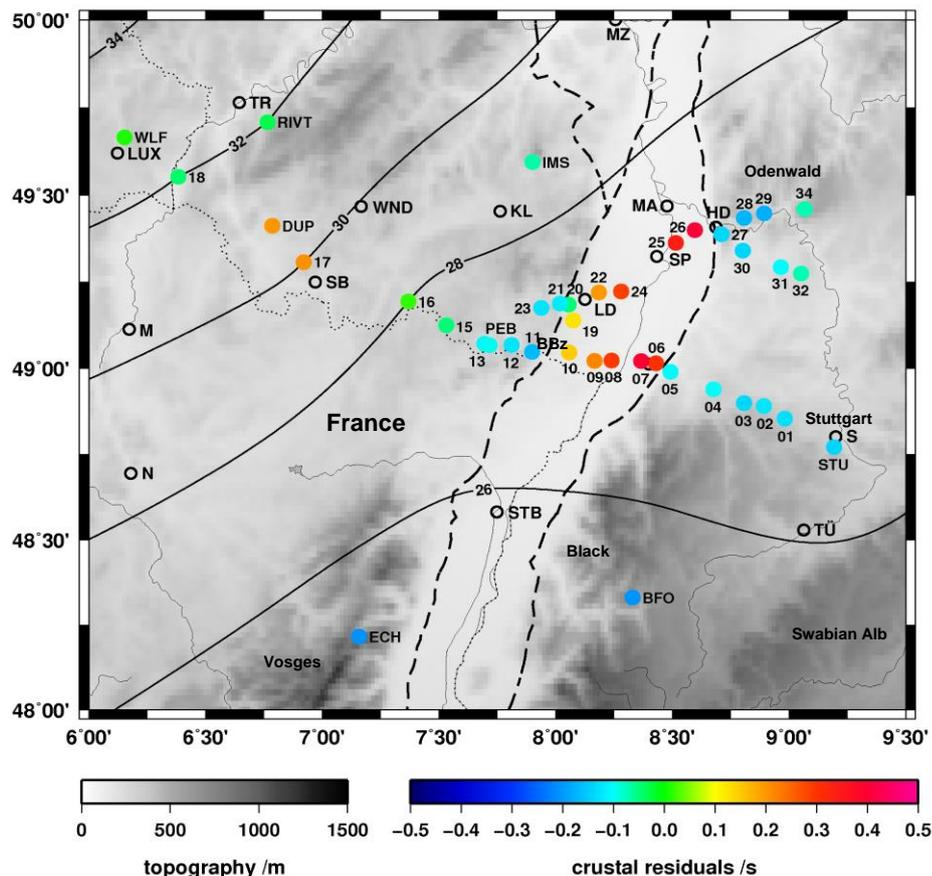
**Fig.9.22:** Station map of the TIMO experiment (2004-2006). The colours indicate average travel time residuals for P-waves due to variations in crustal structure and thickness. Contour lines show known crustal thickness.
