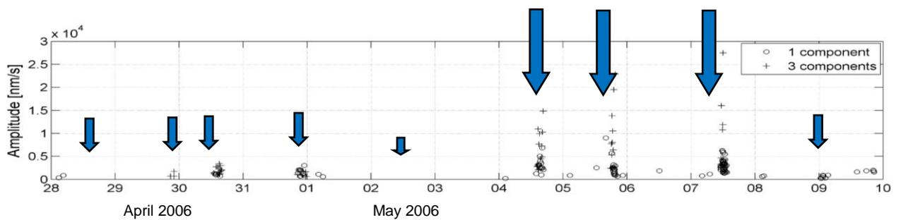
**Fig. 9.30:** Occurrence of seismic events ( $M_L < 1$ , see amplitude scale) in the TIMO dataset at stations near Landau. Arrows indicate fluid injection periods with length about proportional to injection rate (modified after Plenkers et al., 2013).
