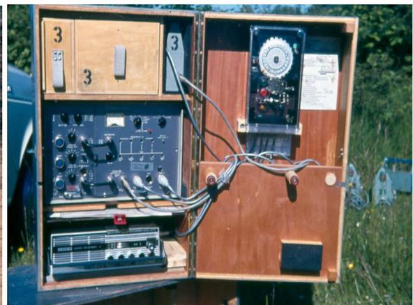
**Fig. 2-04:** Recording unit MARS 66 equipped with a mechanical clock (upper right). Upper left: T75A time-signal receiver, middle left: modulator, lower left: tape recorder. FS-60 seismometers in the background to the right.
