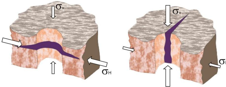
Fig. 5: Hydraulic fractures initiating at a wellbore. These develop when fluid-pressure in the wellbore creates tensile stresses at the borehole wall which exceed the tensile strength of rock mass. At greater distance to the wellbore the pressure necessary to keep fractures open corresponds to the least principal stress. The fractures open according to the principle of least resistance and close when the pressure reduces.
