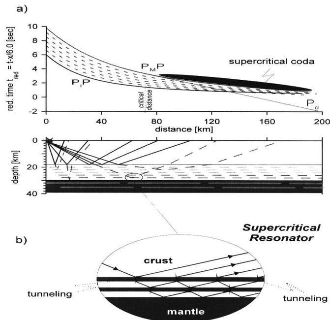
**Fig. 4-25:** Scattering of energy between  $P_iP$  and  $P_M P$  phases, caused by internal structure of the lower crust from 18-30 km model-depth, is followed by supercritical reverberations following  $P_M P$  (supercritical coda), caused by internal structure of the topmost mantle below 30 km model-depth, which has a different scale of structural dimensions (from Enderle et al., 1997, Fig. 4a; Prodehl and Mooney, 2012, Fig. 9.2.2-12).
