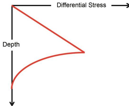
Fig. 10: Sketch of the vertical distribution of maximum differential stress in the crust. For the uppermost crust with low temperatures and low pressures, the differential stress is limited by frictional sliding. At greater depth ductile deformation is limiting the maximum sustainable differential stress.
