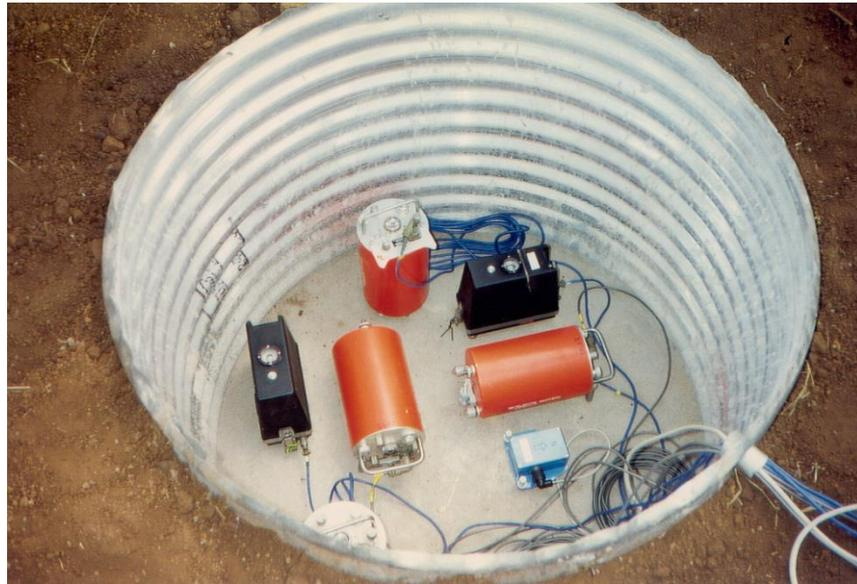
**Fig. 9.9:** Test installation in the Chyulu Hills. Different sensors and their recorders were run in parallel mode to compare response functions (red: Geotech S13, black: Kinometrics SH-1, blue: Lennartz electronic 1 s)
