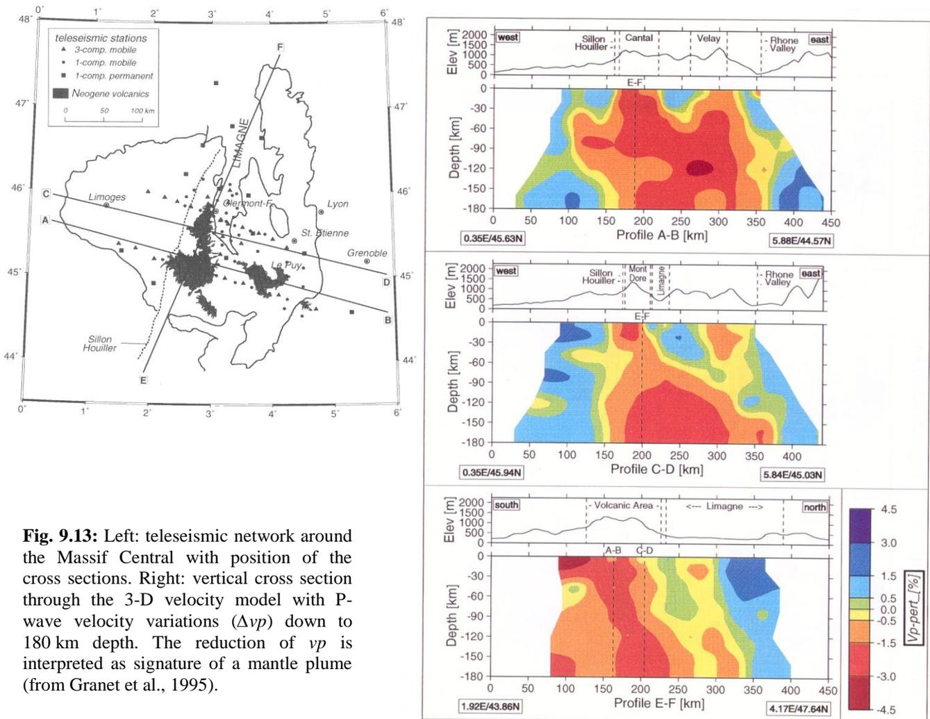
**Fig. 9.13:** Left: teleseismic network around the Massif Central with position of the cross sections. Right: vertical cross section through the 3-D velocity model with P-wave velocity variations ( $\Delta v_p$ ) down to 180 km depth. The reduction of  $v_p$  is interpreted as signature of a mantle plume (from Granet et al., 1995).
