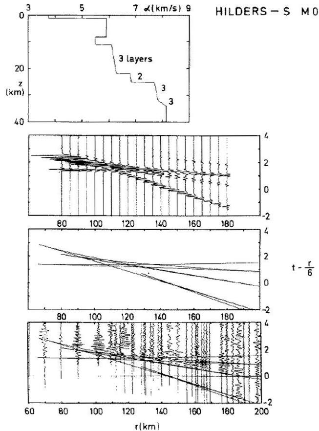
**Fig. 2-1:** Velocity-depth function, synthetic seismograms (vertical displacement), traveltime curves and traveltime curves overlain on the observed seismograms shown for the example of the profile from Hilders-S. Only reflections from the bottom of the layers are included (from Müller and Fuchs, 1976, Fig. 3; see also Prodehl and Mooney, 2012, Fig. 6.2.5-04).
