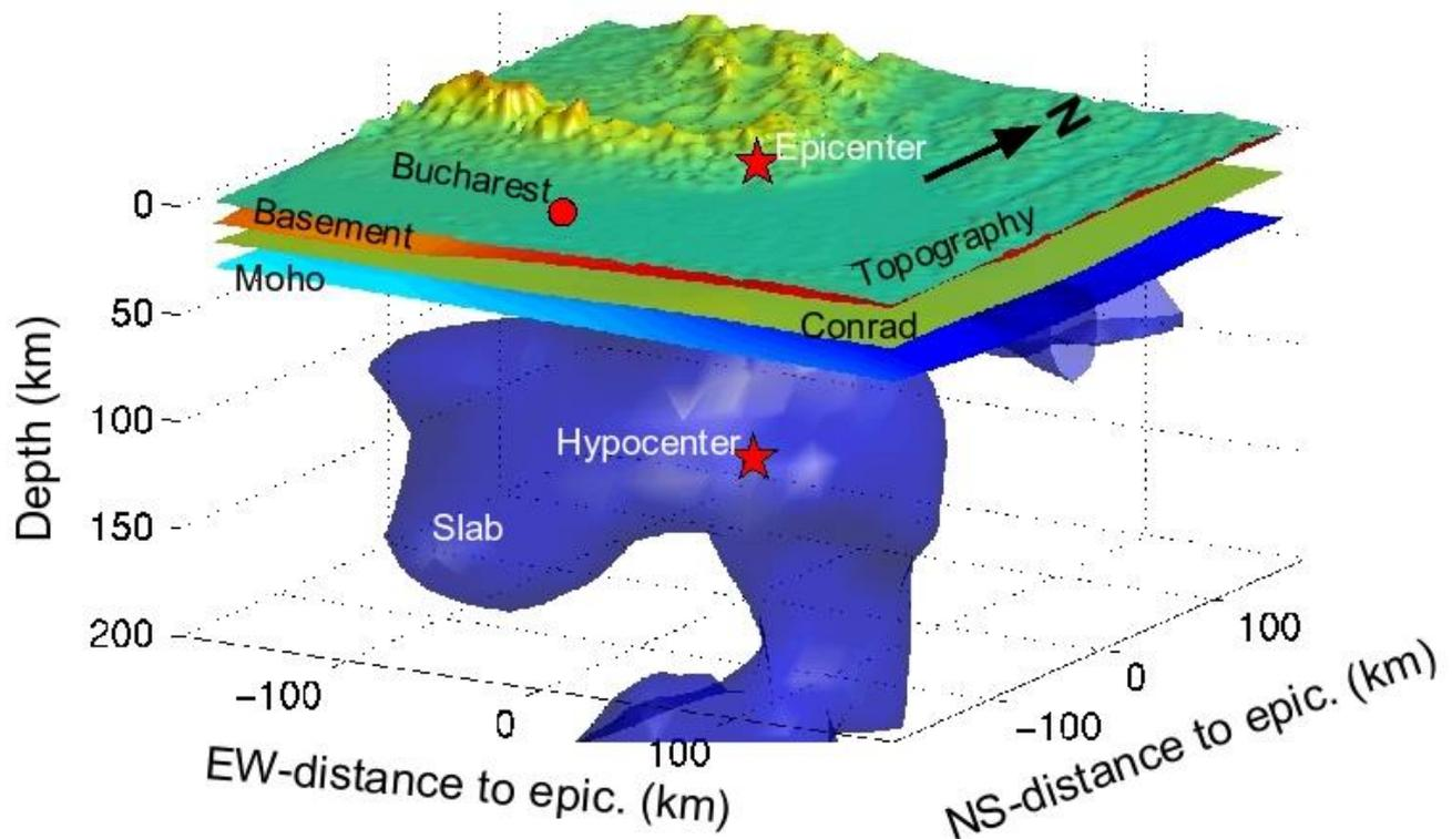
The 3D elastic model that emerged from geology, refraction seismics, and upper mantle tomography. It was used for modeling earthquake wave propagation, tectonic interpretations and state of stress calculations.
