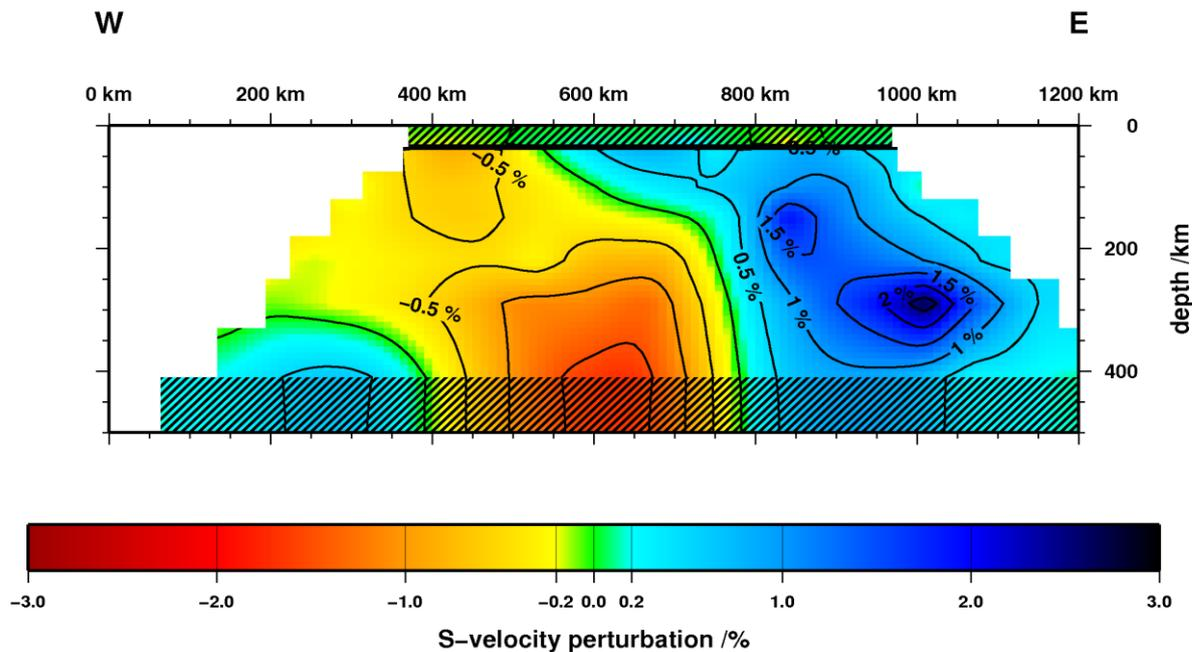
**Fig. 9.28:** East-west cross section through the 3-D tomography model with shear wave velocity ( $v_s$ ) perturbations (for approximate position see Fig. 9.27). There is a clear steeply eastward dipping transition with low  $v_s$  in the west (Phanerozoic lithosphere) and higher  $v_s$  in the east (Baltic Shield lithosphere). This velocity contrast continues subvertically into the upper mantle (after Wawerzinek, 2012).
