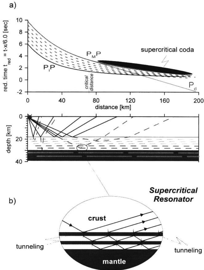
**Fig. 3-2:** Scattering of energy between  $P_iP$  and  $PMP$  phases, caused by internal structure of the lower crust from 18-30 km model-depth, is followed by supercritical reverberations following  $PMP$  (supercritical coda), caused by internal structure of the topmost mantle below 30 km model-depth, which has a different scale of structural dimensions (from Enderle et al., 1997, Fig. 4a; see also Prodehl and Mooney, 2012, Fig. 9.2.2-12).
