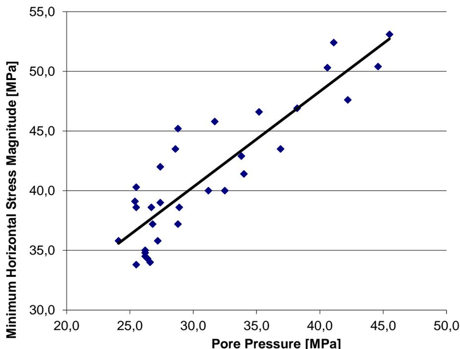
Fig. 12: Change of horizontal stress with change in pore pressure in the Ekofisk field. Data are from Teufel (1996). Due to the production the pore pressure has reduced from 48 MPa in 1969 to less than 25 MPa. The coupling of changes in horizontal stress to changes in pore pressure is around 70-80%.
