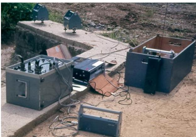
**Fig. 2-03:** Recording unit MARS 66. Left: modulator, center: tape recorder and T75A time receiver, right: seismometer box.
