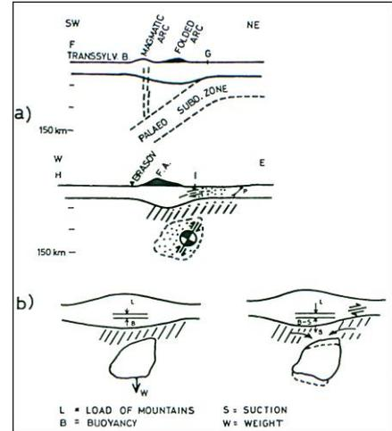
**Fig. 20:** Karl Fuchs ‘Suction Model’ of the Vrancea earthquake scenario.
