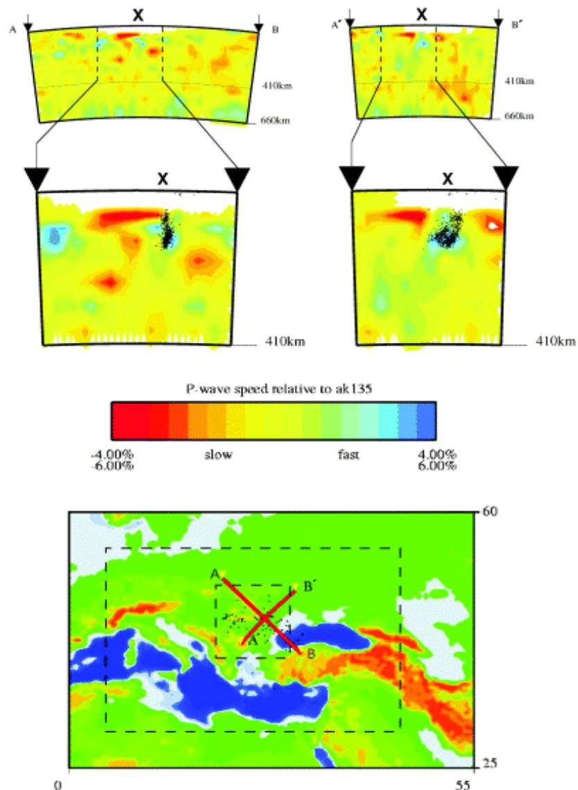
**Fig. 9.15:** Models with P-wave velocity perturbations ( $\Delta v_p$ ) south-eastern Europe. The top panels show  $\Delta v_p$  down to 660 km depth at regional scale (A-B and A'-B'), the panels in the middle are enlargements down to 410 km in the Vrancea region. X is the crossing point of the profiles (Weidle, dissertation, 2005).
