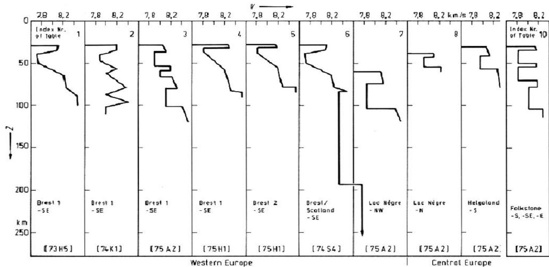
**Fig. 4-08:** Velocity-depth models of the subcrustal lithosphere in Western Europe for profiles recorded until 1973 (from Prodehl, 1984, Fig. 15; Prodehl and Mooney, 2012, Fig. 7.2.1-07). 73H5: Hirn et al., 1973, 74K1: Kind, 1974a, 75A2: Ansorge, 1975, 75H1: Hirn et al., 1975, 74S4: Steinmetz et al., 1974.
