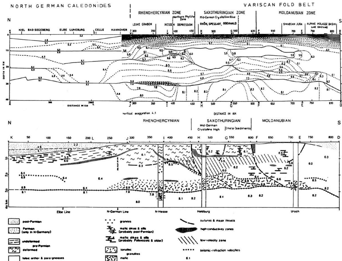
**Fig. 3-03:** Crustal cross section of the EGT central segment from the Baltic Sea to Lake Constance (from Prodehl and Aichroth, 1992, Fig. 3; Prodehl and Mooney, 2012, Fig. 8.3.4-09). Depth versus distance is exaggerated by 4:1. **Upper part:** Seismic velocity model. **Lower part:** Petrological interpretation.
