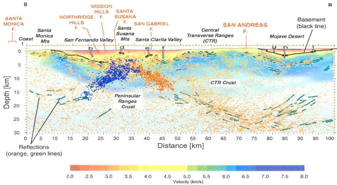
**Fig. 11-19:** Tomographic velocity model and superimposed line drawings of CMP data along LARSE line 2 (from Ryberg et al., 2004, Fig. 11; Prodehl and Mooney, 2012, Fig. 9.4.2-22). Internal report, based on Fuis et al. (2001, 2003).
