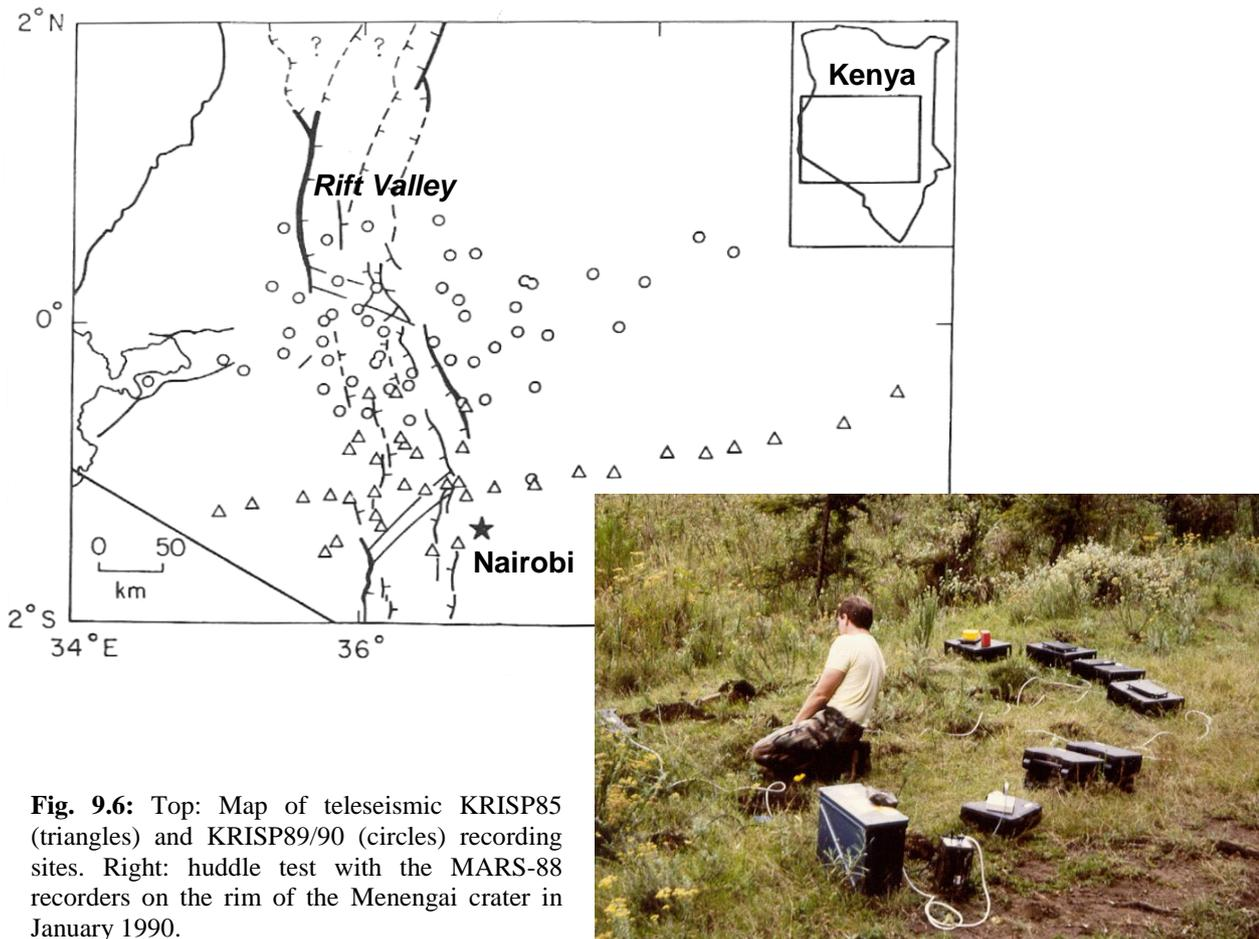
**Fig. 9.6:** Top: Map of teleseismic KRISP85 (triangles) and KRISP89/90 (circles) recording sites. Right: huddle test with the MARS-88 recorders on the rim of the Menengai crater in January 1990.
