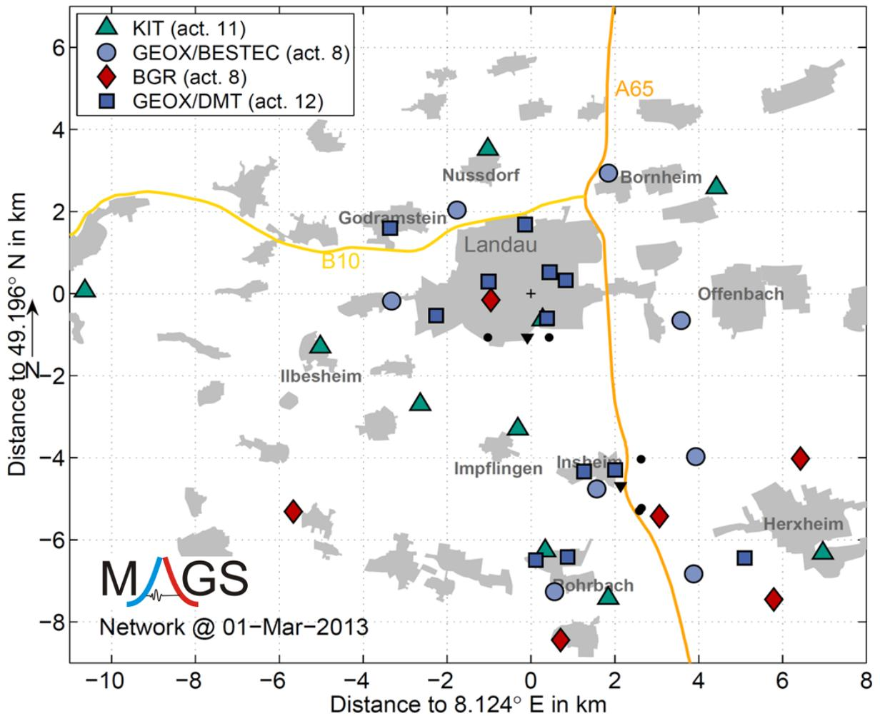
**Fig. 9.29:** Map displaying the TIMO2 / MAGS station sites from different operators around Landau and Insheim. Black inverted triangles represent geothermal power plants, black dots are the landing points of the drill holes at about 2.5-3.5 km depth.
