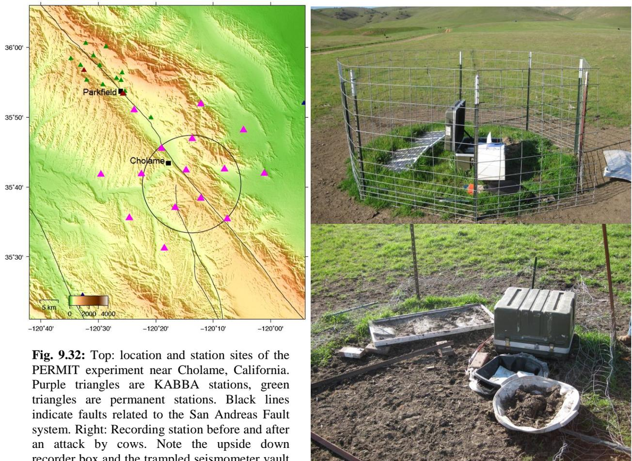
**Fig. 9.32:** Top: location and station sites of the PERMIT experiment near Cholame, California. Purple triangles are KABBA stations, green triangles are permanent stations. Black lines indicate faults related to the San Andreas Fault system. Right: Recording station before and after an attack by cows. Note the upside down recorder box and the trampled seismometer vault (courtesy W. Scherer & E. Cochran).
