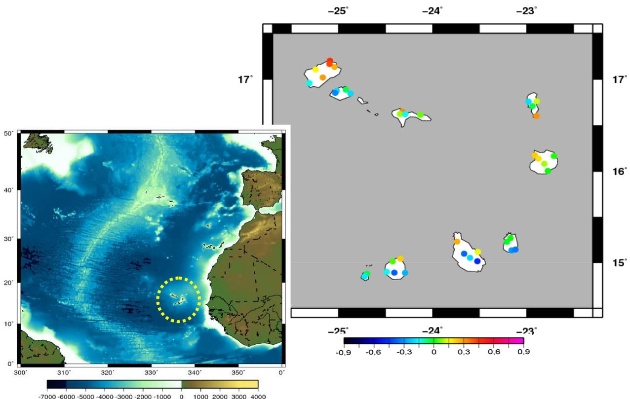
**Fig. 9.18:** Left: map of the Central Atlantic with the Cape Verde Islands (yellow circle). Right: station deployment of the COBO experiment 2007/08. The colour code displays travel time residuals in seconds for the earthquake source region South Sandwich Islands (wave incidence from south) (courtesy of J. Eisenbeis).
