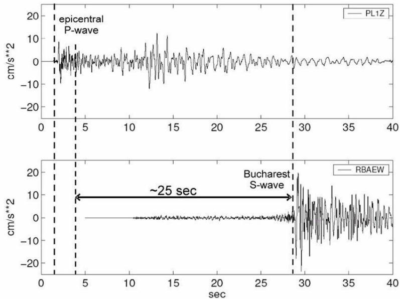
The maximum warning time for Bucharest is defined by the time span between the arrival of the direct P-wave at the detecting EEW sensor in the epicentral area and the S-wave arrival in Bucharest. The expected warning time for Vrancea earthquakes is about 25 s (Maren Böse).
