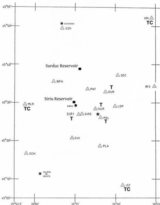
**Fig. 21:** Position map of the Surduc survey (Jung, 1983). The star shows the headquarter of the campaign: the school in Paltinis. The PCM-5000 locations BIC, CAR, and ARS are shown in Fig. 11.
