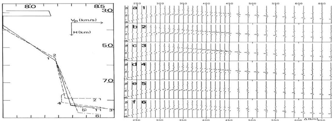
**Fig. 4-07:** **Left:** Velocity-depth models, corresponding to the long-range profiles in western France, show small possible variations in velocity resp. depth for slightly varying recording positions (from Hirn et al., Fig. 7). **Right:** Synthetic record sections in the  $P_1$ ,  $P_{II}$  distance range computed by the reflectivity method for the models to the left (from Hirn et al., 1975, Fig. 8; see also Prodehl and Mooney, 2012, Fig. 7.2.1-06).
