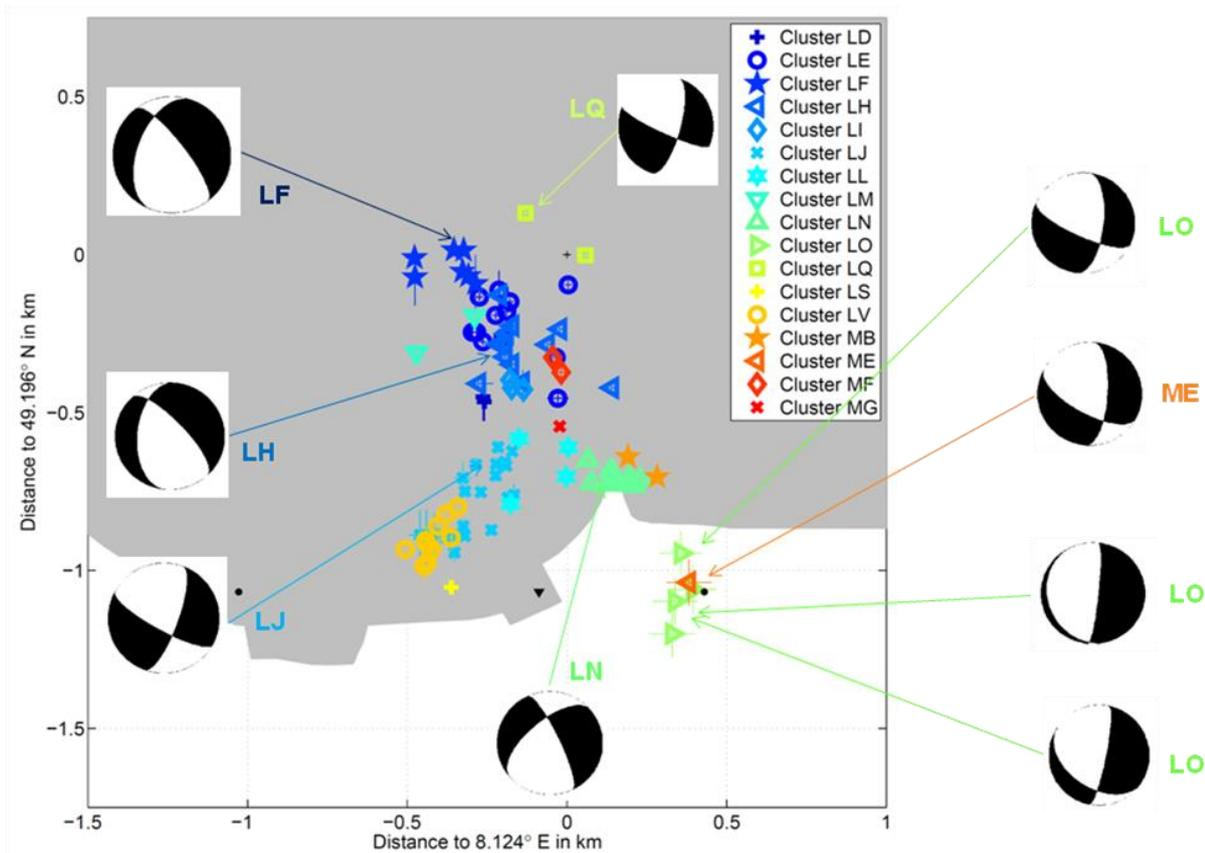
**Fig. 9.31:** Results of the seismic event analysis ( $M_L < 2.7$ ) below Landau (grey area corresponds to the town area of Landau). Colours indicate events with a very high waveform correlation which are merged in clusters. Fault plane solutions imply a normal to strike slip faulting regime. Figure courtesy of Laura Gassner, Jörn Groos, Michael Grund, Joachim Ritter and Jens Zeiß.
