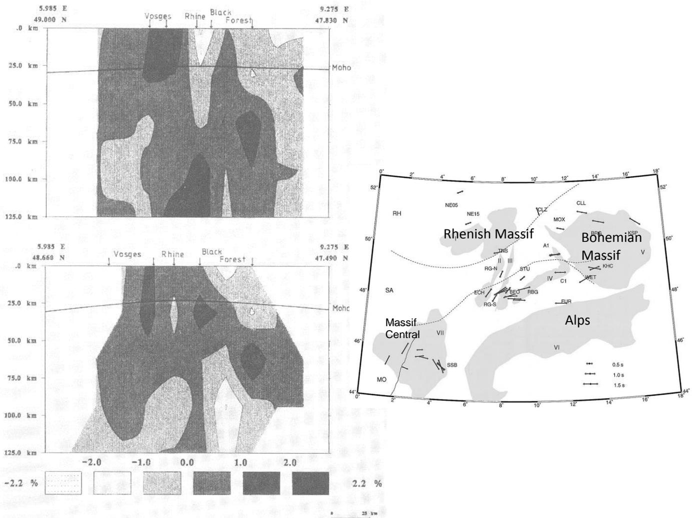
**Fig. 9.12:** Left: vertical cross sections through the 3-D model with perturbations of the P-wave velocity underneath the southern Upper Rhine Graben (for position of the sections see map in Fig. 9.11 from SFB Berichtsband 1991). Right: collection of fast polarisation directions of SKS splitting measurements in several regions of Central Europe. Mountain areas are indicated in grey, modified after Granet et al. (1998).
