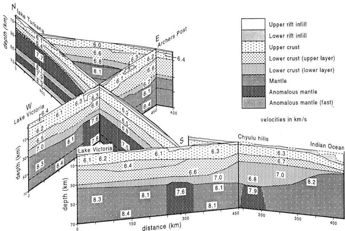
**Fig. 9-25:** KRISP 90/94 fence diagram showing crustal and upper mantle structure of the Kenya rift from Lake Turkana to Lake Magadi and beneath the neighbouring flanks from Lake Victoria to the Indian Ocean (from Khan et al., 1999, Fig. 4; Prodehl and Mooney, 2012, Fig. 9.5.1-08).
