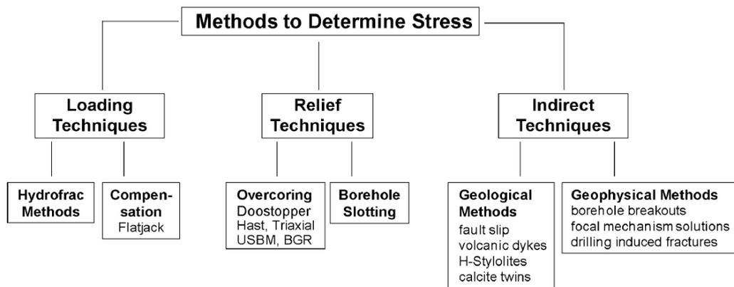
Fig. 7: Overview about the different methods to determine stress orientations or magnitudes of  $S_h$  (loading techniques) or the complete stress tensor (relief techniques).
