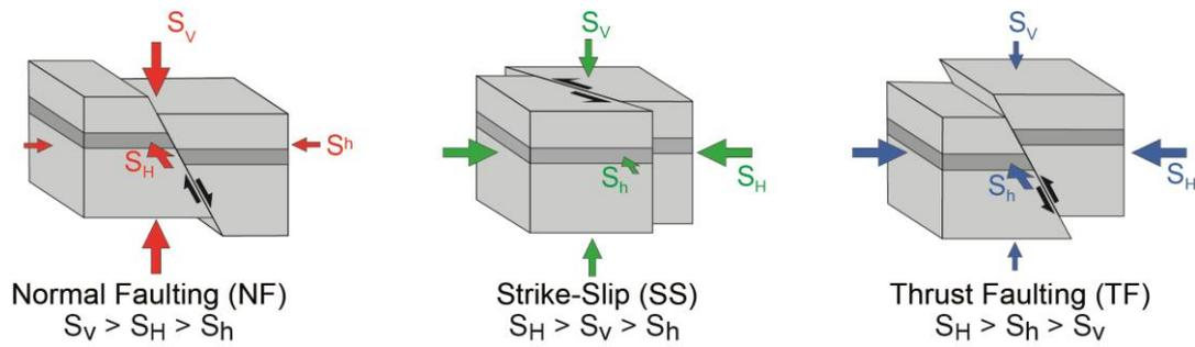
Fig. 2: Tectonic regimes and the role of the vertical stress which is the maximum principal stress in normal faulting regimes, the intermediate principal stress in a strike-slip regime and the least principal stress in a thrust faulting regime.
