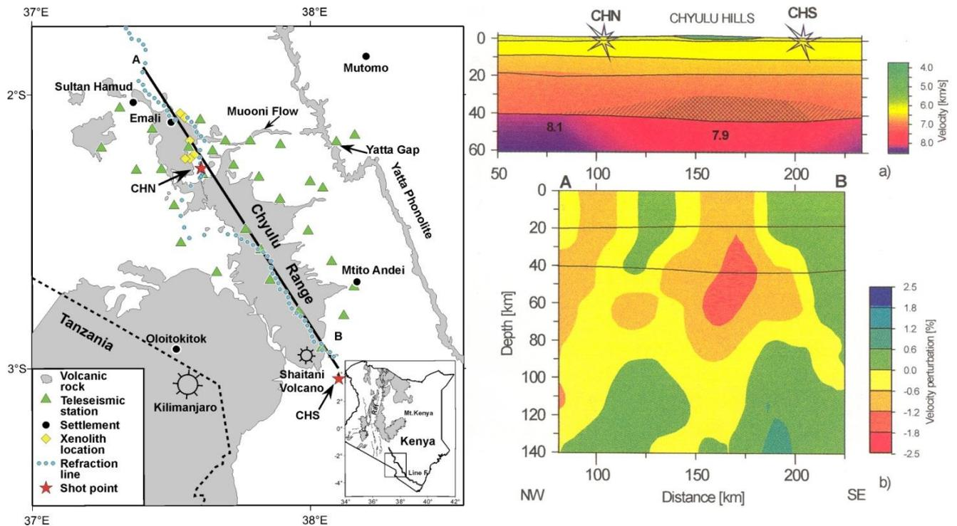
**Fig. 9.10:** Recording network (left) and model (right) of the KRISP'93 experiment in the Chyulu Hills. The models show seismic P-wave velocity combined from seismic refraction (top) and teleseismic (bottom) modelling (from Novak et al., 1997). CHN and CHS are refraction shot points (after Ritter, dissertation, 1996).
