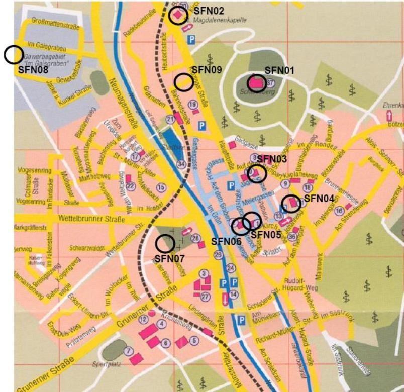
**Fig. 9.25:** Station map of the URS2 experiment (2008/09) inside the town of Staufen im Breisgau, Southern Upper Rhine Graben. The main uplift was at stations SFN06 and SFN05 in the centre.
