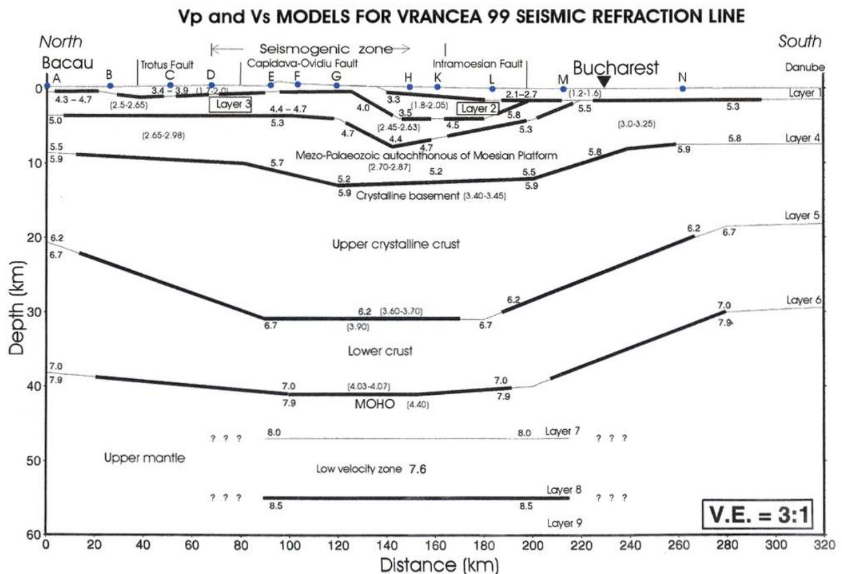
**Fig. 12-02:** Crustal P-wave cross section along the north-south profile VRANCEA 1999 (from Hauser et al., 2001, Fig. 9; Prodehl and Mooney, 2012, Fig. 9.2.4-13). Velocities in brackets are corresponding S-velocities.
