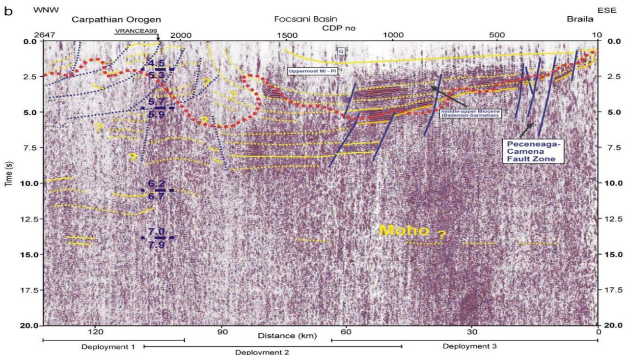
**Fig. 12-12:** Interpreted time seismic section of the DACIA PLAN seismic survey (from Panea et al., 2005, Fig. 10b; Prodehl and Mooney, 2012, Fig. 10.2.3-06). Dark blue velocity interfaces are from the VRANCEA-1999 model of Hauser et al. (2001), red dashed interface represents the 5.0 km/s velocity contour of the tomographic model of Bocin et al. (2005), blue and yellow lines – geological interpretation of the seismic-reflection data.
