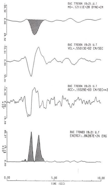
**Fig. 15:** The Vrancea earthquake of March 4, 1977: The INCERC SMAC-B recording processed by Bonjer and Apopei (1991).
