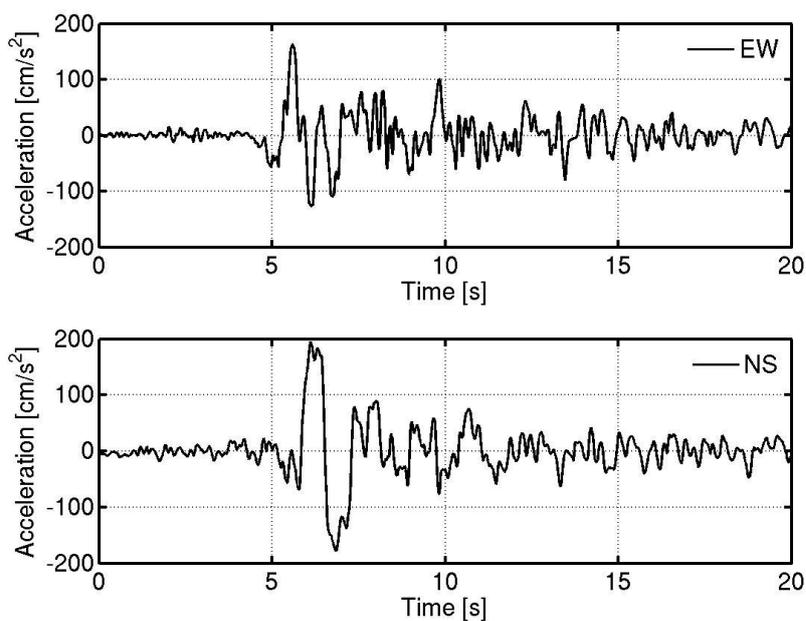
Horizontal acceleration records of the March 4, 1977 earthquake in Bucharest (INCERC). The long-period characteristic of the NS-component made engineers believe that the Vrancea events have much more lower frequencies as compared to standard Eurocode Spectra.
