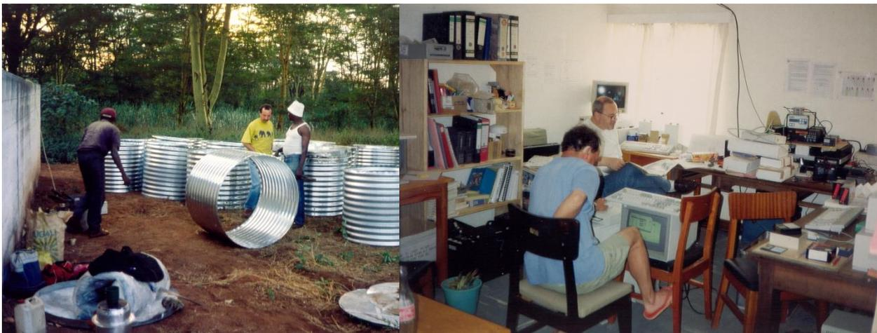
**Fig. 9.8:** Headquarter of the KRISP'93 experiment in Kiboko. Left: preparation of metal drums for recording sites (see also Fig. 9.9). The drums were later buried and fixed into a massive concrete base at the recording sites (in the centre: Raimund Stangl with local helpers). Right: office with radio communication and Jürgen Oberbeck studying a manual and Raimund Stangl fixing a computing problem.
