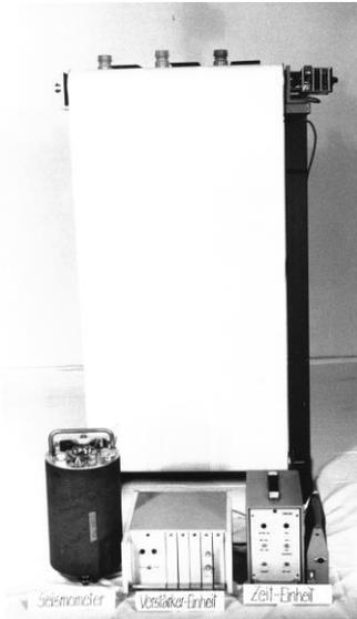
**Fig. 3:** Components of a stand-alone station. All instruments were manufactured in the labs of the GPI, with the Geotech S-13 seismometer.
