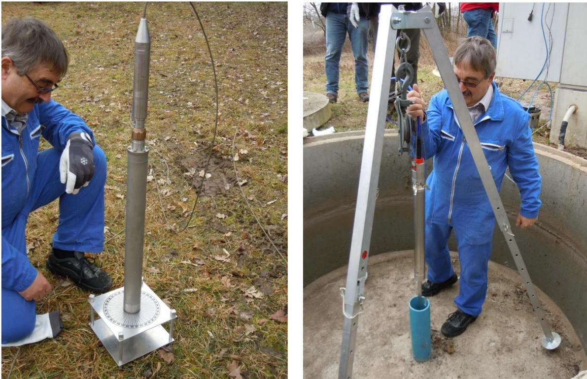
**Fig. 9.19:** Top: first test measurements with the Karlsruhe BroadBand Array near Huchenfeld, Pforzheim (from left: T. Diehl, J. Ritter & J. Mathar). Different sensor types can be seen (red: Geotech KS-2000, green: Streckeisen STS-2, blue: Lennartz 5 s, silver: Güralp 40T). Bottom: Orientation and installation of a Lennartz borehole seismometer near Landau (Fig. 9.29) with W. Walker.
