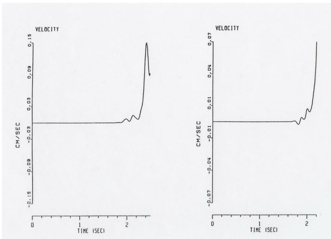
**Fig. 32:** SUR (see Fig. 33) velocity-recordings of the vertical component of the initial phases of the strong Vrancea earthquakes of August 1986 and May 1990. Note the oscillatory character of the onset. It remains still open whether or not this is due to the source processes or to structural effects at the sources or along the propagation paths.
