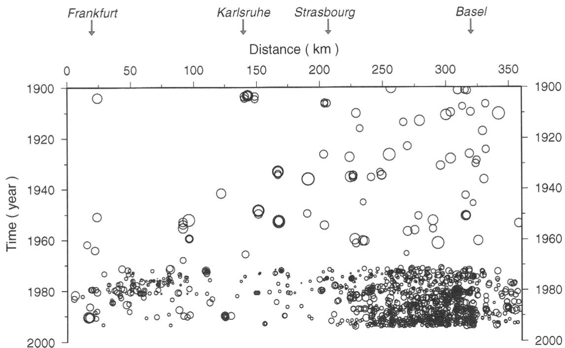
**Fig. 7:** The seismic activity in the Upper Rhinegraben between Frankfurt and Basel for the years 1900-1979. The rather abrupt increase of the seismic activity around 1971/72 is the result of the implementation of the high-gain networks of the GPI, the French networks in the Vosges Mountains and the Swiss networks in the southern end of the Rhinegraben.
