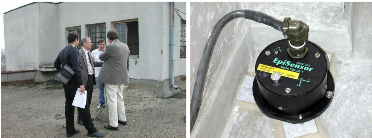
**Fig. 38:** Briefing at the top of the multi-story building: M. Bayraktarli (project C1/C2), Dan Lungu (owner of the flat, see Fig. 37), INCERC member, K.-P. Bonjer (left figure). The center EpiSensor is still without thermal protection. The ceramic isolators of the feet are visible (right figure).
