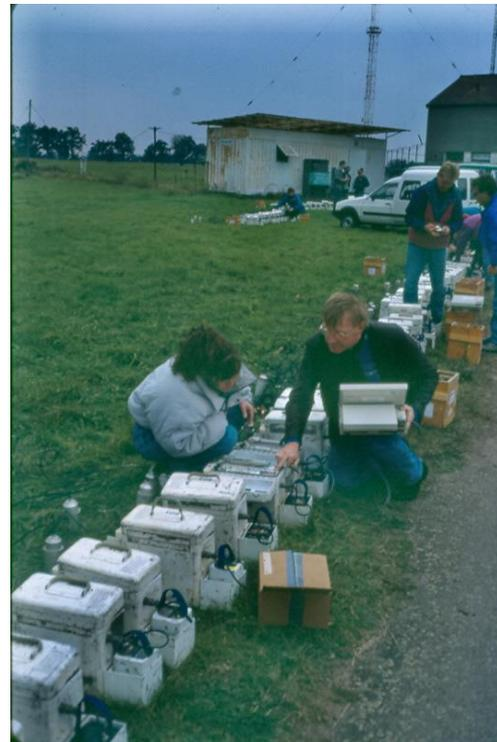
**Fig. 3-06:** Huddle Test of the SGR
