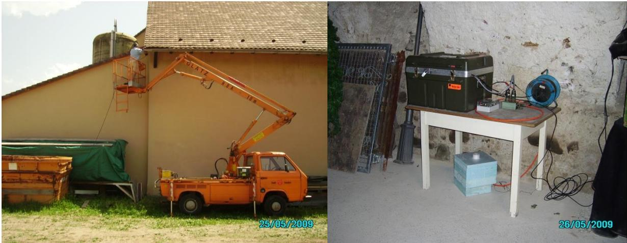
**Fig. 9.26:** Station SFN02, URS2 experiment in Staufen im Breisgau. Left: installation of a GPS antenna. Right: recording box and STS-2 seismometer (inside the blue box for thermal insulation) in a historic cellar.
