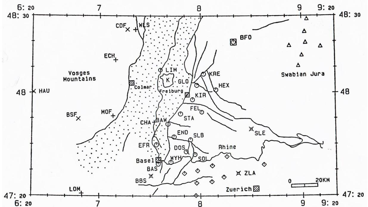
**Fig. 9:** Map of the earthquake stations in the southern Rhinegraben area: CRC 108-B3 PCM-5800 stations (circles), Nagra telemetry-network (diamonds), Swabian-Jura network of the Institute of Geophysics Stuttgart (triangles) as well as the French telemetry networks in the Vosges Mountains and the telemetry stations of the SEDZ.
