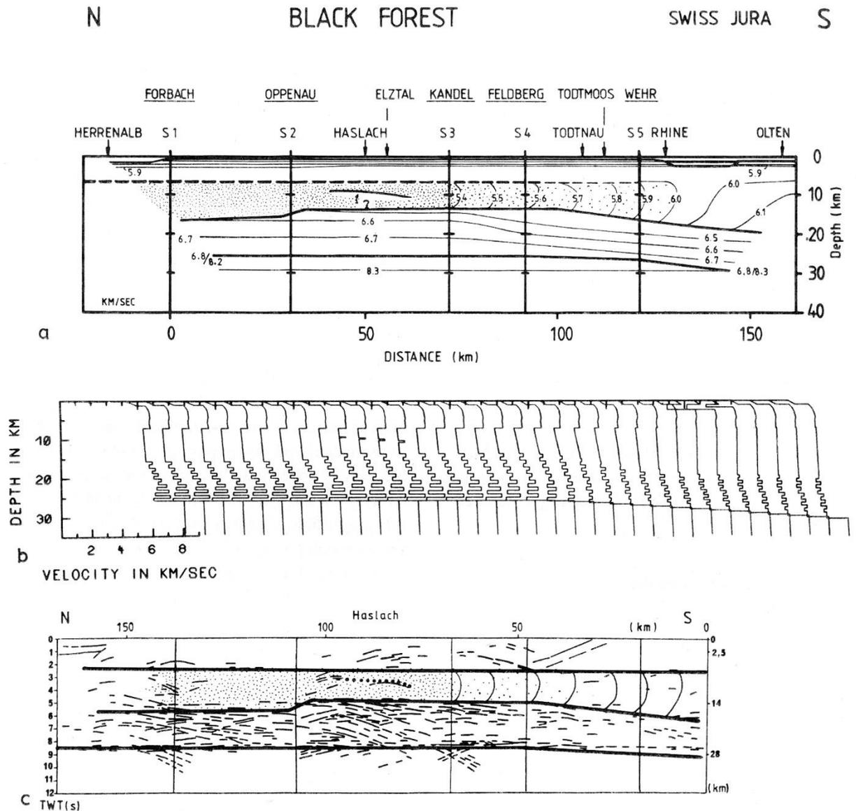
**Fig. 3-1:** Crustal model of the Black Forest (from Gajewski and Prodehl, 1987, Fig. 8; see also Prodehl and Mooney, 2012, Fig. 8.3.3-03). (a) Model with lines of equal velocity, derived from seismic-refraction data. (b) Velocity-depth sections along line S, derived from seismic-refraction data. (c) Line drawing of the seismic-reflection section along the Black Forest (simplified after Lueschen et al., 1987). Two-way travel times as calculated from model (a) are plotted as thick lines in (c).
