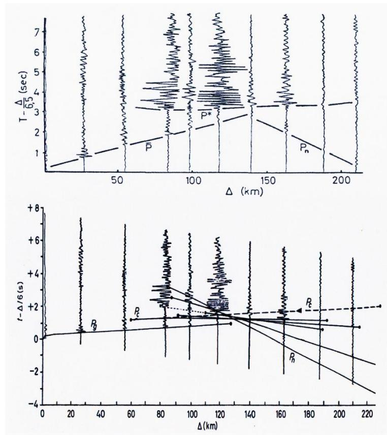
**Fig. 1-3:** Record section of the ESE profile of the blasts near Haslach in 1948
