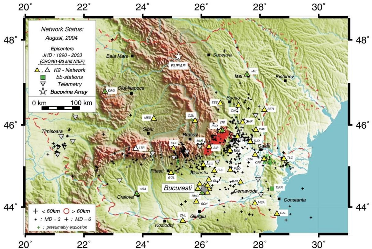
Fig. 34: Position map of the CRC 461- and NIEP K2-accelerometer stations (status of August 2004).
