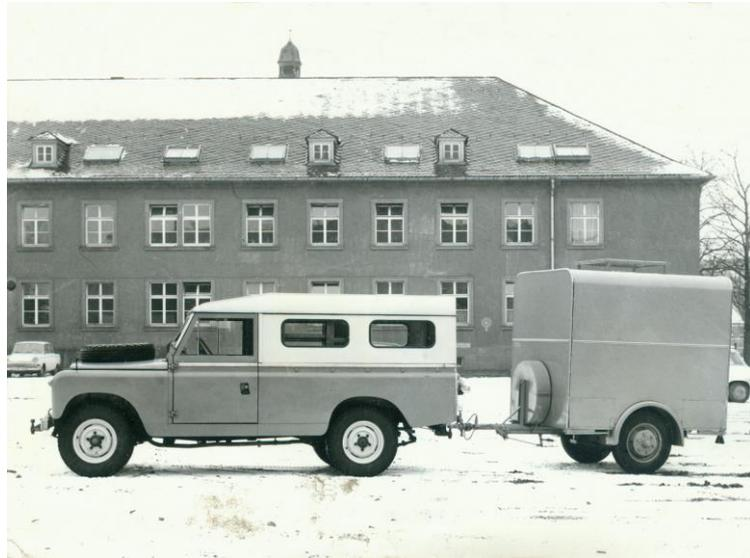
**Fig. 4:** The mobile station, assembled by the GPI. Long-duration tape recorder and ink monitor, timing unit, filters, and amplifiers, and buffered batteries were arranged in the trailer.
