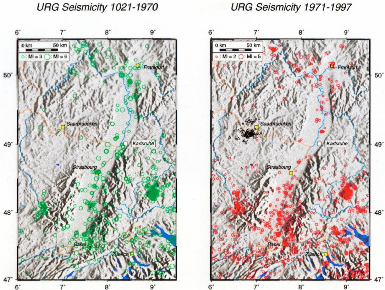
**Fig. 8:** The seismicity of the Upper Rhinegraben from 1021-1997: Period 1021-1970 (left figure; data are from an earlier version of the catalog of Leydecker, 2011); period 1971- 1997 (right figure; data are from the nrift35-file of Bonjer, 1979). Note the similarity of the distribution of 'felt' and (mostly) microearthquakes. About 25 years are seen to be sufficient to discover the significant epicentral patterns in the Upper Rhinegraben area.
