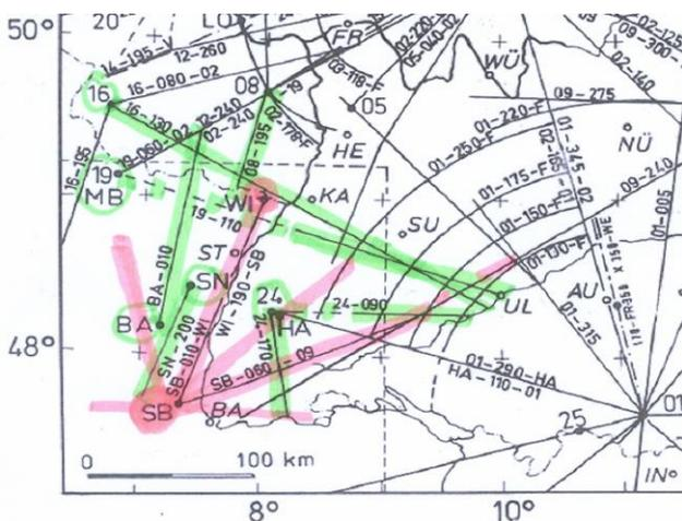
**Fig. 2-01:** Location of seismic-refraction profiles in the Rhinegraben and its surroundings until 1972 (green: quarry blast profiles, red: project 1972).
