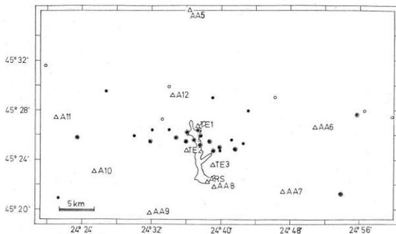
**Fig. 26:** Position map of the Vidraru-Arges survey: ARS = permanent station in the eastern abutment of the dam; T1, T2, T3 = permanently installed telemetry stations (see the survey report of November 1976); A\* = mobile stations. Located events are shown by circles.
