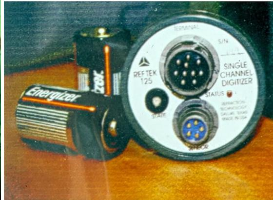
**Fig. 12-08:** Equipment: 15 „Texans“ in a box for transportation. **Fig. 12-09:** „Texan“ – RefTek-1-component station.
