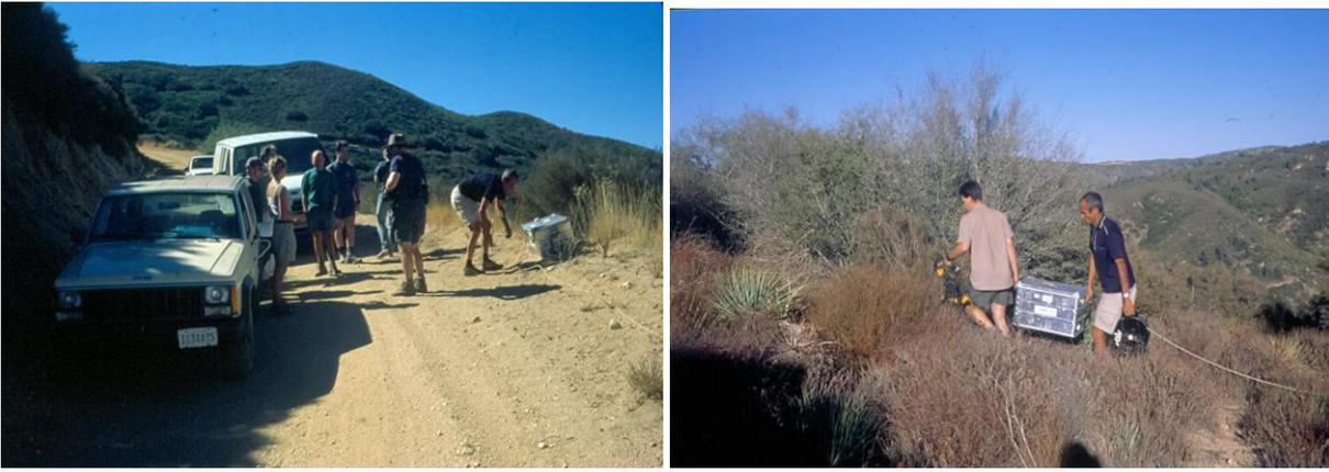
**Fig. 11-14** and **Fig. 11-15**: GFZ-6-channel stations with 6 vertical seismometers being connected to the central station by long cables are being deployed in difficult terrain in the Susanna Mountains north of Los Angeles.
