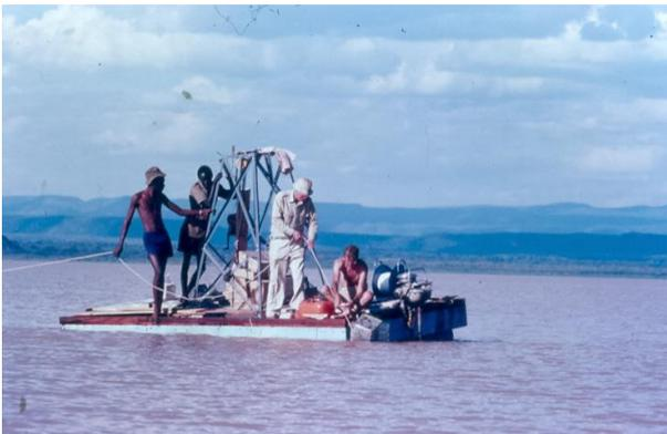
**Fig. 9-03:** Don Griffith's raft to lower seismic charges.
