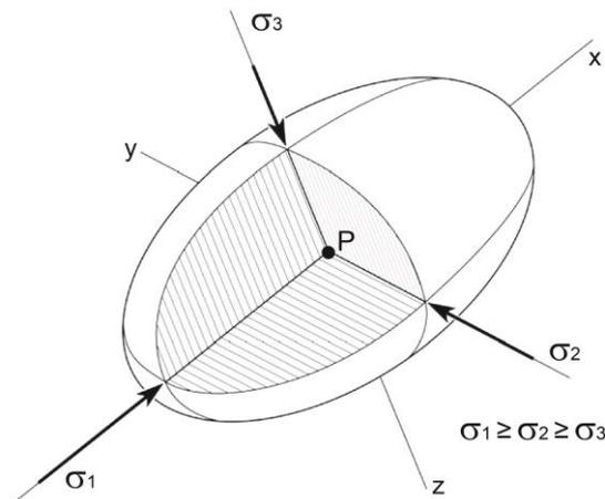
Fig. 1: Lamé stress ellipsoid. The three principal stresses (Eigenvectors)  $\sigma_1$ ,  $\sigma_2$  and  $\sigma_3$  of the symmetrical stress tensor  $\sigma_{ij}$  describe the state of stress at a point P.
