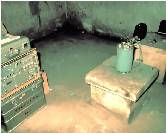
The Mainka seismograph was used routinely for the event recording and magnitude determinations over decades. The parallel recording was considered necessary to prove a presumed deficit in the 5.5-6.5 magnitude range of the Vrancea earthquakes.
