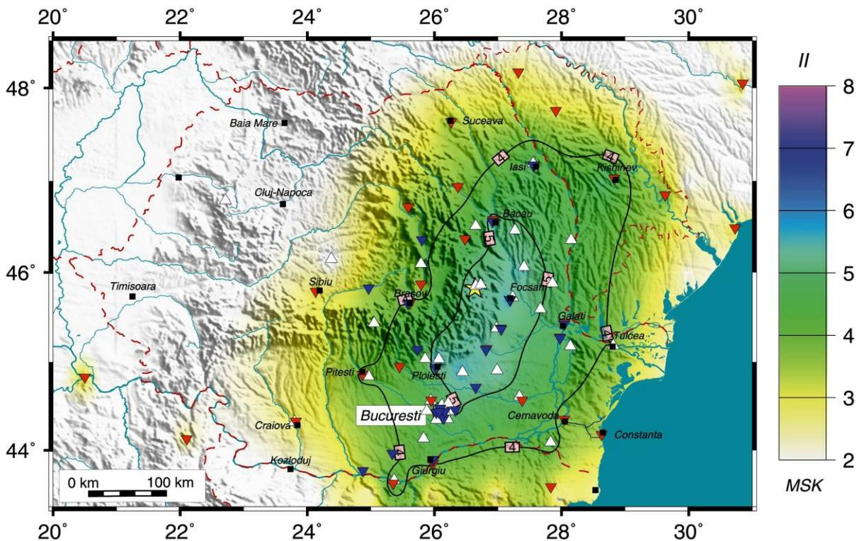
**Fig. 44:** Shakemap of the Vrancea Mw=5.8 earthquake of October 27, 2004 (Bonjer et al., 2008; Bonjer, 2012): The intensities (II) are determined from accelerograms (white triangles: CRC-NIEP K2-data; blue triangles: INCERC-UTCb data) and from the observed intensities from the Community Internet Intensity Map data (Wald et al., 1999).
