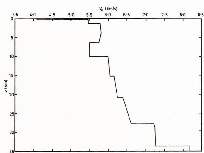
**Fig. 1-4:** Crust with low-velocity zone beneath a high-velocity lid (model of Landisman et al., 1966)
