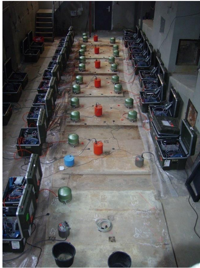
Fig. 13-1: Calibration test with the KABBA instruments in the basement of KIT-GPI. The mobile recording units measured coincidentally for two months in order to detect possible instrument malfunctions and to compare the instrument response functions.
