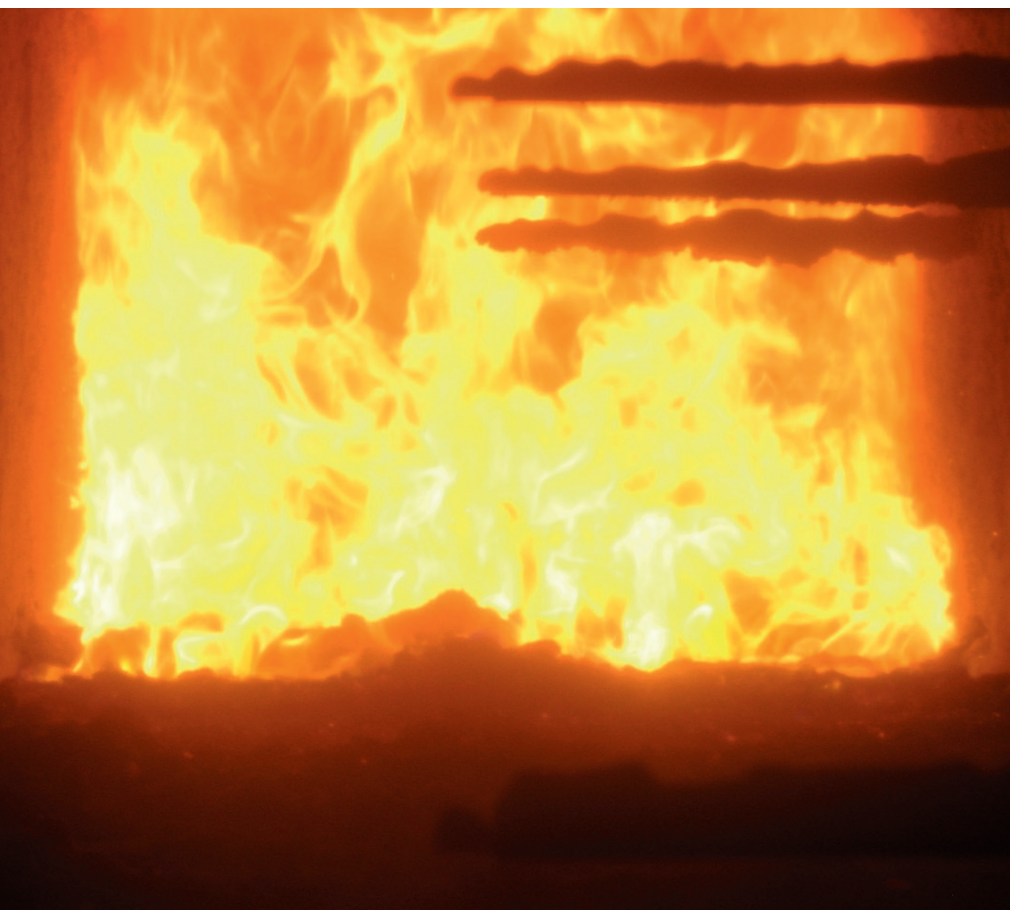
The TAMARA pilot plant for grate combustion at KIT: view into the combustion chamber.
