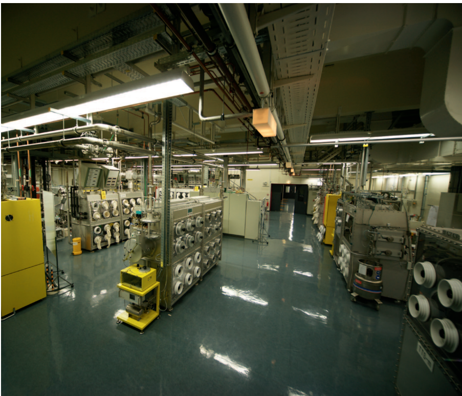
The main experimental hall of TLK with several glove boxes for experiments using tritium.
