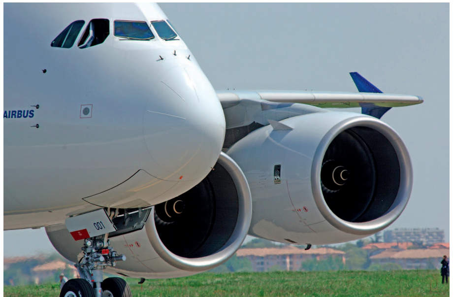
Airbus A380, equipped with Rolls-Royce Trent 900 turbofan engines. (This photograph is reproduced with the permission of Rolls-Royce plc, copyright © Rolls-Royce plc 2012.)
