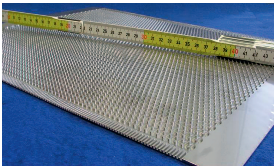
A structured reaction plate designed for a reactor that produces synthetic diesel fuel.
