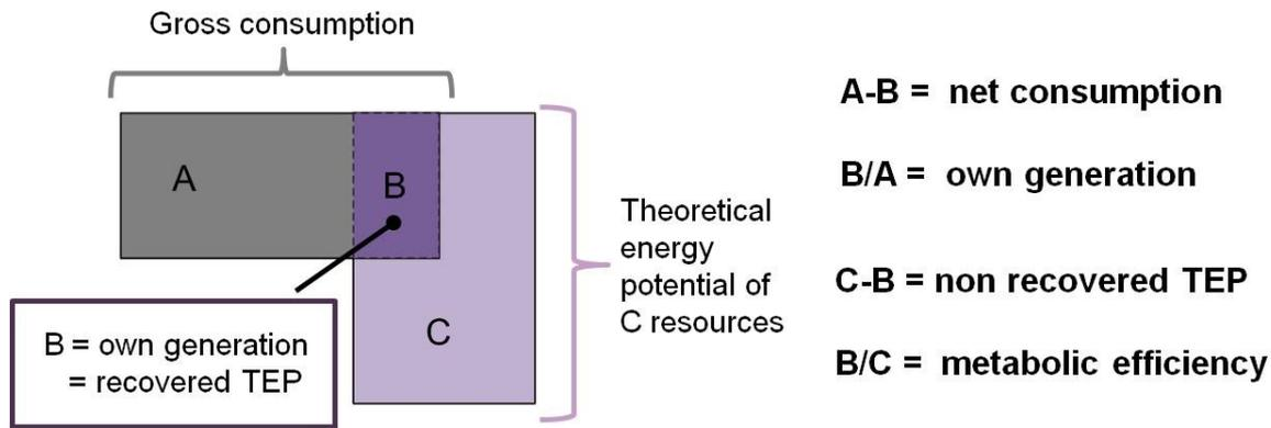
Figure 2-2: Elements of the extended energy balance
