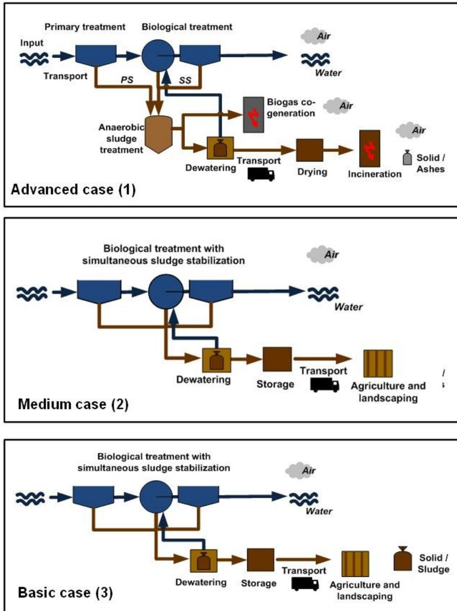
Figure 3-1: Status quo: Three cases for wastewater and sludge treatment
