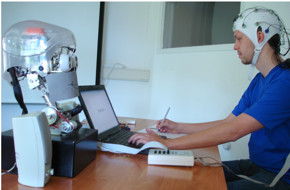
Figure 4.3 – Recording setup with ROBERT (left side), the Computer for the secondary task (center) and participant wearing an EEG cap (right side).
