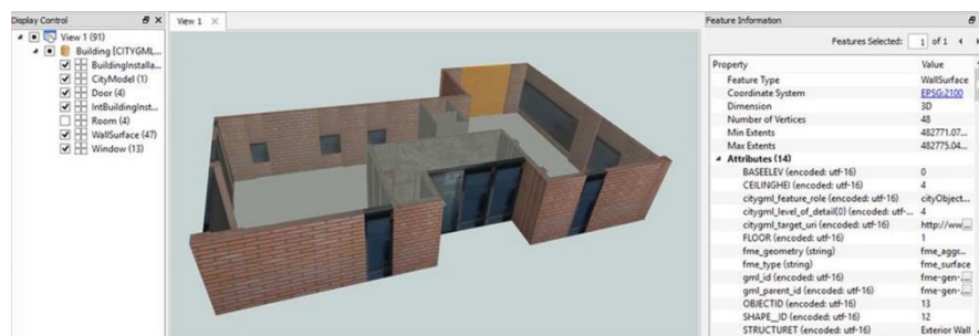
Fig. 5 CityGML Building Model in FME Data Inspector
