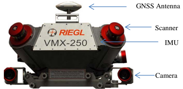
Figure 11 – Riegl VMX-250 system used to measured the point cloud used in test site 1
