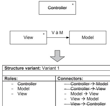
Figure 4.16.: An Example of a Textual Representation for the Model View Controller Pattern Variant
