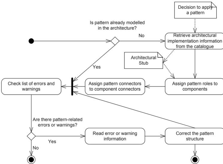
Figure 3.13.: Activity Diagram of Check Architectural Implementation Violations Use Case
