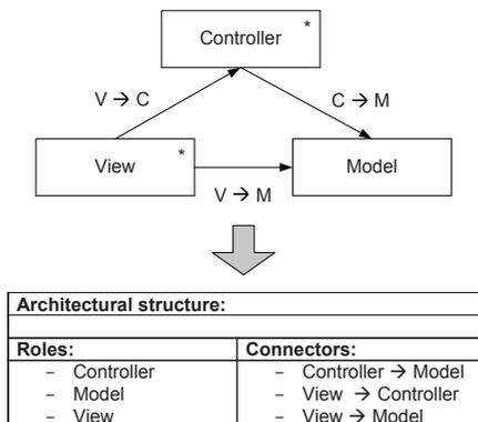
Figure 4.15.: An Example of a Textual Representation for the Model View Controller Pattern
