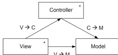
Figure 4.11.: An Example of Roles and Connectors Representation for the Model View Controller pattern
