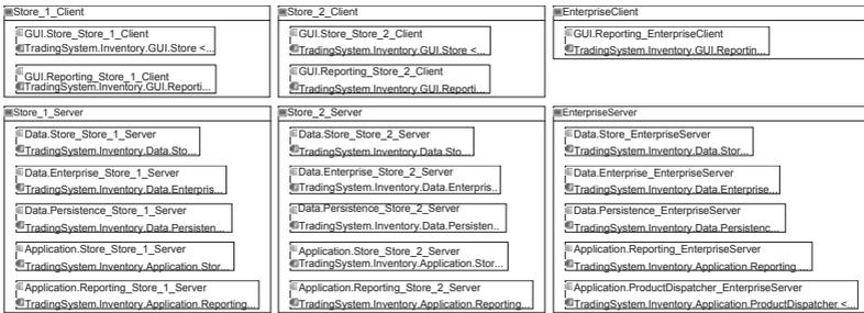
Figure 3.20.: Deployment Model of the CoCoME Architecture in PCM System View [158] (Repetition from Section 2.5.2)
