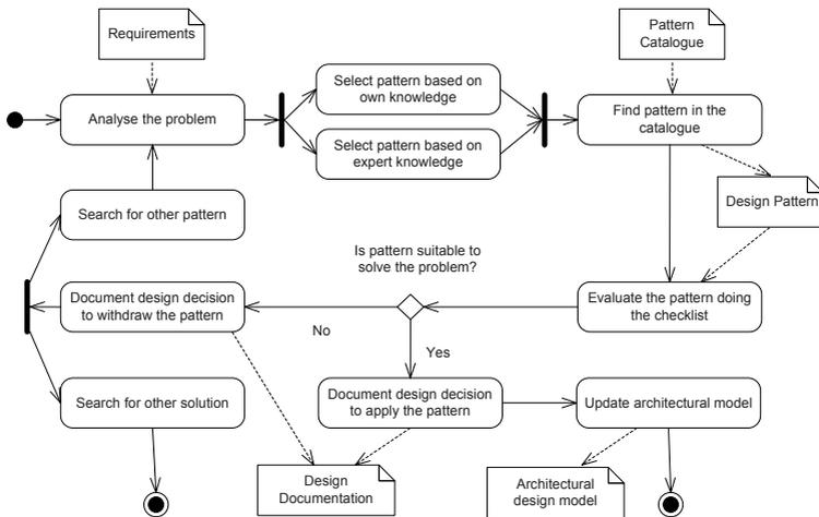
Figure 3.6.: Activity Diagram of Pattern Application Use Case
