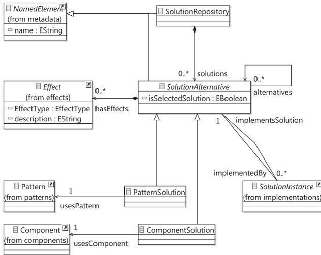
Figure 4.31.: Solutions Meta-Model Package
