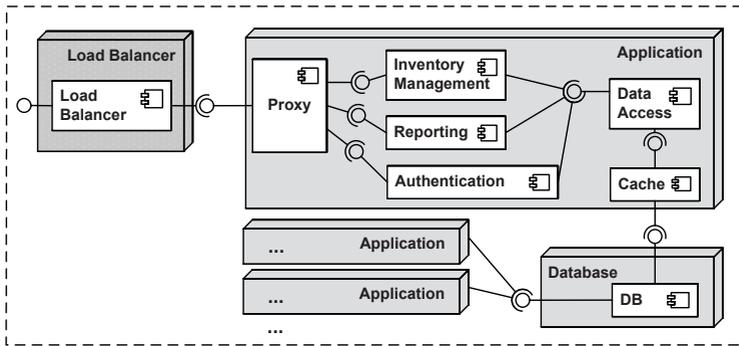
Figure 3.24.: Modified Hexxon CoCoME Architecture of the Enterprise Server (Adopted from [2])
