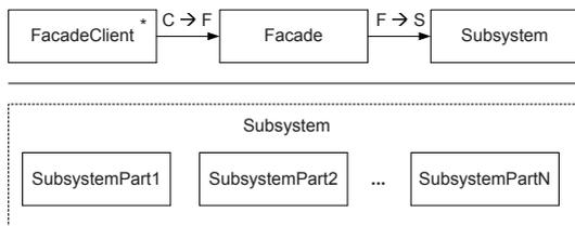
Figure 4.12.: An Example of Roles and Connectors Representation for the Façade Pattern
