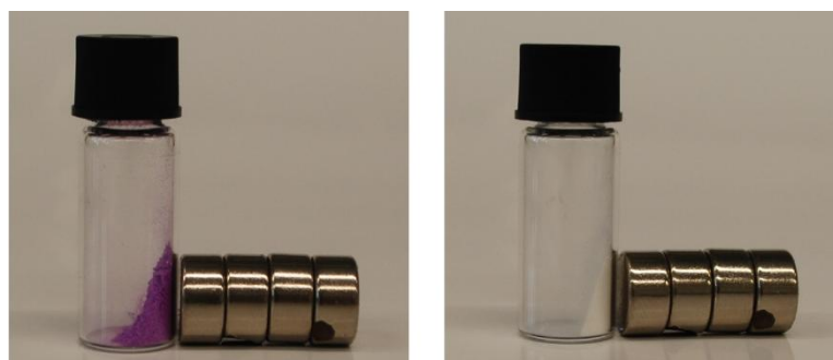
Figure 101: Pictures of the dried Co(PP) (left) and (Gd) 2 (PP) 3 (right) nanoparticles and their behavior in an external magnetic field.
