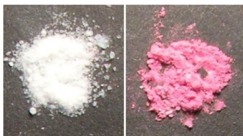
Figure 53: Nanoscale AIO(OH) hollow spheres (left) and DXR-filled AIO(OH) hollow spheres (right).
