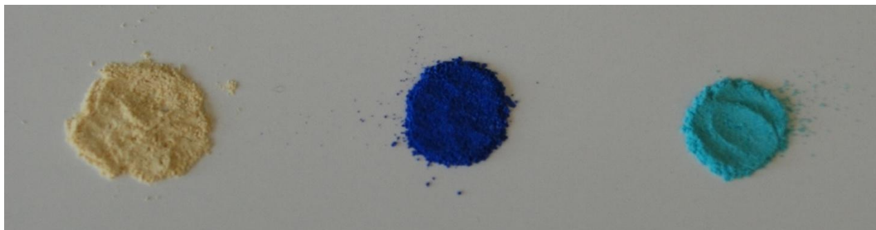
Figure 88: Picture of the final dried materials obtained combining aminoethyl phosphonic acid with different transition metal cations: Fe(2-AEP) yellow, Co(2-AEP) dark blue and Cu(2-AEP) light blue.
