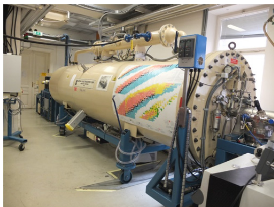
Fig. 5: The vessel filled with SF 6 at a pressure of about 6 bar which contains the +3-MV tandem accelerator of VERA (Pelletron type, model 9SDH-2).
