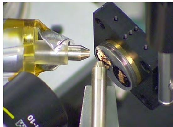
Fig. 2: Polycapillary setup for  $\mu$ -XAFS/XRF measurements at the INE-Beamline – the SDD is depicted with a secondary capillary mounted for confocal measurements (in-depth resolved).
