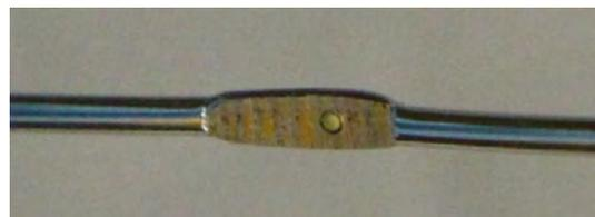
Fig. 1: Microsphere placed in the hole of the wire before measurements.
