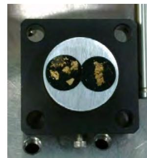
Fig. 1: Dried and lacquer-fixed sludge material (sample A left, sample B right) was not investigated), mounted on ESCA sample holder for  $\mu$ -XAFS/XRF investigations.
