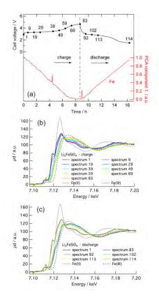
**Figure 1.** (a) Voltage profile during *in situ* XAS experiment for the first charge/discharge cycle of Li<sub>2</sub>FeSiO<sub>4</sub> against Li metal in the voltage range 1.5-4.7 V at a current density of 20.6 mA g<sup>-1</sup> (i.e., C/16) together with component 1 of the PCA. The corresponding Fe *K*-edge absorption spectra during (b) charge and (c) discharge.
