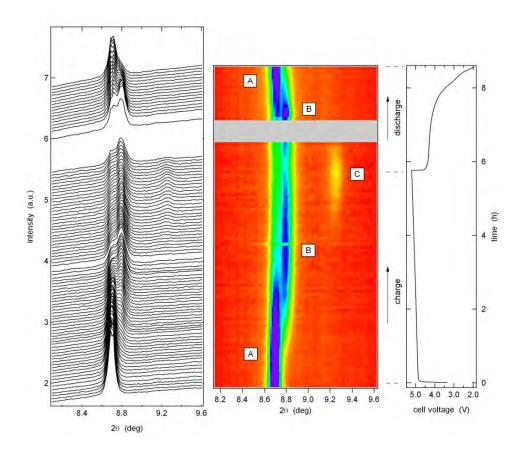
Fig. 1: In situ XRD measurements on olivine  $LiCoPO_4$  during galvanostatic cycling against Li metal in a battery cell. The voltage profile as a function of time is shown on the right side.
