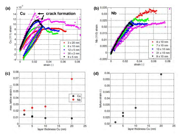
**Fig. 2:** Exemplary results of the in situ diffraction testing. (a), (b) Lattice strain as function of the total strain determined from the (111) fcc Cu and (110) bcc Nb reflection, respectively. (c) Maximum Cu and Nb lattice strain and (d) failure strain of the Cu layer as function of the Cu layer thickness.
