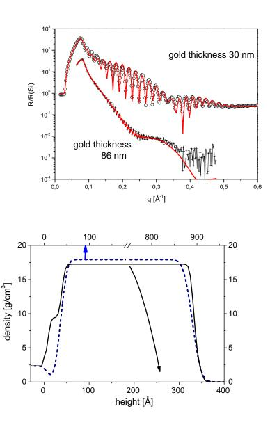
Fig. 1a: XRR of two representative thin films of gold on top of silicon. The 30 nm film has a nominally 2 nm chromium film as interlayer. Fits (red lines) are done with a 4-layer model.
