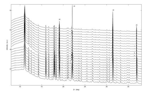
Fig. 2: In situ XRD measurements on non-olivine LiCoPO<sub>4</sub> during galvanostatic charging (top to bottom) against Li metal in a battery cell.
