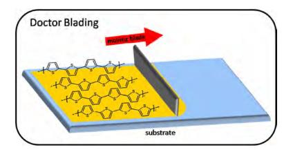
**Fig.1:** Schematic setup of doctor blade casting, applied for the preparation of the thin polymer films.
