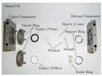
Fig. 1: A) Exploded view of the hydrothermal cell.
