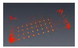
**Figure 2:** 3D rendering of a SRCL scan of micro solder bumps on flip chip at TopoTomo. Resolution  $6.71 \mu m$ .
