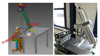
spectrometer motors. The stationary detector positioning unit has three degrees of freedom (a long and a short linear stage and a rotation stage), which allow the detector to be moved along the Rowland circle. Mechanical spectrometer performance tests and adaption of the control software, as well as commissioning, have been performed and the spectrometer is now installed for use at the INE-Beamline for actinide research.
