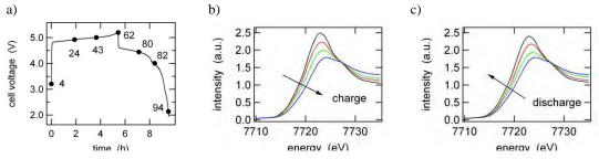
**Figure 3.** (a) Voltage profile during *in situ* XAS experiment for the first charge/discharge cycle of LiCoPO<sub>4</sub> against Li metal in the voltage range 2.5-5.2 V. The corresponding Co *K*-edge absorption spectra during (b) charge and (c) discharge.
