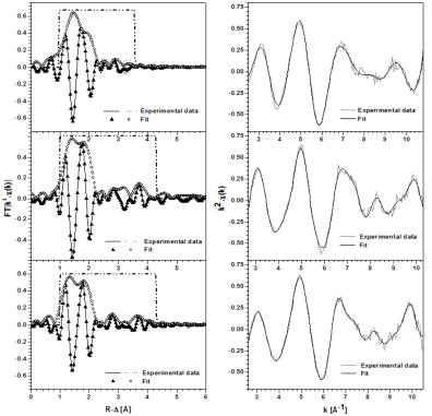
**Fig. 1:** k2-weighted Np L3-edge EXAFS  $\chi(k)$  of neptunium solubility limiting solid phases: green (top), white (middle) and violet (bottom) and respective Fourier transforms. Data are depicted as solid lines, fits as circles and triangles.
