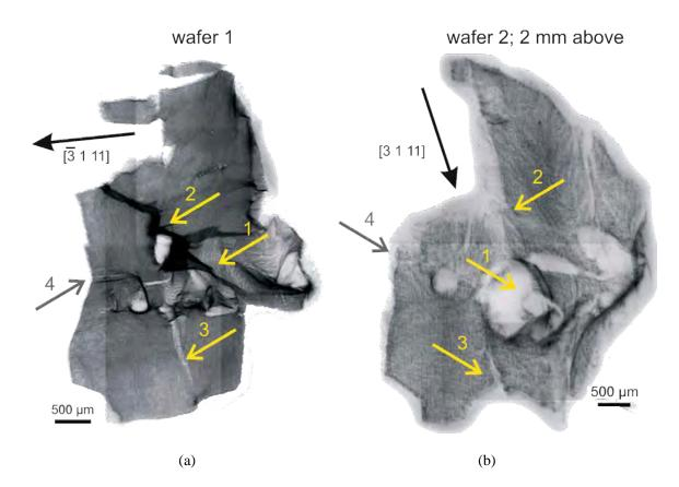
**Fig. 2:** 3 1 11topographs showing the evolution of small-angle grain boundaries and accumulations of dislocations of one grain during 2 mm of growth from wafer 1 (a) to wafer 2 (b): Larger accumulations of dislocations in positions 1 - 3 extend, while small-angle grain boundaries in pos. 4 vanish.
