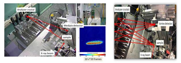
Fig. 2: Photo of the MAC-Spectrometer in dispersive (left) and scanning geometry (right) during commissioning at the INE-Beamline. The image measured with the Medipix detector shows focused Cu K $\alpha_1$  emission (left).
