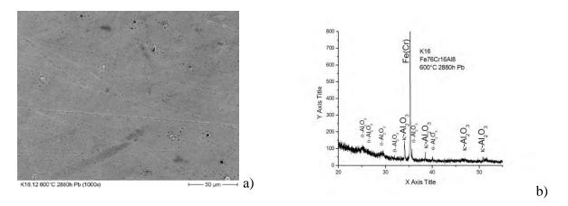
*Fig. 2:* Surface morphology (SEM - a) and XRD pattern (GI-XRD - b) of a multilayered Al<sub>2</sub>O<sub>3</sub> scale grown during 2880h exposure to molten Pb, at 600 °C.
