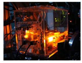
Fig. 2: Experimental set-up for in-situ XAS measurements (sample temperature is 1670 K).
