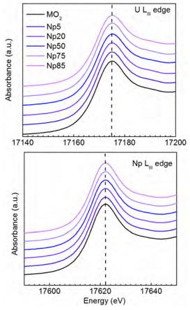
Figure 1: XANES spectra at the U LIII and Np LIII edges of MO2 (M=U or Np) and of the U1xNpxO2 samples.
