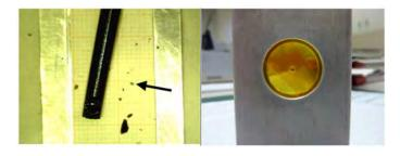
Fig. 1: HAWC glass fragment (arrow) selected for investigation at INE-Beamline (left, scale in mm); glass fragment inside a double containment mounted in the sample holder (right) prior to the transport to ANKA.
