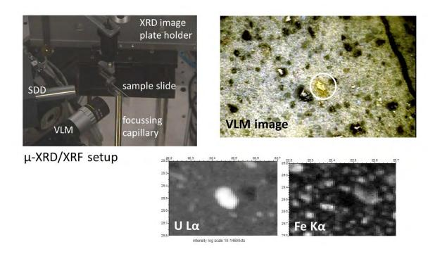
**Fig. 1:** top left -  $\mu$ -XRD/XRF setup at INE-Beamline; top right - visible light microscopy (VLM) image of U-rich hot spot in sample F33-B1-50 (marked by circle); bottom - U L $\alpha$  and Fe K $\alpha$  fluorescence maps (scale in mm) recorded with a silicon drift detector (SDD) showing U-Fe anti-correlation (cf. [1] for sample nomenclature).
