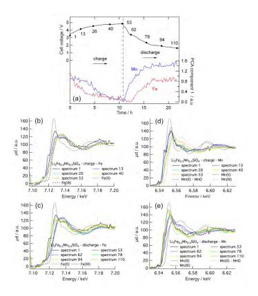
**Figure 2.** (a) Voltage profile during *in situ* XAS experiment for the first charge/discharge cycle of  $\text{Li}_2\text{Fe}_{0.5}\text{Mn}_{0.5}\text{SiO}_4$  against Li metal in the voltage range 1.6-4.8 V at a current density of 16.5 mA g<sup>-1</sup> (i.e., C/20) together with component 1 of the PCA of both edges. The corresponding Fe *K*-edge absorption spectra during (b) charge, (c) discharge and Mn *K*-edge absorption spectra during (d) charge, (e) discharge.
