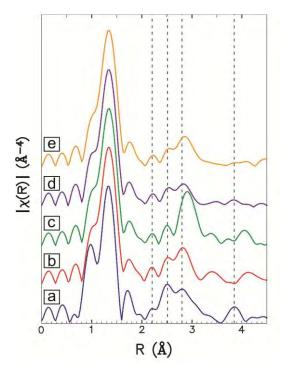
Fig. 2. FT EXAFS spectra of a) As-hematite, b) angelellite, c) scorodite, d) kaňkite, e) parasymplesite.
