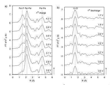
Fig. 1: Fourier transforms (FT) of  $k^2\chi(k)$  collected a) during  $1^{st}$  charge at the Fe K-edge and b) during  $1^{st}$  discharge at the V K-edge of the *in situ* battery cell. The plots are offset by 1 and the *R*-scale was not corrected for the phase shift of the absorber atom.
