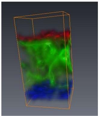
Fig. 1 Ni (gr), Ga (bl) Cu (r): 3D fluorescence images over an area of  $100x100x200 \ \mu m^3$  with the current collector at the bottom, Ni in the bulk material and Cu on top at the E/S interface
