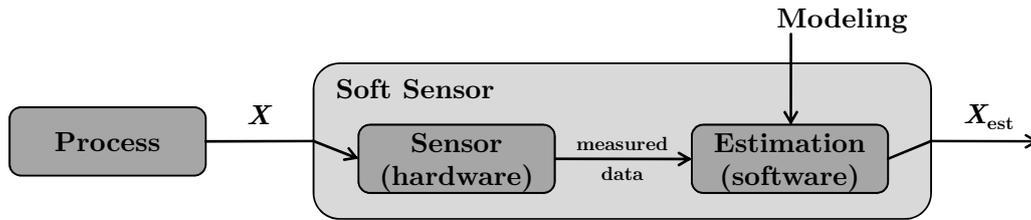
Figure 2.1: General principle of a soft sensor based on a process model. State variables  $X$  are measured by a hardware sensor, and an estimated output  $X_{\text{est}}$  is generated using a software estimator based on process modeling [CHÉRU Y 1997].
