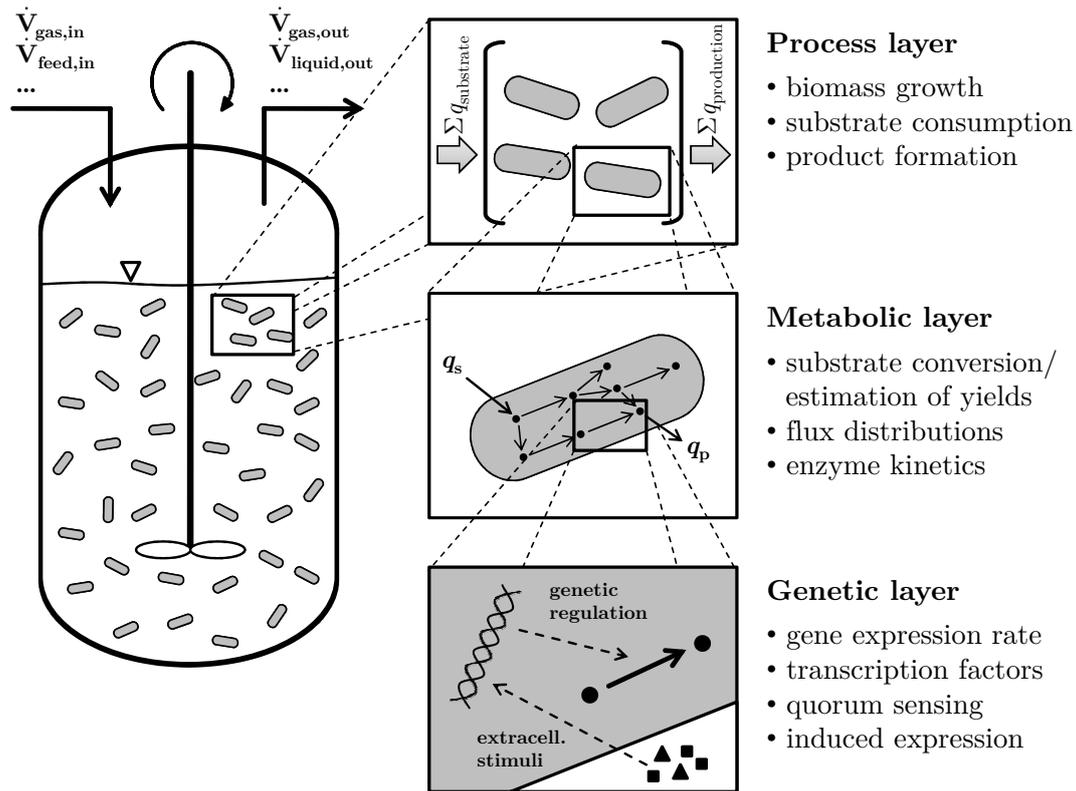
Figure 2.2: Different layers of modeling for a process in a bioreactor.
