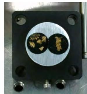
Fig. 1: Dried and lacquer-fixed sludge material (sample A left, sample B right) was not investigated), mounted on ESCA sample holder for  $\mu$ -XAFS/XRF investigations.
