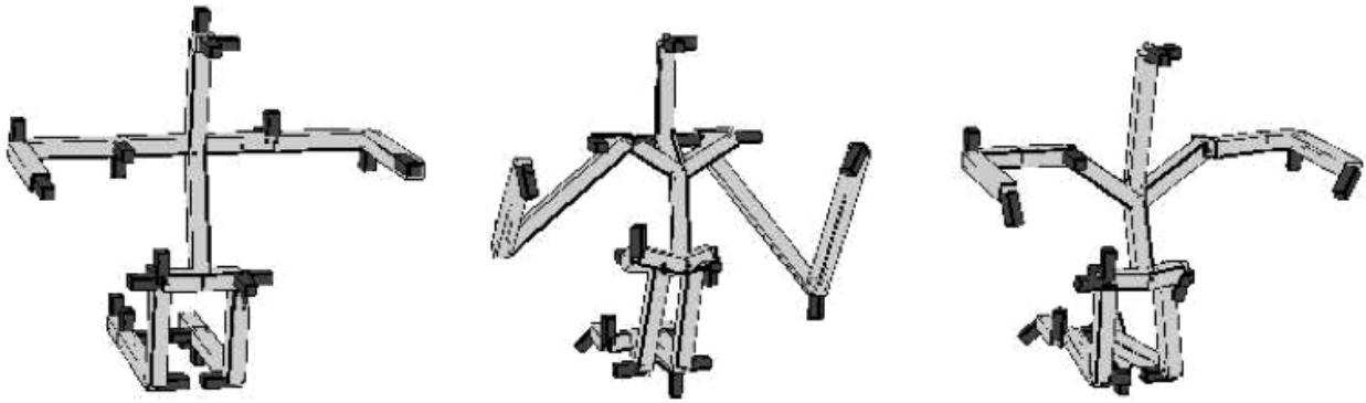
Figure 2.5.: Example of the ‘subjective body schema’ in (Hersch et al., 2008). On the left, the real (‘objective’) body of the robot is shown while two images on the right show possible (‘subjective’) valid variants of the same robot. Source: (Hersch et al., 2008)
