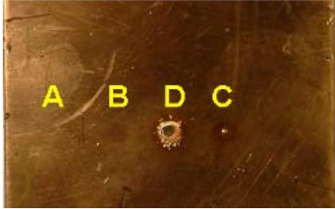
Figure 1.1.: Copper targets irradiated with a 450 GeV LHC beam to show the damage potential of the beam. The locations marked A,B,C,D are irradiated with different intensities, which are as follows: A:  $1.3 \times 10^{12}$ , B:  $2.6 \times 10^{12}$ , C:  $5.3 \times 10^{12}$ , D:  $7.9 \times 10^{12}$  protons. The plate shown was about 4.7 cm deep inside a target consisting of several layers of various target materials [Kai05].
