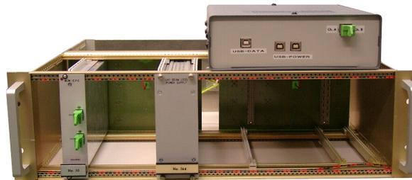
Figure 4.12.: Picture of the USB readout together with the tunnel card electronics and a power supply module for the tunnel card [Mül11].
