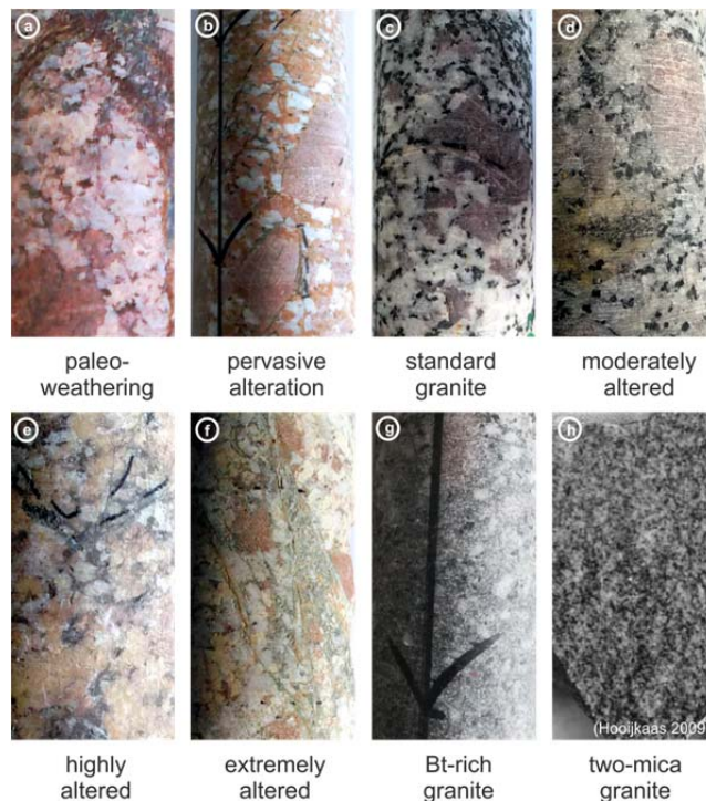
Figure 3-3: Different alteration types and grades of the porphyritic Soultz granite as observed on drill core samples (a-g) and a sample of the lower two-mica granite (h).
