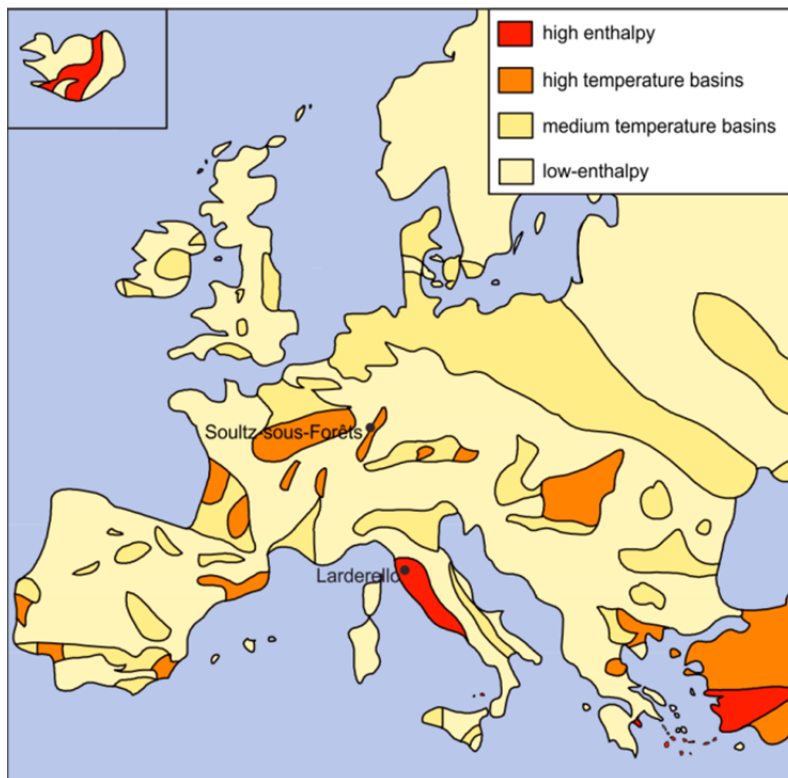
Figure 1-2: Main geothermal resources in Europe [modified after Antics and Sanner, 2007]. The major part of Europe is characterized by a medium temperature to low-enthalpy underground suited for EGS only. In 1913, a high-enthalpy reservoir in Larderello (Italy) was for the first time used for geothermal electricity production. In the 1990s, a European EGS prototype was installed in the crystalline basement of the Upper Rhine Graben (Soultz-sous-Forêts, France).
