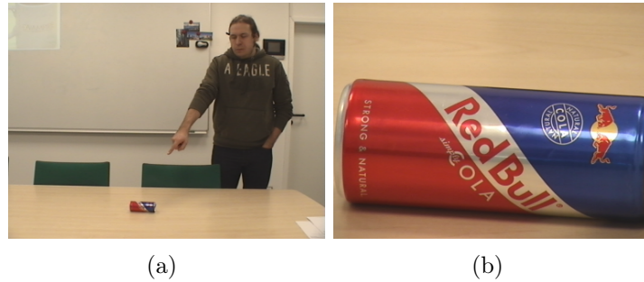
Figure 4.14.: Exemplary acquisition of an object model for the ReferAT dataset’s object database. The trainer points to an objects that is then automatically identified (a). Then, the system automatically estimates the target object’s size and uses the camera’s zoom functionality to obtain a close-up image (b).
