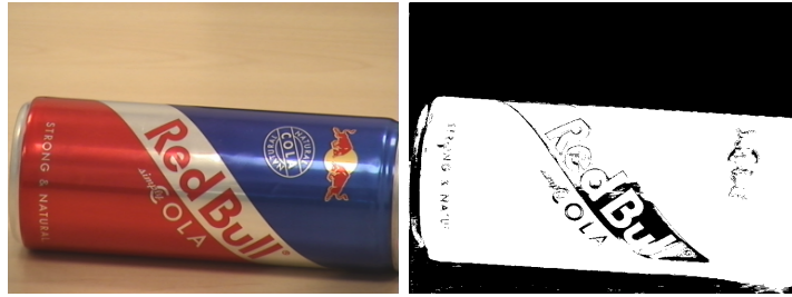
(a) Known target object’s model view and its segmentation mask obtained with color spatial variance.
