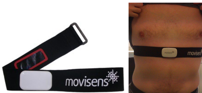
Figure 5.3: ekgMove sensor: belt with dry electrodes on the left, worn around the chest on the right.
