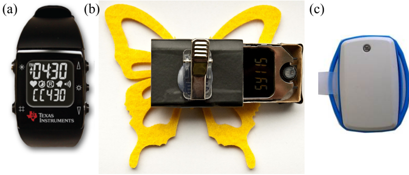
Figure 6.2: CaReflect hardware iterations: (a) original Chronos eZ430 watch, (b) prototype of the wearable badge used during the first study, and (c) final robust badge case
