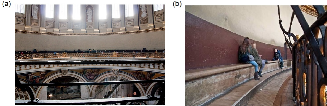
Figure 2.1: (a) St. Paul's cathedral church in London (flickr.com). (b) The whisper at one end of the wall is heard at the other end due to the repeated reflection of the acoustic wave near the the curved boundary of the wall (wanderstories.com).
