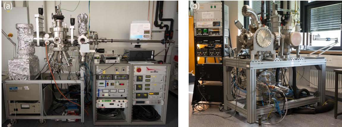
**Figure A.2:** (a) UHV metal evaporator (Beckmann group), (b) HV metal evaporator (Schimmel group).
