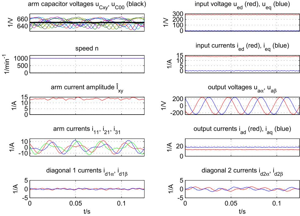
Fig. 5: Measurement of the M3C control variables at a machine speed of  $1000 \text{ min}^{-1}$ , short time averaged values at  $t_A = \frac{1}{f_{\text{PWM}}} = \frac{1}{8 \text{ kHz}}$ .
