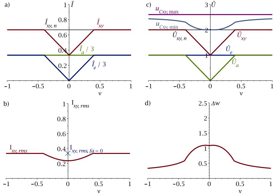
Fig. 2: Operation of a synchronous machine at constant torque below  $|v| = 0.4$  and constant power above  $|v| = 0.4$ : a) arm current amplitude components  $\hat{I}_{xy}$ ,  $\frac{\hat{I}_a}{3}$ ,  $\frac{\hat{I}_e}{3}$ ; b) arm current rms-value  $I_{xy,rms}$ ; c) arm voltage amplitude components  $\hat{U}_{xy}$ ,  $\hat{U}_e$ ,  $\hat{U}_a$ ; d) maximum energy pulsation  $\Delta w$  (all pu values)
