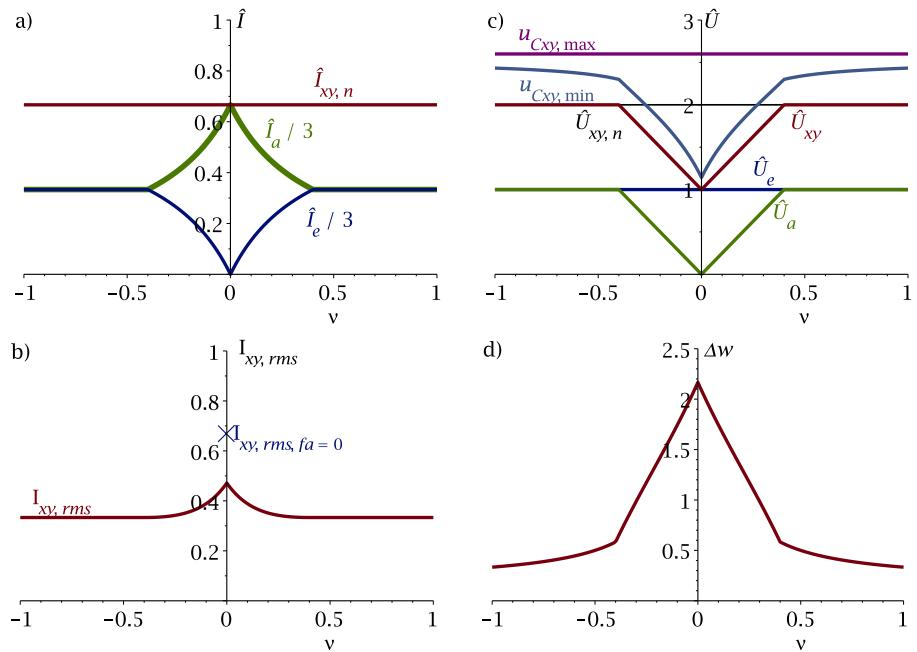
Fig. 3: Operation of a synchronous machine at a constant rated arm current amplitude  $\hat{I}_{xy,n}$ : a) arm current amplitude components  $\hat{I}_{xy}$ ,  $\frac{\hat{I}_e}{3}$ ,  $\frac{\hat{I}_a}{3}$ ; b) arm current rms-value  $I_{xy,rms}$ ; c) arm voltage amplitude components  $\hat{U}_{xy}$ ,  $\hat{U}_e$ ,  $\hat{U}_a$ ; d) maximum energy pulsation  $\Delta w$  (all pu values)
