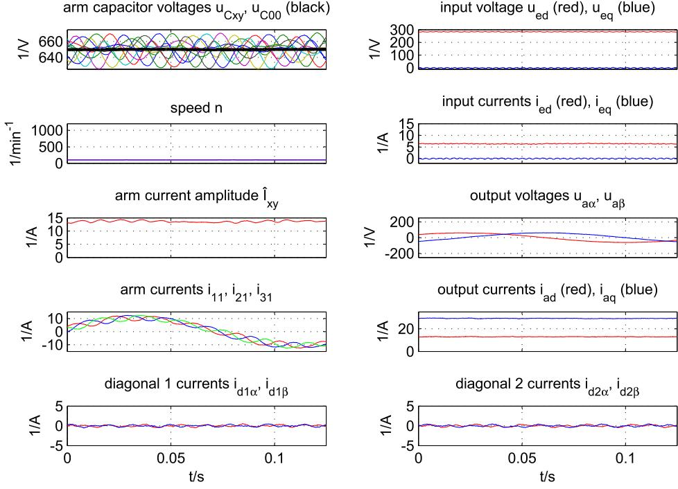
Fig. 4: Measurement of the M3C control variables at a machine speed of  $100 \text{ min}^{-1}$ , short time averaged values at  $t_A = \frac{1}{f_{\text{PWM}}} = \frac{1}{8 \text{ kHz}}$ .
