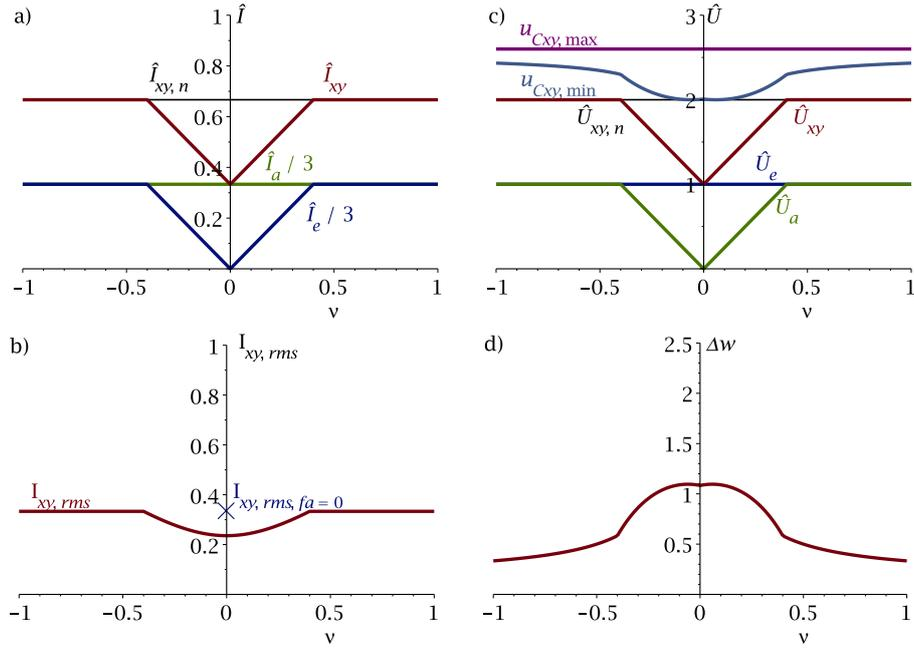
Fig. 2: Operation of a synchronous machine at constant torque below  $|\nu| = 0.4$  and constant power above  $|\nu| = 0.4$ : a) arm current amplitude components  $\hat{I}_{xy}$ ,  $\frac{\hat{I}_e}{3}$ ,  $\frac{\hat{I}_a}{3}$ ; b) arm current rms-value  $I_{xy,rms}$ ; c) arm voltage amplitude components  $\hat{U}_{xy}$ ,  $\hat{U}_e$ ,  $\hat{U}_a$ ; d) maximum energy pulsation  $\Delta w$  (all pu values)
