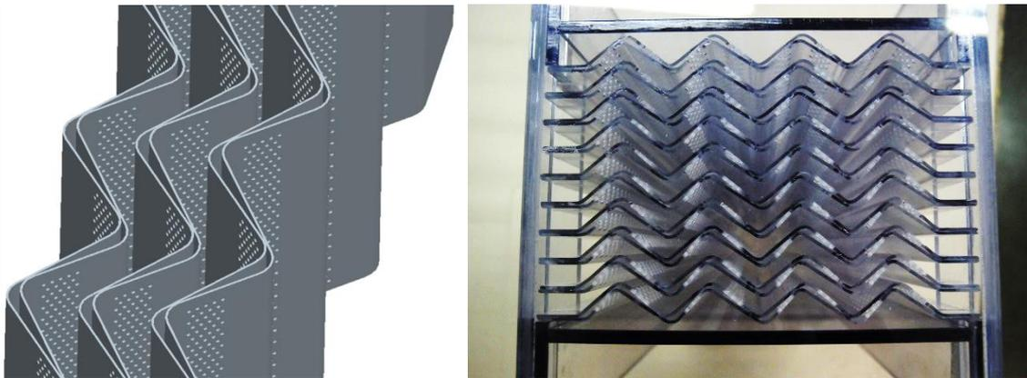
Fig. 6.10 Schematic view of the optimized vane separator design (left)<sup>136</sup> and the test module (right)
