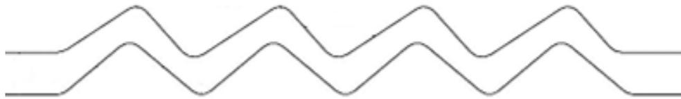
Fig. 6.3 Variable channel width of novel vane separator geometry
