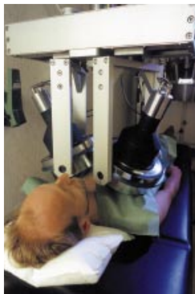
Fig. 1: Partial-body counter with two NaI(Tl)/CsI(Tl) phoswich detectors for measurements of photon emissions in the energy range between 15 and 100 keV in the lung.
