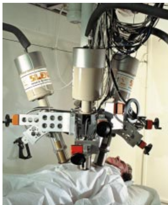
Fig. 2: Partial-body counter with four HPGe sandwich detectors for measurements of photon emissions in the energy range of 15 to 200 keV in the lung.
