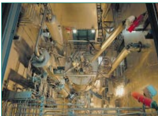
Fig. 8: View of a melter cell with remote handling capability of the non-radioactive prototype vitrification facility (PVA) of INE.
