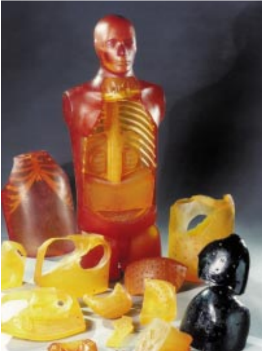
Fig. 3: Physical phantom for calibration of whole-body and partial-body counters for nuclide depositions in major organs and tissue structures of the body.
