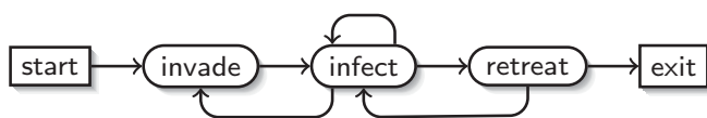
Figure 3.1.: State chart of an invasive program [104]. The phases invade , infect and retreat can be entered recursively or iteratively to adapt the degree of parallelism of the invasive program.
