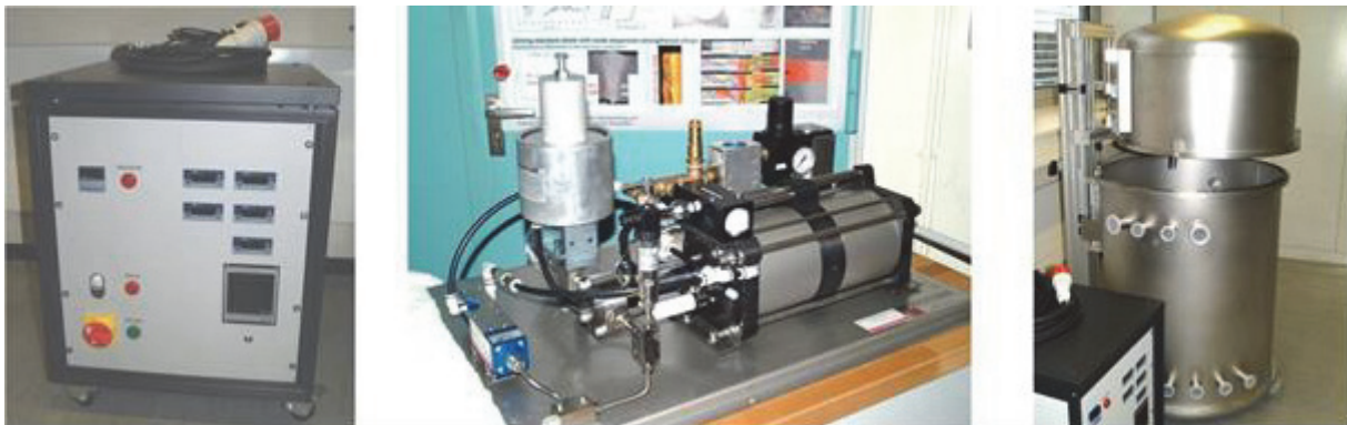
Fig. 5: Setup of a burst test / HRP device. The performance planned is 900 bar and 1100 °C, Ar gas.
