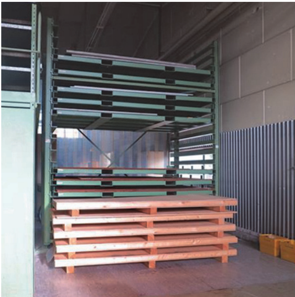
Fig. 3: New KIT heavy duty rack system for maximum plate dimensions of 4m x 2m.
