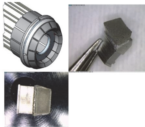
Fig. 11b: Design drawing of the segmented emitter (top left), manufactured segment (top middle and bottom right).
