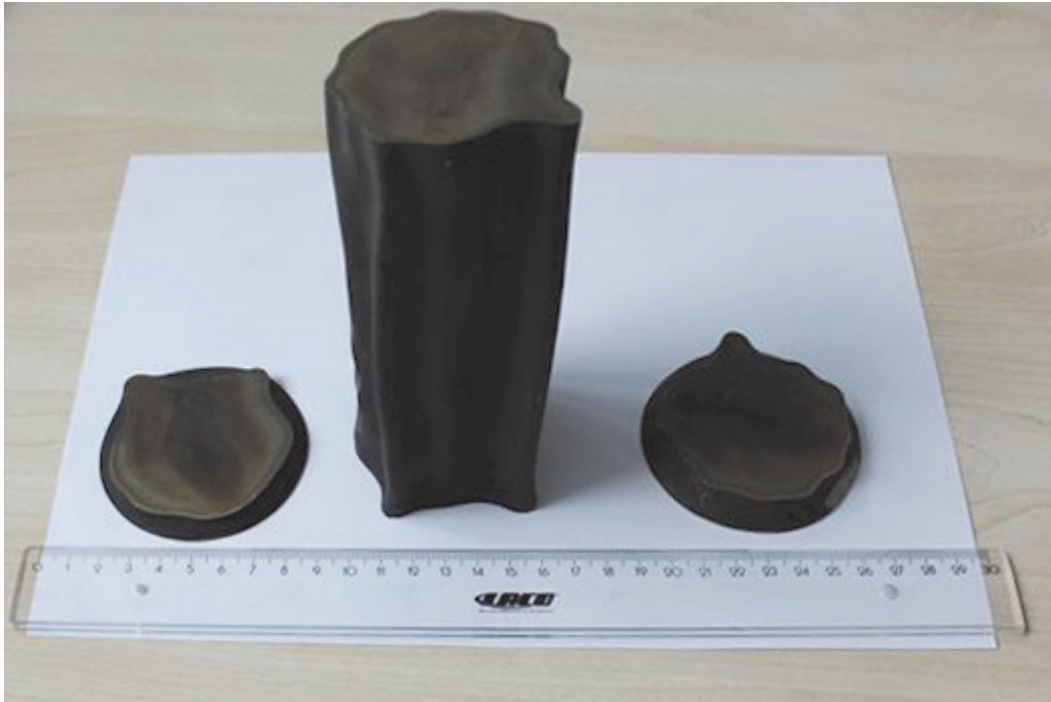
Fig. 8: Capsule after HIP (both ends removed by EDM).
