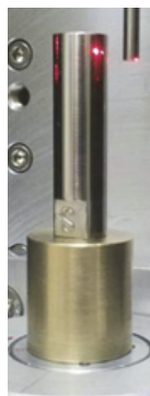
Fig. 4: Corrosion attack of an EUROFER sample in axial direction measured by laser scanning method as indicated in the picture in the left.
