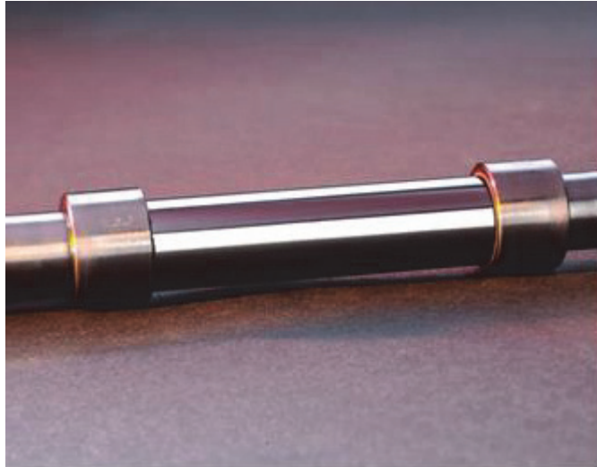
Fig. 6: W laminate pipe tested at PSA. The laminate pipe is coated with a black surface (H. Leiste, KIT, IAM-AWP) for a high absorption and low reflection of the sun light. On both ends the laminate pipe is joined to steel pipes made of austenitic steel. The HHF tests at the PSA were performed with water as cooling media. The W laminate pipe has a diameter of 15 mm and a wall thickness of 1 mm.
