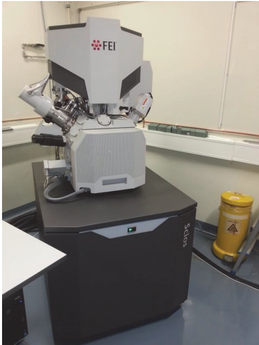
Fig. 2: FEI „SCIOS“: brand new dual beam microscope type.
