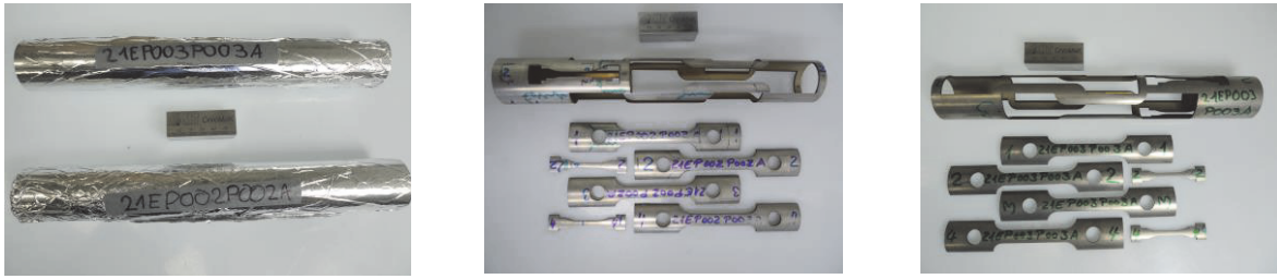
Fig. 1: On the left jacket sections after 2.5% stretching at room temperature and sectioned returned from CRPP after heat treatment (in the middle the specimen of 21EP002P002A after cutting, on the right specimen taken from 21EP003P003A).
