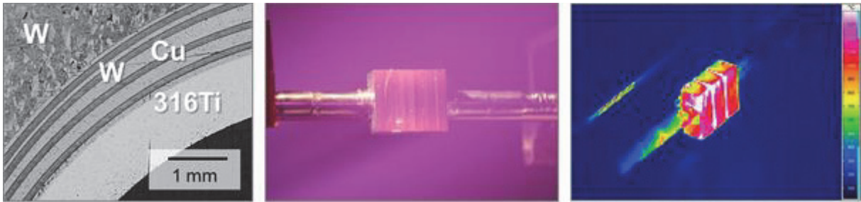
Fig. 2: For water in the PWR condition an austenitic steel pipe is used as a corrosion protection layer for the W laminate pipe. Successful tests were performed at the IPP in Garching (GLADIS, H. Greuner). Next steps might be to decrease the thickness of the steel pipe from 1 mm to 0.1 mm.
