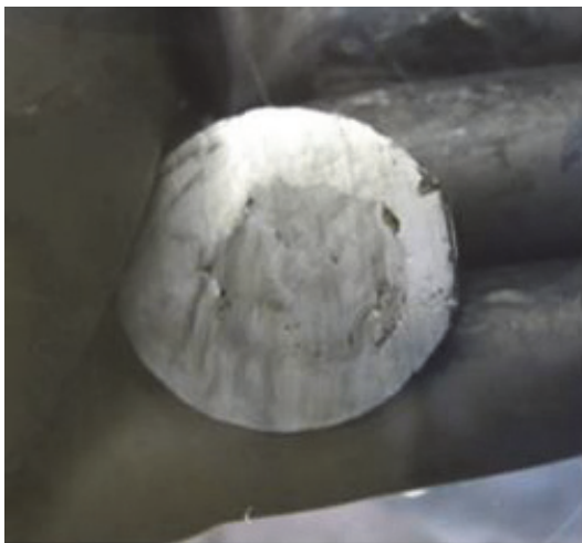
Hot-extruded Be-Ti rod inside of a steel jacket.
