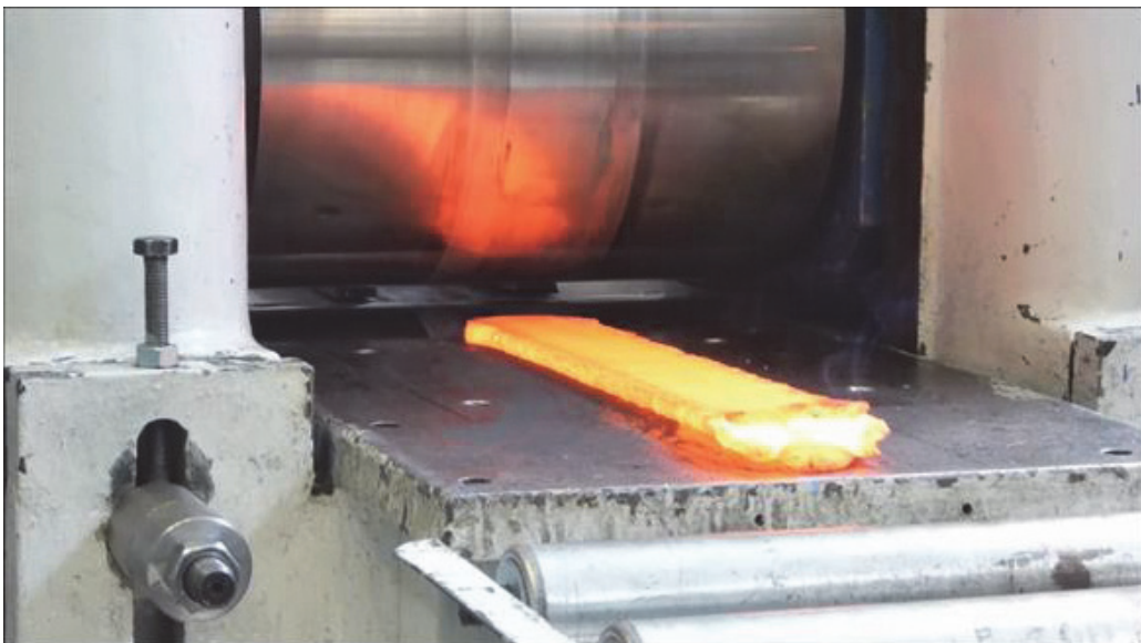
Fig. 9: Capsule after hot rolling.
