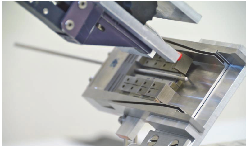
Mounting of SSTD specimens into the assembly tray of an IFMIF capsule using a vacuum gripper operated by a standard manipulator in a hot cell simulator.
