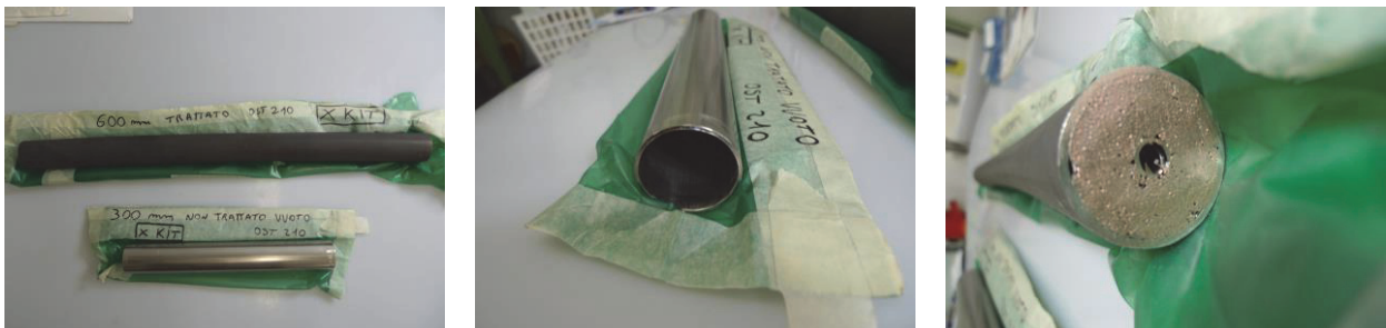
Fig. 3: Jacket material received from ASG (only compacted and heat treated conductor section).
