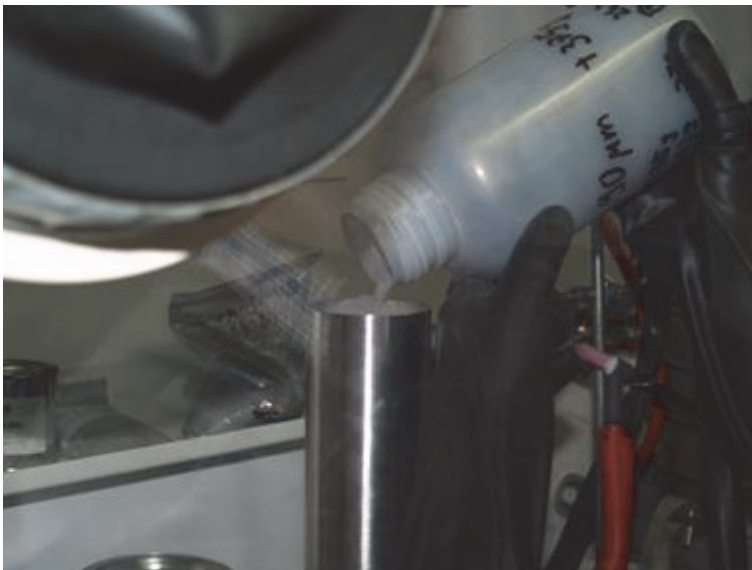
Fig. 5: Filling of the capsules inside an Argon-filled glove box.
