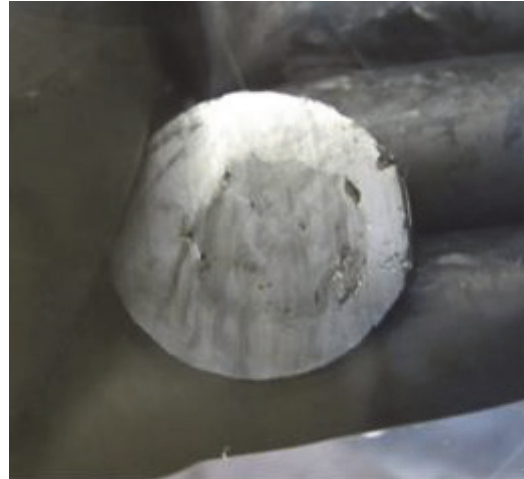
Fig. 1: Hot-extruded Be-Ti rod inside of a steel jacket.
