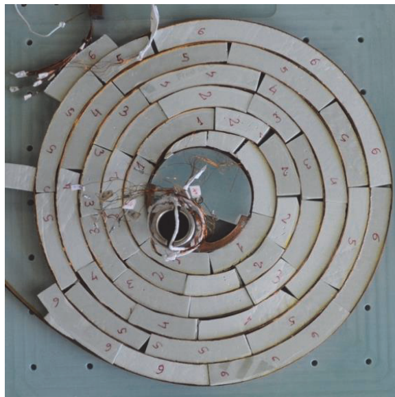
Fig. 3: Pancake coil of Roebel cable with spacings between turns.
