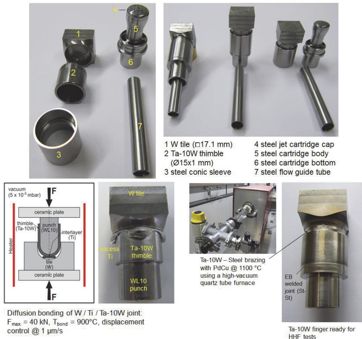
Fig. 1: Design and fabrication of square finger mock-ups: Individual component parts machined (top); diffusion bonding of W tile and Ta-10W thimble with Ti interlayer (bottom left); brazing Ta-10W thimble with steel transition tube with PdCu filler (bottom right).
