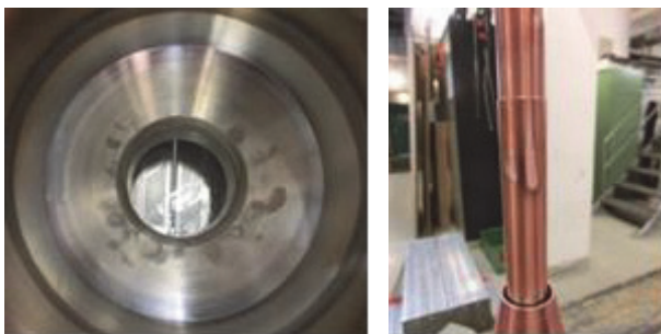
Fig. 2: Surface damages observed on of the anode (left) and coaxial insert (right) created due to the activity of trapped electrons.
