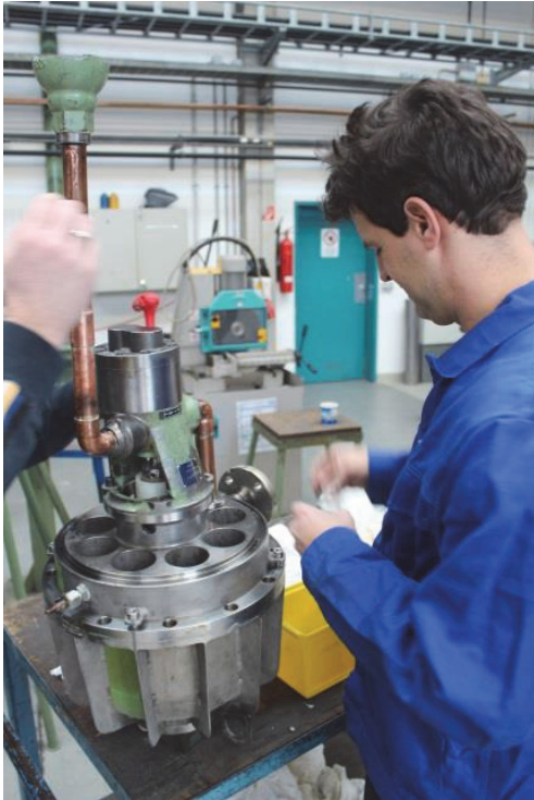
Fig. 3: Remedial maintenance work at components of the 300 W He-refrigerator.
