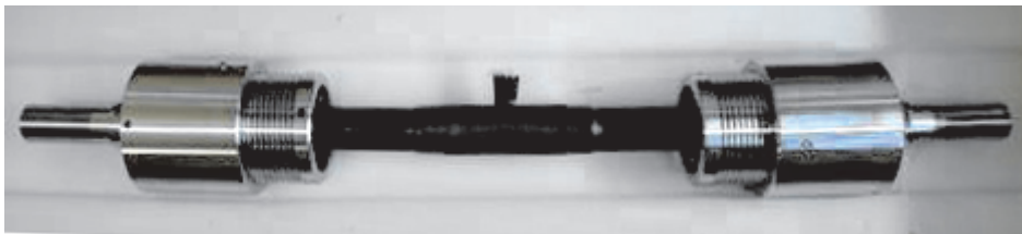
Japanese He-inlet prototype sample with fixture on both ends for machine installation.
