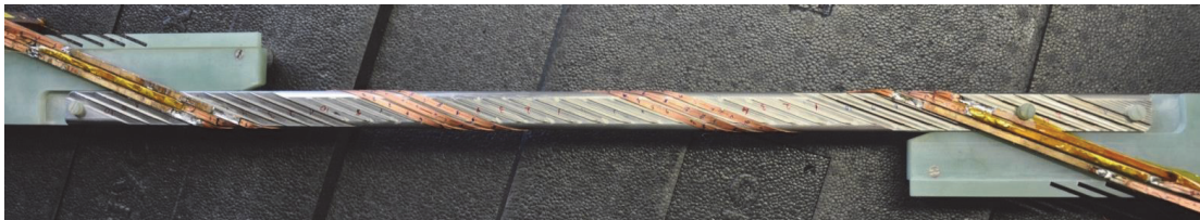
Fig. 5: Flat Rutherford cable (CCRC) with 3 Roebel strands of 4 mm width.
