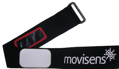
Abbildung 4.3: ekgMove-Sensor (movisens GmbH, 2014)
