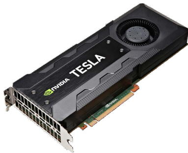
(a) Picture of the Nvidia Tesla K40 PCI express extension card [80].
