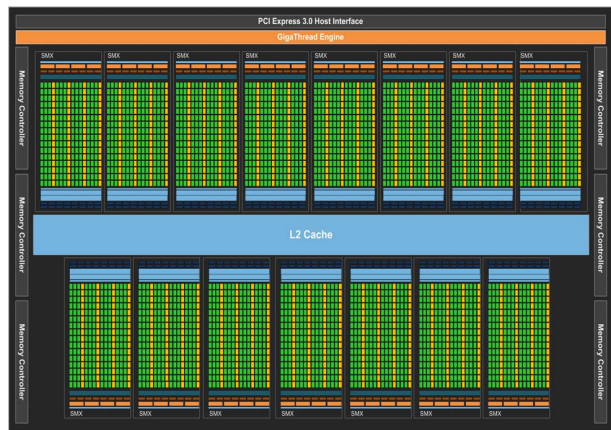
(b) GK110 full chip block diagram [79].
