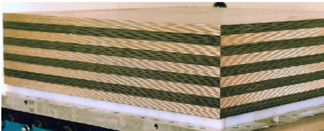
Figure 2.15: ECAL active volume (*pancake*). 9 superlayers are piled-up for a total of 50,000 1 mm  $\varnothing$  scintillating fibers running in opposite directions. The total  $68.5 \times 68.5 \times 16.7$  cm<sup>3</sup> pancake volume consists of a lead-fiber-glue volume ratio of 1:0.57:0.15, for an average density of  $\sim 6.8$  g/cm<sup>3</sup> [202].
