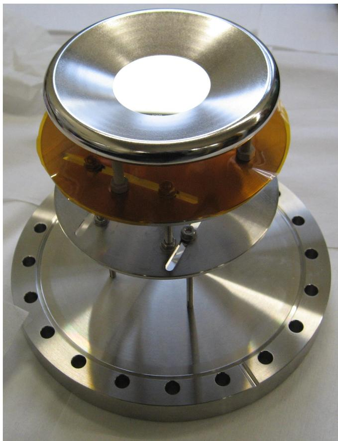
**Figure 5.16.: Picture of the pierce electrode installed on a flange** - The picture shows the special shape of the pierce electrode as well as an inserted and electrically contacted gold sample. The orange-brown sheet is a KAPTON-foil in order to protect the lower grounded parts of the construction from the high voltage cathode.
