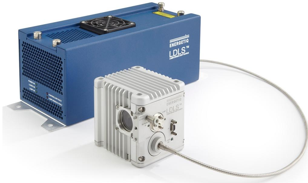
**Figure 4.7.:** Picture of the EQ-99X - the laser driven light source (LDLS) consists of the plasma enabling laser and the lamp itself with a proprietary xenon light bulb. The high intensity UV light is transmitted through the large window. [84]
