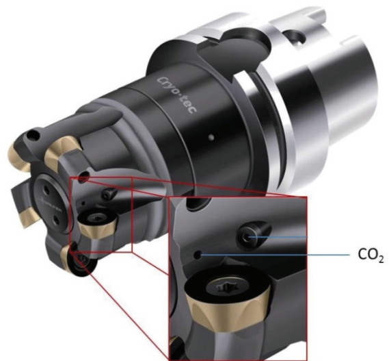
Figure 6: CO 2 Cooling Technology (Walter, 2013)
