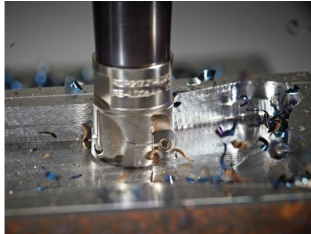
Figure 7: Dry Machining (Machinery Market, 2013)
