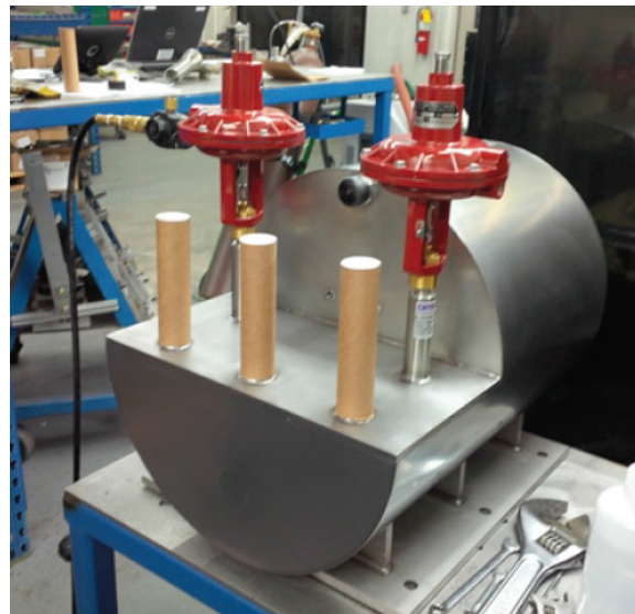
Figure 3: Sub-Cooler (5ME, 2014i, p. 35)
