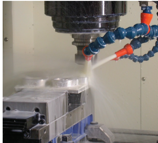
Figure 4: Conventional Flood Cooling (McKechnie)
