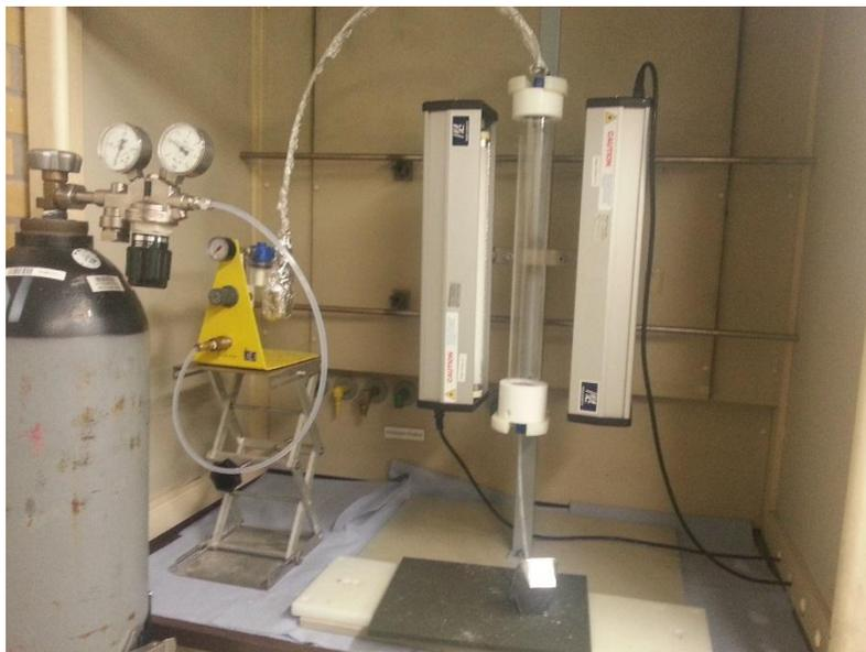
Figure 12 Photoreactor equipped with UV fluorescent tubes
