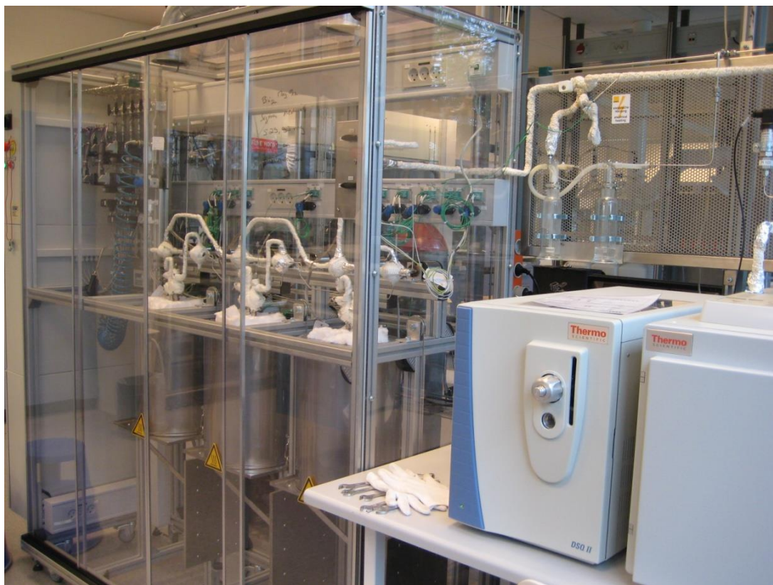
Figure 2.3: Photograph of the activity test set-up for selective oxidation reactions at DTU, Department of Chemical and Biochemical Engineering. On the left the mass flow controllers can be seen and on the right is the GC-MS. On the picture all ovens are lifted up and the reactors are covered.
