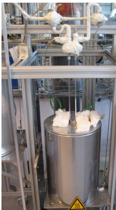
Figure 2.4: Photograph of the quartz reactor loaded with a catalyst connected to the test set-up.
