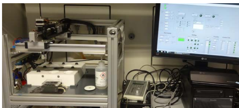
Figure 1.6: (top) A schematic diagram for the step-by-step growth of MOFs on SAMs using robot-dipping method: : (1) Metal solution, (2) pure ethanol, (3) pure ethanol, (4) ultrasonic bath, (5) linker solution, (6) substrate, (7) supporter, (8) substrate holder, (9) PC controller, (10) control electronic line, (11) dipping sequence. (bottom) The setup of robot dipping technique.
