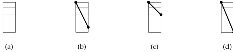
Figure 4.9: (a) A meta cell with its three minor cells for d = 4 ; (b) input embedding of a vertical switch; (c)+(d) the two possible output embeddings of the vertical switch.
