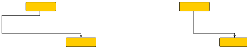
Figure 5.5: An edge that is a bow (left) and the edge after bow reduction (right).
