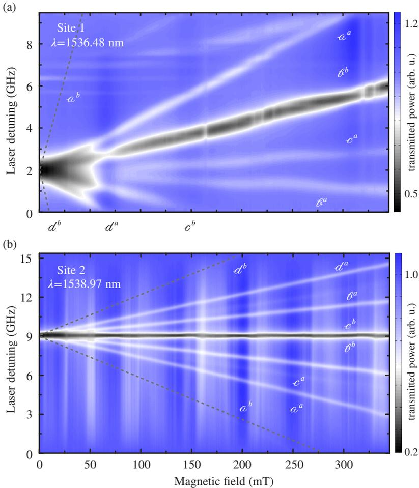
**Figure 7.2:** Optical transmission power spectrum vs. magnetic field of (a) site 1 and (b) site 2. The spectra were recorded at  $\approx 10 \mu\text{W}$  laser power.
