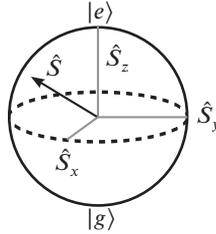
**Figure 2.3:** Bloch sphere. The kets  $|e\rangle$  and  $|g\rangle$  denote the excited and ground state of the spin, respectively.
