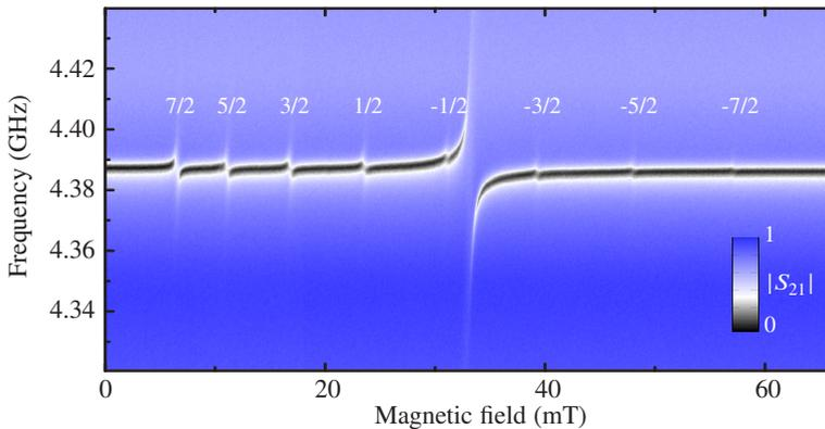
**Figure 5.12:** On-chip ESR spectrum of Er:YALO coupled to LE resonator #1. The numbers give the nuclear spin numbers for the eight hyperfine transitions.
