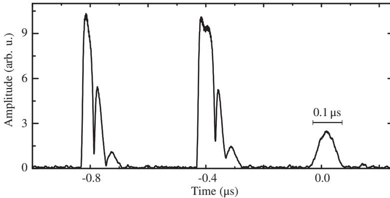
**Figure 6.9:** Spin echo sequence with a pulse separation of  $\tau = 400$  ns. Each pulse is accompanied by vacuum Rabi oscillations. The  $\pi/2$ -pulse has a width of 20 ns, but the echo appears as a 100 ns wide pulse of approximately Gaussian shape.
