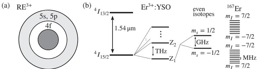
**Figure 2.1:** (a) Schematic structure of a tripositive rare earth ion: The 4f shell is shielded by the closed 5s and 5p shells. (b) Level structure of  $\text{Er}^{3+}$  doped into  $\text{Y}_2\text{SiO}_5$ .
