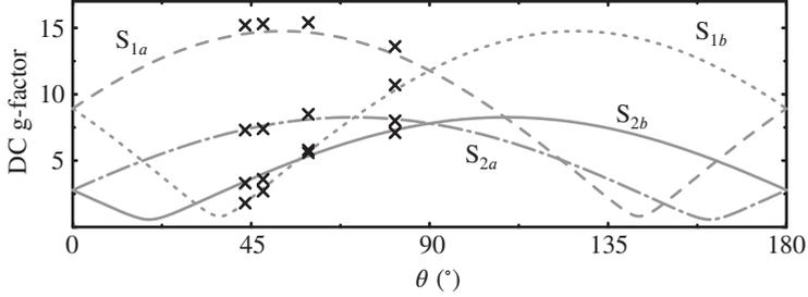
**Figure 5.4:** Simulation of the DC g-factors of sample Er:YSO1 as a function of  $\theta$  for fixed  $\phi = 111^\circ$ . The black crosses indicate the measured DC g-factors.
