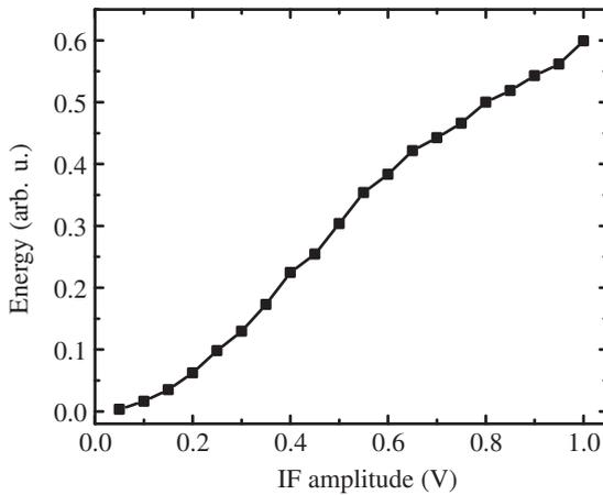
**Figure 1:** IF amplitude vs. relative pulse energy.
