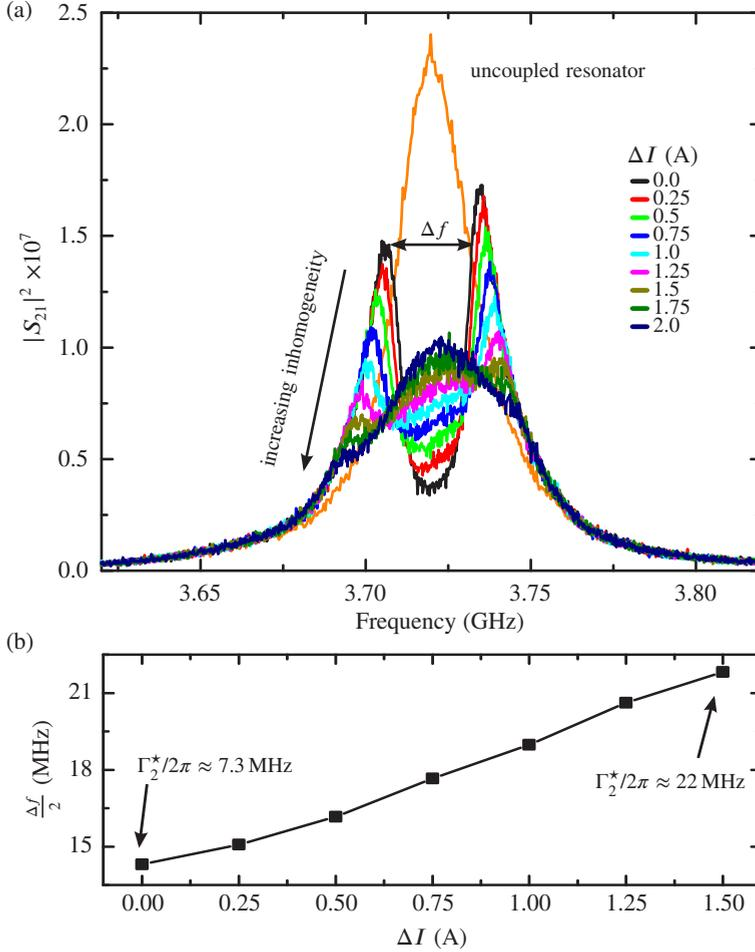
**Figure 6.5:** (a) Power spectra of the Cu resonator coupled to the spin ensemble. The colors indicate spectra with different magnetic field inhomogeneity introduced by the Helmholtz coil pair. For comparison, the orange line presents the spectrum of the uncoupled resonator. (b) Half mode splitting vs. electrical current inhomogeneity  $\Delta I = (I_1 - I_2)$  in the Helmholtz coil pair.
