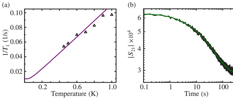
**Figure 6.4:** (a) Temperature dependence of the spin-lattice relaxation time. The purple line is a fit assuming a direct relaxation process. (b)  $|S_{21}|$  decay curve after a saturation pulse, plotted in double-logarithmic scale. The decay strongly deviates from a simple exponential decay curve. The green line is a fit employing a sum of three exponential decays. After 100 s,  $\approx 90\%$  of the spins are relaxed back to equilibrium.
