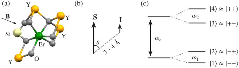
**Figure 2.5:** (a) Crystal structure of Er:YSO at site 2. (b) Dipole-dipole interaction between an electronic  $\mathbf{S}$  and nuclear  $\mathbf{I}$  spin. (c) Resulting level structure: The electronic levels split by the two super-hyperfine frequencies  $\omega_1$  and  $\omega_2$ .
