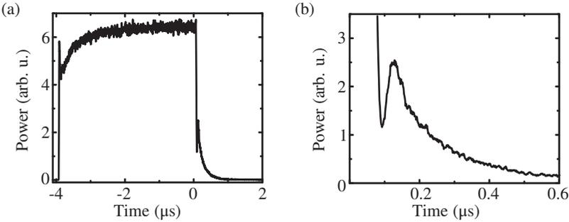
**Figure 6.7:** (a) Transmitted resonant microwave power vs. time. The beginning and end of the pulse shows a characteristic oscillation. (b) Zoom onto the oscillation at the end of the pulse.
