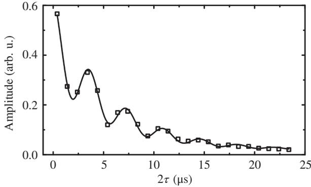
**Figure 6.10:** The exponential echo decay is modulated by prominent oscillations. The solid line presents a fit to the data with a  $T_2$  time of 5.6  $\mu\text{s}$ .
