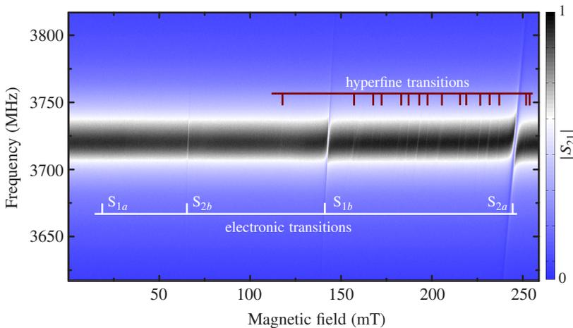
**Figure 6.2:**  $|S_{21}|$  transmission vs. frequency and magnetic field. Four sub-ensembles and a number of hyperfine transitions are visible. The  $S_{2a}$  transition shows a clear avoided level crossing.
