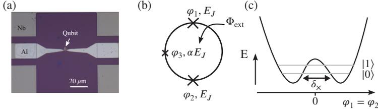
**Figure 3.1:** (a) Micrograph of a flux qubit (small circular structure) embedded in a coplanar microwave resonator (central line). (b) Schematics of a three junction flux qubit. (c) Effective potential of the flux qubit with its two computational states (gray lines).
