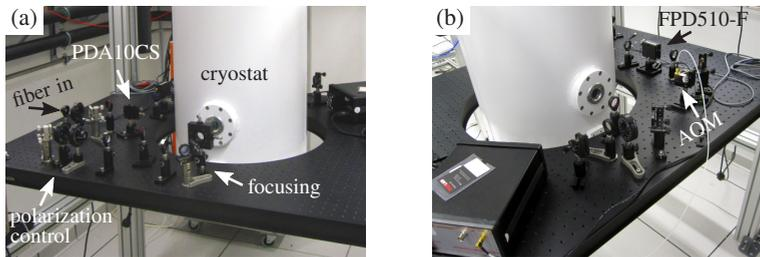
**Figure 4.5:** Second small optical table at the cryostat. (a) The laser beam is coupled out of the fiber, linearly polarized, widened to approximately 1 cm diameter and finally focused into the fridge. In the background, the Thorlabs PDA10CS photodetector is seen. (b) Optical output of the cryostat. The beam is focused on the AOM switching it between two photo detectors.
