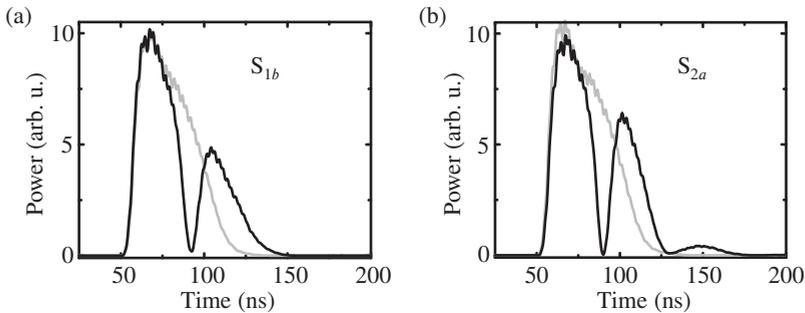
**Figure 6.8:** Response to a 20 ns MW pulse. The grey line shows an off resonant pulse for comparison. (a)  $S_{1b}$  transition (143.0 mT). (b)  $S_{2a}$  transition (245.8 mT).
