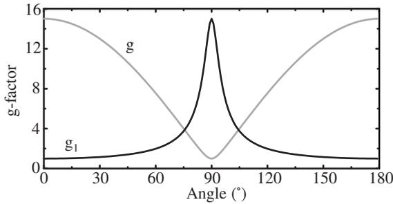
**Figure 2.2:** Angular dependence of DC and AC g-factors in axial geometry,  $g_{\perp} = 1$ ,  $g_{\parallel} = 15$ .
