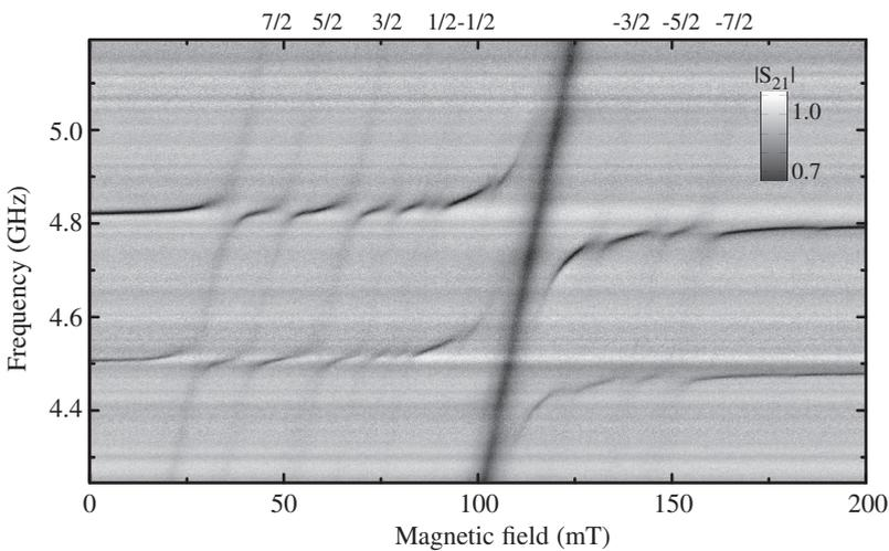
**Figure 5.13:** Avoided level crossings between the two LE resonators and the Nd spin ensemble. The coupling to the hyperfine transition is clearly visible.
