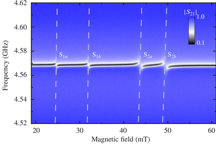
**Figure 5.2:** On-chip ESR spectrum of sample Er:YSO1 coupled to a LE resonator. The orientation of the crystal's b-axis with respect to the DC magnetic field is  $\theta = 81.3^\circ$ .
