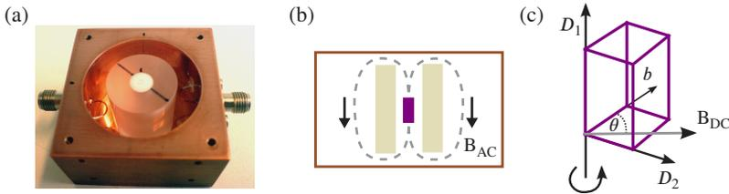
**Figure 5.18:** (a) Three dimensional sapphire loaded copper cavity. The loops on the left and right serve as coupling coils. (b) Coupling geometry: The dashed line represents the AC magnetic field of the  $\text{TE}_{011}$  mode, which is very homogeneous at the location of the Er:YSO crystal (purple). (c) Orientation of the crystal axes.
