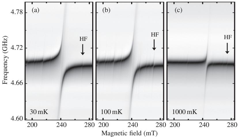
**Figure 5.9:** Avoided level crossing at different temperatures. Remarkably, the hyperfine transitions are more pronounced at 100 mK, and the system is still strongly coupled at 1 K,.
