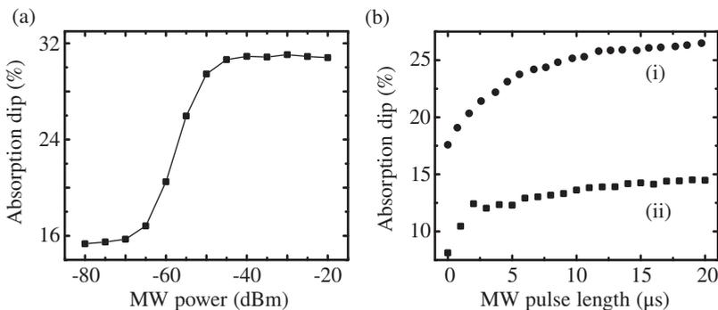
**Figure 7.4:** (a) MW power dependence of the optical  $e^a$  absorption dip. (b) Optical absorption signal of the  $e^a$  transition vs. MW pulse length. The power of the pulse is approximately 10 dBm at the crystal. Curve (i) was recorded using optical pumping to reset the system whereas curve (ii) was measured by waiting 100 s after each point to allow the spin ensemble to thermalize to the ground state (see text for details).
