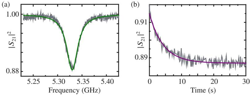
**Figure 5.8:** (a) Transmission line absorption dip revealing the  $S_{2a}$  transition at a magnetic field of 273.2 mT. The green line displays a Lorentzian fit to the spectrum. (b) Reappearance of the absorption signal after a strong saturation pulse. The solid line is an exponential fit to the data.
