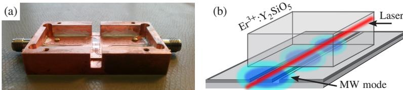
**Figure 7.1:** (a) Sample holder with microwave connectors on the left and right and slits in the front and back for the laser. In the middle, the Er:YSO crystal is seen. (b) Schematics of the hybrid system shown the coupling geometry where the optical beam (red) overlaps with the magnetic mode of the CPW resonator (blue).
