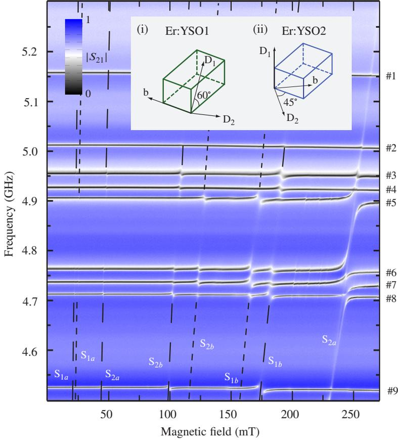
**Figure 5.6:** On-chip ESR amplitude spectrum of samples Er:YSO1 (inset (i)) and Er:YSO2 (inset (ii)) coupled to an array of nine SC LE resonators. The four electronic transitions of Er:YSO1 are indicated by dashed lines whereas the dotted lines denote the transitions of Er:YSO2.
