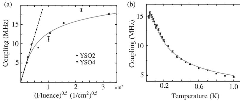
**Figure 5.17:** (a) Collective coupling vs. the square root of the fluence. The dashed straight line shows the expectation for a 100% effective implantation. The gray line is a fit to an empirical theory, see text for details. (b) Temperature dependence of the collective coupling strength of sample YSO4 area #3. The temperature dependence follows the expectation for a paramagnetic crystal (gray line).
