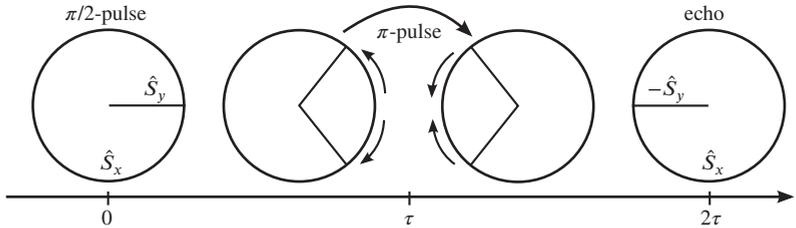
**Figure 2.4:** From left to right, spin dynamics of the two pulse sequence in the equatorial plane of the Bloch sphere. After the initial  $\pi/2$ -pulse, the spins defocus. At  $t = \tau$ , the  $\pi$ -pulse flips the phase of the  $y$ -component leading to a rephasing and an echo at  $t = 2\tau$ .
