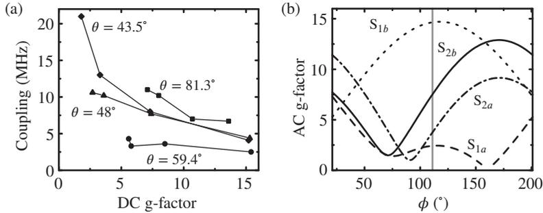
**Figure 5.5:** Anisotropic coupling. (a) Coupling vs. DC g-factor. For almost all samples, the coupling scales inversely to the DC g-factor. (b) Simulated angular dependence of the AC g-factor for  $\theta = 44^\circ$ . The grey line denotes the mean orientation. The coupling measured with on-chip ESR represents an average value with respect to the AC g-factor anisotropy due to the inhomogeneous AC field of the LE resonator.
