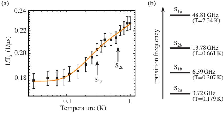
**Figure 6.13:** (a)  $1/T_2$  vs. temperature. Note the logarithmic scale. Between 30 mK and 1 K, the  $T_2$  time decreases from approximately  $5.6 \mu\text{s}$  to  $4.4 \mu\text{s}$ . The solid line is a fit to theory considering decoherence induced by thermal fluctuations from the surrounding sub-ensembles. (b) Transition frequencies and effective temperatures at 246 mT of all sub-ensembles.
