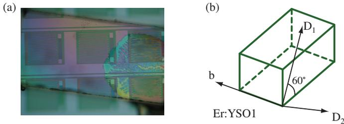
**Figure 5.1:** (a) Er:YSO crystal on top of an array of LE resonators. (b) Orientation of the axes of the crystal.
