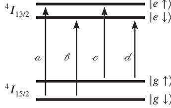
**Figure 2.6:** Optical transitions for an erbium site and magnetic class. In a magnetic field, the degeneracy of the spin states in the optical ground and excited state is lifted thereby giving rise to four optical transitions.
