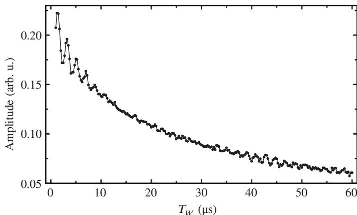
**Figure 6.11:** Stimulated echo decay. The beating between the two hyperfine frequencies is clearly visible. The data can be fit with a double exponential decay with decay times of 2 and 23.9  $\mu\text{s}$ .
