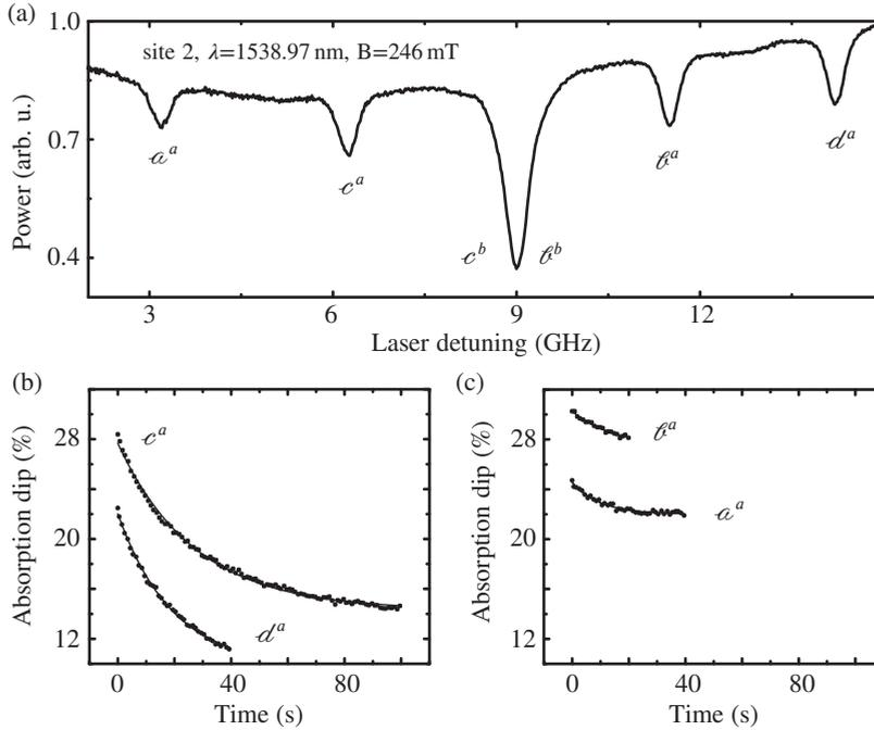
**Figure 7.5:** (a) Optical transmission at 246 mT. (b) Time evolution of the absorption dips of transitions  $e^a$  and  $d^a$  after a strong microwave pulse on the  $|g \downarrow\rangle$  to  $|g \uparrow\rangle$  transition of site 2a (site  $2^a$ ). (c) Corresponding time evolution of the absorption dips of the  $e^a$  and  $l^a$  transitions.
