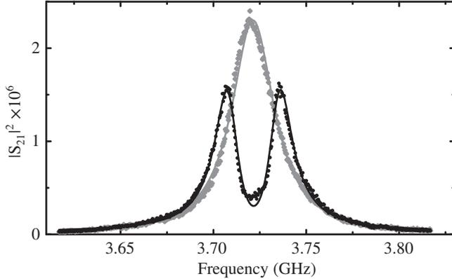
**Figure 6.3:** Avoided level crossing of the resonance at 246 mT (black points). The solid black line represents a fit to the data. For comparison, the resonator at 227.7 mT is displayed (gray dots).
