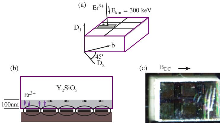
**Figure 5.15:** (a) Sketch of the implantation process. A focused  $\text{Er}^{3+}$  ion beam irradiates several areas of an undoped  $\text{Y}_2\text{SiO}_5$  crystal. (b) Schematics of the coupling geometry. (c) Picture of the implanted YSO crystal on top of a superconducting chip with an array of nine LE resonators. Each implanted area fits to the size of one LE resonator.
