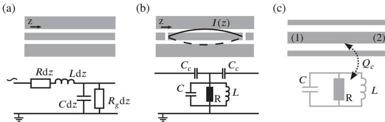
**Figure 3.2:** (a) Coplanar transmission line and corresponding equivalent circuit. (b) Transmission line resonator. The solid and dashed lines sketch the current distribution of the first harmonic. The lumped element circuit model of the resonator is shown below. (c) Lumped element resonator coupled to a transmission line (notch type configuration).
