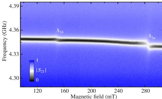
**Figure 5.16:** ESR transmission spectrum of the YSO4 crystal, area #3 coupled to one of the LE resonators. Two dispersive shifts of the resonator are visible in the spectrum due to the magnetic coupling to the electronic spin transitions  $S_{1b}$  and  $S_{2a}$  of the erbium ions
