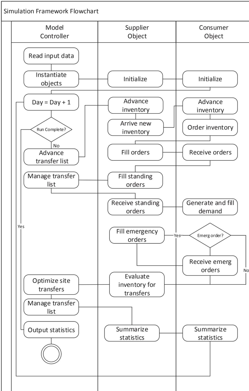
**Figure 1-** Flowchart describing processing simulation process flow
