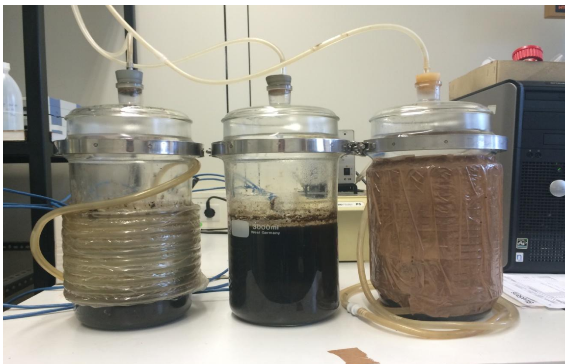
Figure 3.5 Batch assays for dry anaerobic digestion of biowaste with different moisture content.
