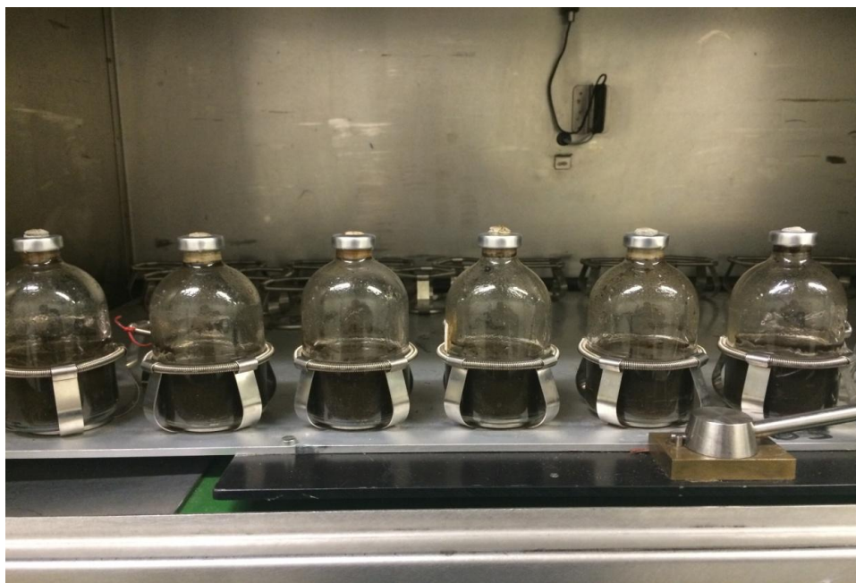
Figure 3.6 Batch assays for determination of VFA degradation to biogas
