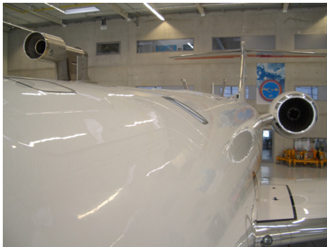
(c) Different trace gas inlets (TGI) and view-ports on top surface
