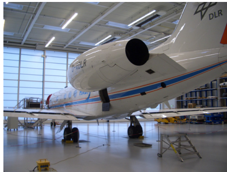
(d) Left engine; opening below: baggage compartment aperture
