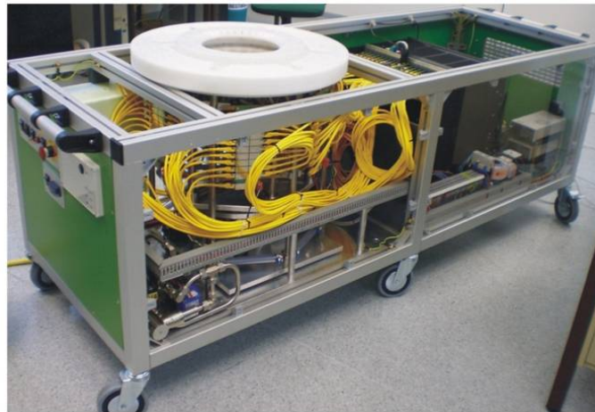
Figure 7.30.: The 3D USCT II system for ultrasound computer tomography [22]
