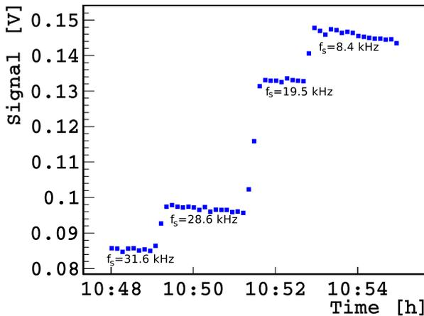
Figure 3: The microwave signal at the IR1 beamline of the ANKA storage ring taken during the low- $\alpha_c$  squeeze procedure. The level of the microwave signal corresponds to the bunch length. We have used preamplifier and Shottky diode setup for this measurement.
