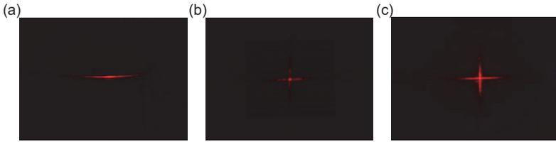
Figure 2.18: The emission patterns of Alq<sub>3</sub>:DCM DFB lasers pumped by a Nd:YVO<sub>4</sub> Laser (355 nm): (a) 1D-DFB laser. (b) 2D-square-array DFB laser pumped with pulse energy 2 times higher than the laser threshold. (c) 2D-square-array DFB laser pumped with pulse energy 5 times higher than the laser threshold.
