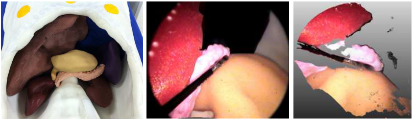
Figure 9.9.: OpenHELP torso phantom built from segmented CT images (left), endoscopic video frame featuring several silicone organs (middle) and corresponding 3D-reconstruction from stereo endoscopic data (right).
