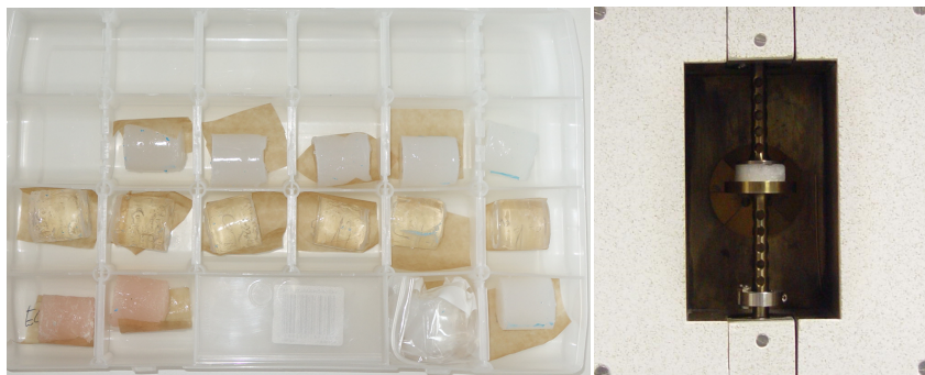
Figure 9.5.: A sample was manufactured from several silicone mixtures (left) which were subsequently analyzed using an Eplexor rheometer (right).
