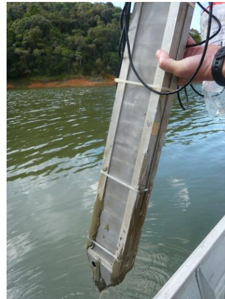
Figure 4-22: DPS after recovery with adherent sediment.
