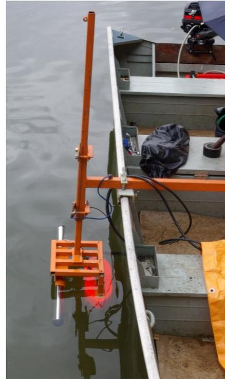
Figure 4-4: The mounted EA 400 echo sounder on the aluminum vessel.
