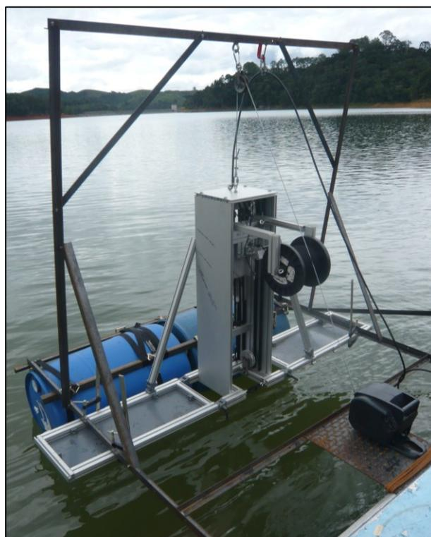
Figure 5-44: The DPS-PS positioned on the floating platform at the side of the vessel in combination with an electric winch.
