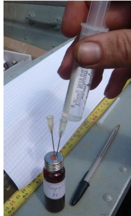
Figure 4-23: Injection of DPS solution in the head space vial.
