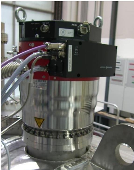
Abb. 9-8: Turbomolekularpumpe HiPace2400
