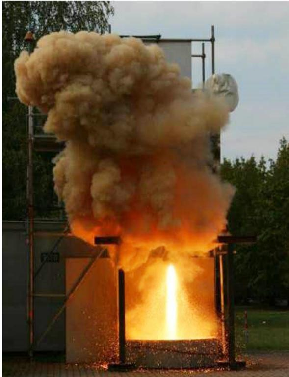
Fig. 6: DISCO jet experiment: a core melt jet is penetrating the reactor pressure vessel.
