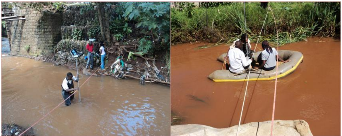
Figure 13: Flow measurement techniques using current meter at the Nairobi River (WRMA 2012)
